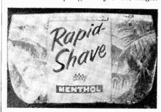
and linearity controls, we noticed that they were fully advanced. All other settings gave abnormal compression at the top and bottom of the raster. Finally we decided to replace the 6AH4, used
