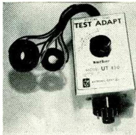
Test adapter for newer low-voltage-heater CRT's.
