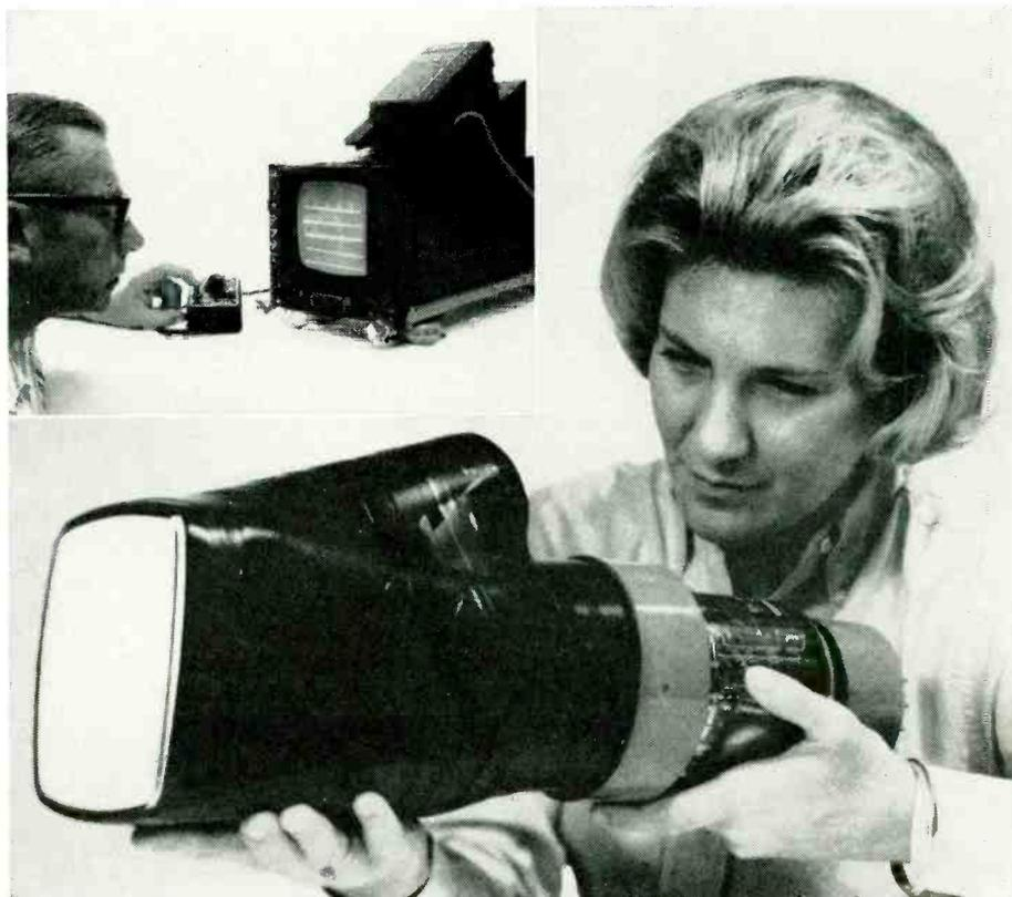
Barbara Britton of the US Army Electronics Research & Development Laboratory, Fort Monmouth, N. J., peers through the rear-view porthole of newly designed picture tube for Army applications. (Inset) Technician prepares to trigger the camera, mounted above and behind the tube, as he watches the display on the screen.
