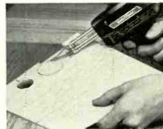
**Does more than soldering.** With cutting and smoothing tips you can cut plastic tile, repair plastic toys, seal plastic bags, repair furniture dents, etc.
