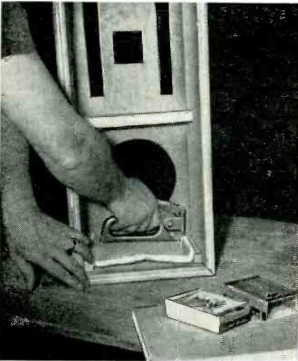
← Acoustic insulation goes on easily with a stapler or tacker. Rubber or household cement will do just as well. (Bottom photo) Speaker should go in only after all heavy assembly and sanding are done.
