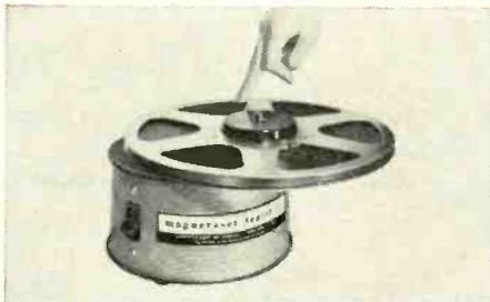
10½-in. reels without spindle shifting. Erases ¼ and ½-in. wide tapes as well as 16 and 35 mm magnetic sound film tracks. Automatic on-off rocker switch.—Amplifier Corp. of America, 398 Broadway, New York 13, N. Y.
