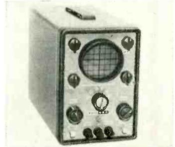
rms/cm; cathode follower input with fine attenuator in output. Sweep circuit: Recurrent sweeps 10 cycles—100 kc in 4 overlapping ranges, external or internal synchronization; synchronization is fully automatic on all ranges; full retrace blanking.—EICO Electronic Instrument Co., Inc., 33-00 Northern Blvd., Long Island City 1, N.Y. END
