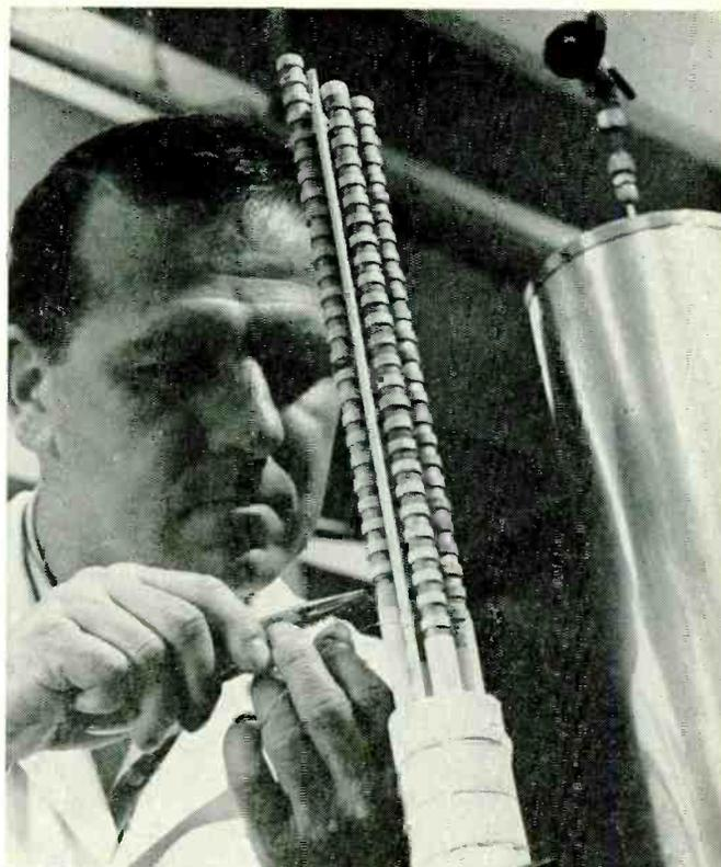
**EXPERIMENTAL FUEL-CELL SYSTEM** generates pure oxygen from two waste products of breathing—carbon dioxide and water. Normal cell uses oxygen in reaction with fuel—such as hydrogen—to generate electricity. Here, process is reversed: cell eats electricity, makes oxygen. Obvious application? Space-capsule oxygen generation. Westinghouse, developer of system, estimates four men could be supplied from equipment weighing 60 to 75 lb complete, occupying only 3 cu ft and taking about 1 kw power.
