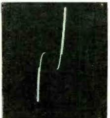
Tunnel diode with trace expanded
