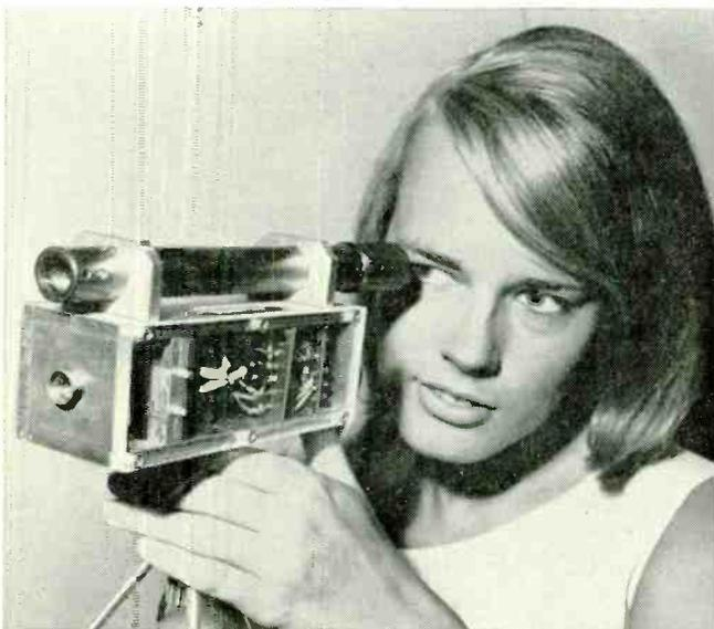
**LOOK ME IN THE LASER!** This is a public-demonstration model of a laser transmitter RCA will install on Gemini 7. Conversations by laser beam will be tried between Gemini 7 and ground stations. Heart of the actual (left) device is new room-temperature gallium arsenide laser diode. Four are used, located behind small lens openings. Large opening is for telescope used to aim transmitter at laser receiver beacon at White Sands Missile Range.
