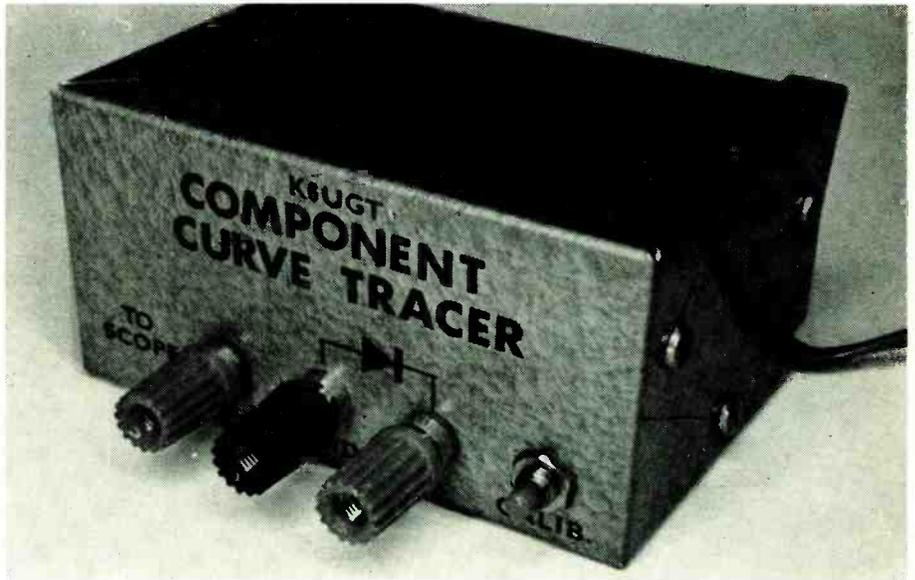
left open, and calibration switch S is closed, equal voltages will appear across J1-J2 and J2-J3, since R1 and R2 are equal in value, with "ground" at their junction.
