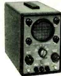
**New Model 440** Scope. Lowest-priced quality oscilloscope available. Excellent for electronics teaching and home workshop. Flat 2c-500kc. 3" flat-face new CRT. Compact, light, rugged. **\$49.95 kit, \$69.95 wired.**
