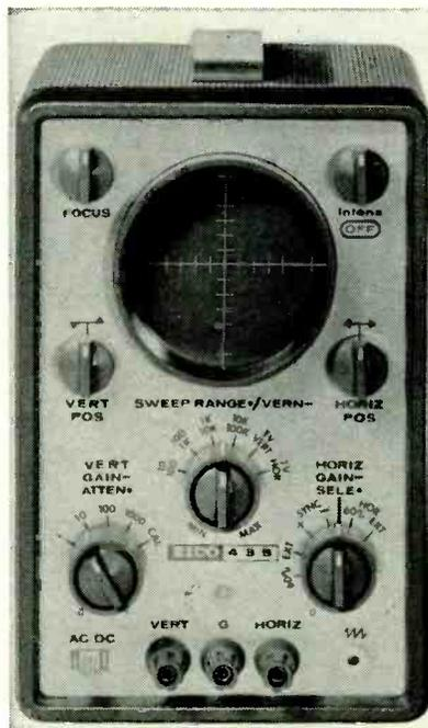
A built-in 200-mv p-p calibration voltage is provided; this is set by a Zener diode, and can be recalibrated by an internal adjustment if necessary.
