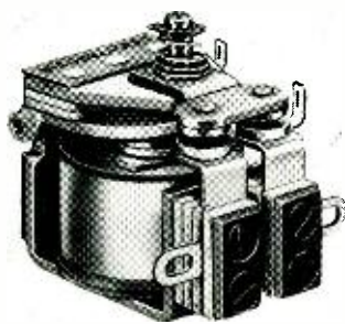
Fig. 3. Typical general-purpose clapper-style relay.
