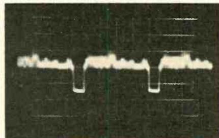
Fig. 13—Proper retrace blanking at CRT grid-cathode circuit. Total p-p amplitude is 8 volts, cutting off CRT beams.
