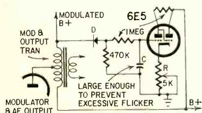
Fig. 7—Overmodulation indicator: The modulated B+ is rectified and fed to the grid of 6E5, varying the shadow angle.
