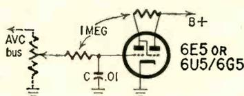
Fig. 2—Maximum avc voltage in AM receiver causes the smallest shadow angle.
