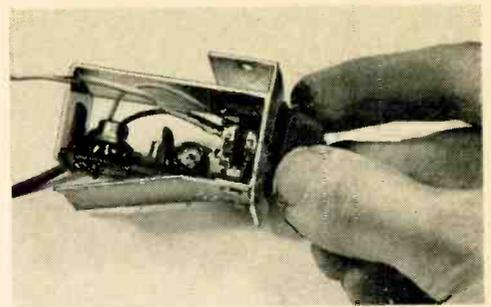
Now there's no need to reach for the windshield wiper knob every few seconds when driving through light mist or on slush-covered roads. You can set this Automatic Pause Controller to obtain any desired pause between sweeps, while the wiper still operates at normal speed.
