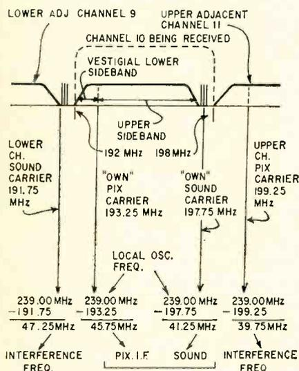
Fig. 1—Distribution of other signals in and around TV channel 10. The intermediate and interference frequencies are identical on all other television channels.
