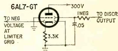
Fig. 4—6AL7 light bars are shortest when deflector 2 has zero voltage and deflector 3 has a maximum negative voltage.
