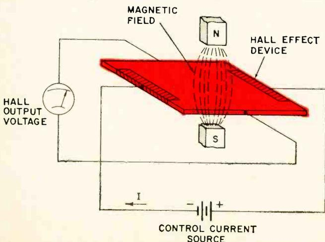
Fig. 2-a—Outside a magnetic field, charge carriers are uniformly distributed in the Hall element and voltage is zero.
