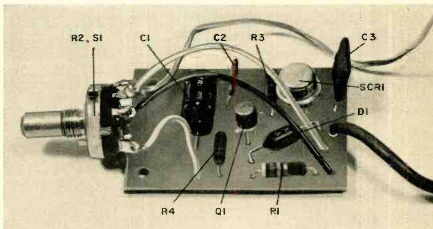
The APC can be built on a PC board or a perforated board for point-to-point wiring.
