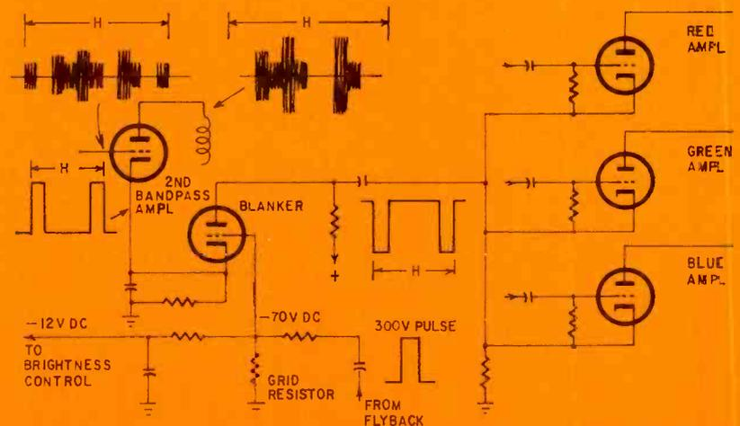
Fig. 2—Blanker tube is keyed on by flyback pulse during retrace, cutting off the second color i.f. amplifier and passing only the color video information.
