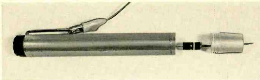
Use the solid-state "glow-lamp" oscillator as signal injector to test radios and amplifiers. The 47K series resistor in the hot output lead minimizes circuit loading.
