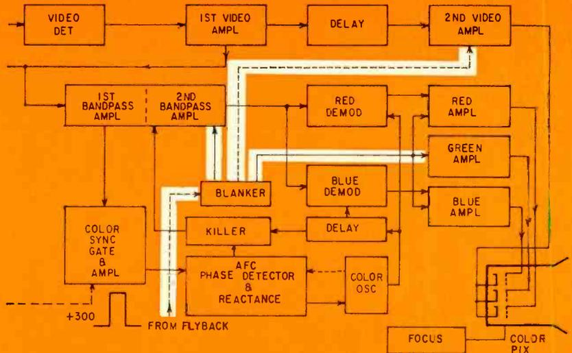
Fig. 1—Typical blanking circuit in today's color sets performs three functions.
