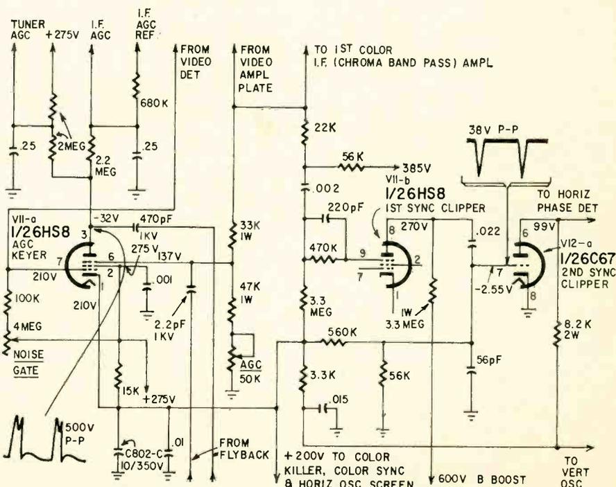
Fig. 2—Agc and sync circuits in the Motorola TS-908 color TV chassis. Unstable horizontal sweep and jittery color were caused by a defective filter capacitor (C802-c) which permitted the agc keying pulses to appear on the 200-volt line.
