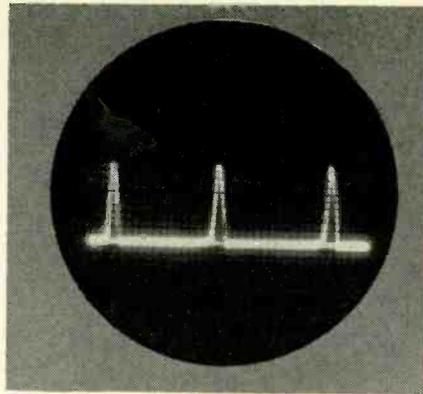
Fig. 3—The correct pulse on the first sync-clipper grid is 34 volts peak-to-peak.
