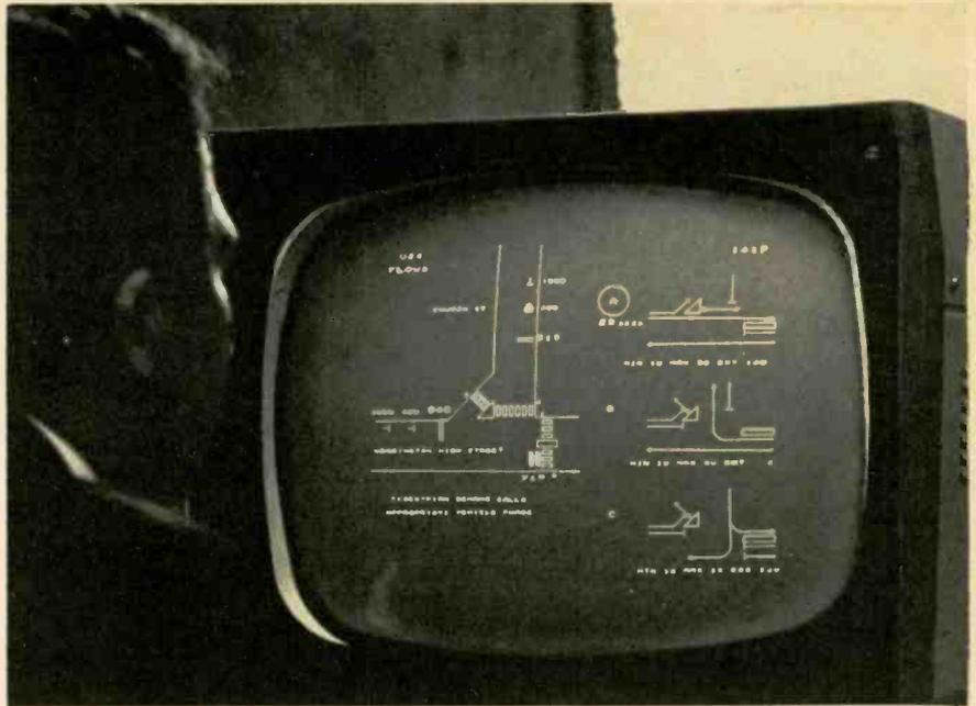
**Computer monitors London traffic**—Street names, traffic flow, pedestrian crossings and other information are shown on this computer-controlled display system to be installed in New Scotland Yard for experimental control of traffic. Marconi Company will build and install system.
