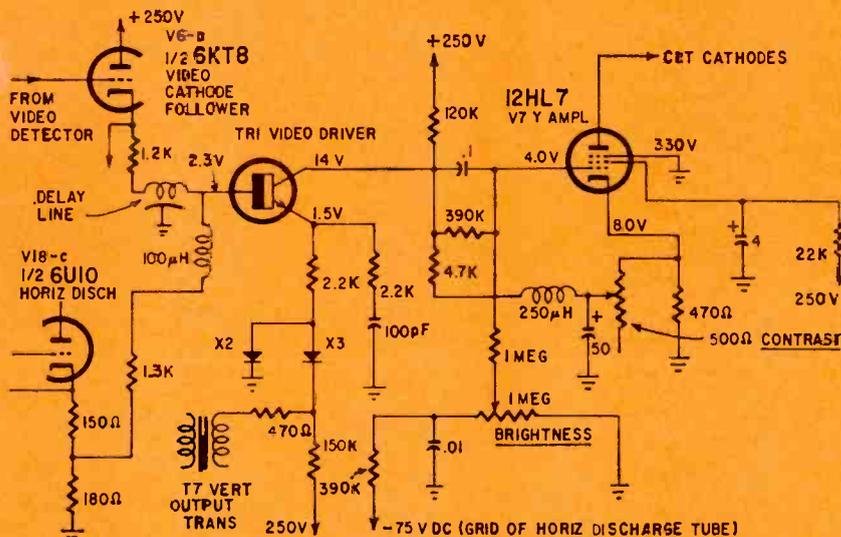
Fig. 7—All blanking in the Zenith 20X1C36 chassis is done in video driver stage.
