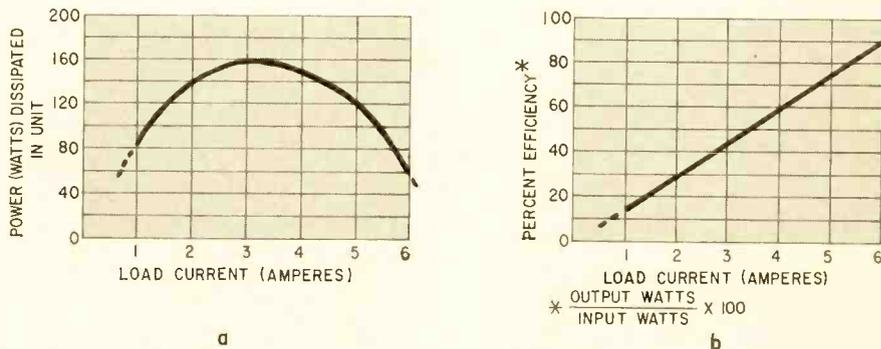
Fig. 2—Performance curves for a conventional series-regulated variable-voltage supply driving a 15-ohm load. Fig. 2-a shows dissipation. Fig. 2-b, efficiency.
