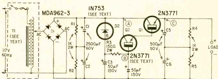
Fig. 1—High-efficiency dc supply for delivering up to 6 amps into 15-ohm load. C4, the 50- $\mu\text{F}$  electrolytic tied to Q2's base, is part of current-control network.
