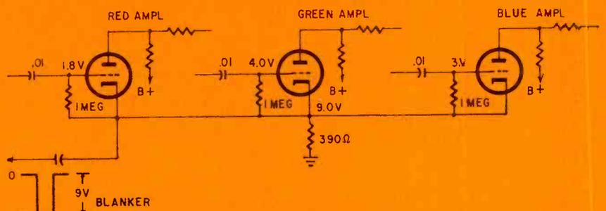
Fig. 3—Red, green, blue amplifier cathodes are clamped line-to-line by blanking pulse, preventing an undesirable shift of the color values due to RC coupling.
