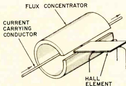
Fig. 7—Magnetic field around conductor (or ion beam, see "Some Commercial Applications") is concentrated on Hall device and the output is measured as current.
