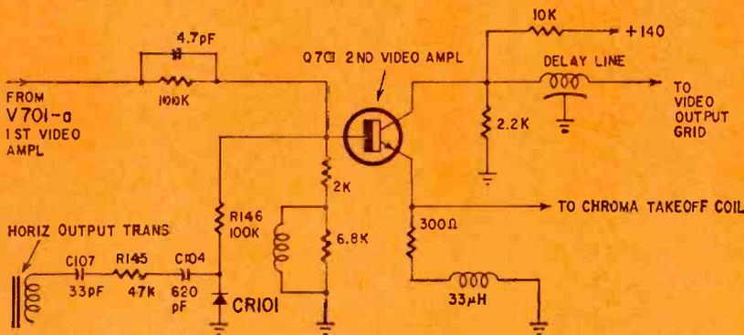
Fig. 6—Horizontal blanking in the G-E CB chassis at second video amp stage.
