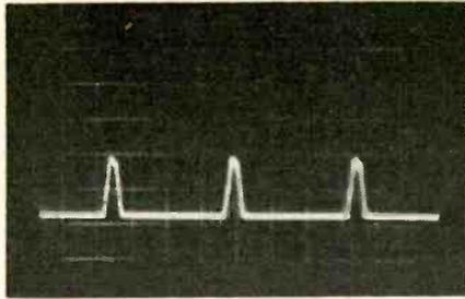
Fig. 9—Horizontal blanking pulse (4 volts p-p) taken from cathode circuit of horizontal discharge tube in Fig. 7.
