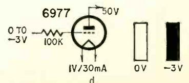
Fig. 1 (a-d)—"Magic eye" tubes provide a variety of these small signal display patterns. (1M3/DM70 is shown at c.)
