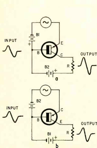
Fig. 3—An npn grounded-base transistor amplifier (a) has high power and voltage gains with slight current loss. Transposing emitter and collector and reversing bias polarities (b) results in considerable current loss, moderate voltage gain and possibly some power gain as well.
