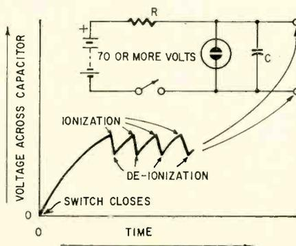
Fig. 1—Glow-lamp relaxation oscillator and output waveform. High voltage need makes lamp impractical for solid state.
