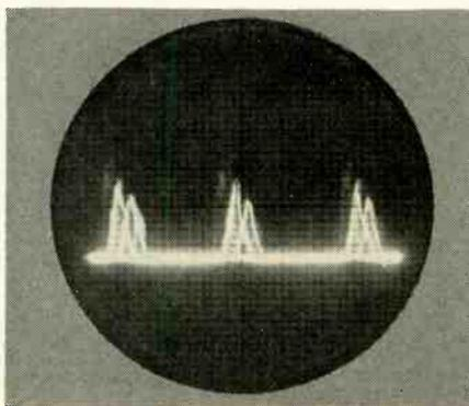
Fig. 1—This agc keying pulse strayed into the horizontal afc and color apc circuits, causing jittery sync and color.
