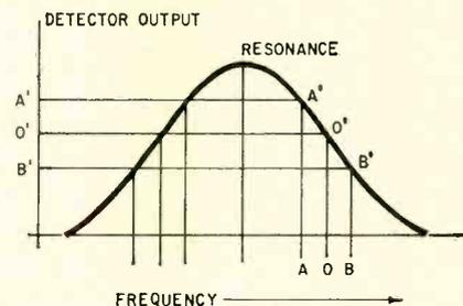
Fig. 10—In slope detection, carrier is tuned to point O. Capacitance changes may cause carrier shift to points A or B.
