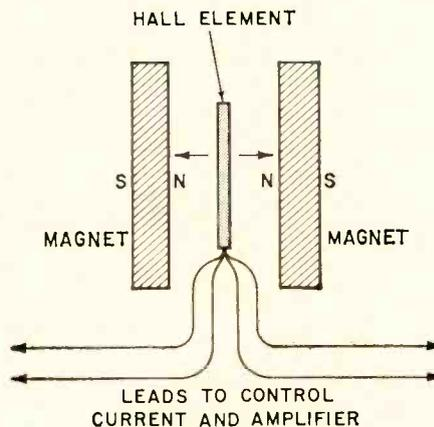
Fig. 6—Minute movements of Hall device or magnets can be detected and measured.
