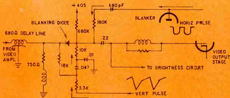
Fig. 4—Blanking circuit of the RCA CTC31 chassis. The diode is reverse-biased by blanking pulses, which cut off color video during the horizontal retrace period.
