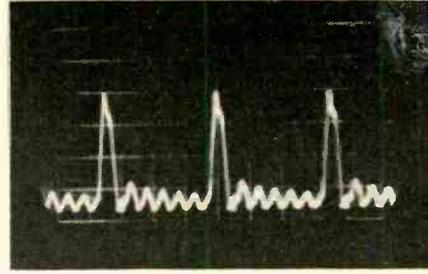
Fig. 11—Shorting of diodes X2 or X3 makes horizontal blanking pulse ring. Six-volt p-p signal taken on TR1 collector.
