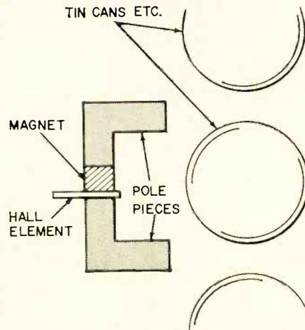
Fig. 5—Sensitive to changes in magnetic flux, the Hall device is useful for counting ferrous objects such as beer cans.
