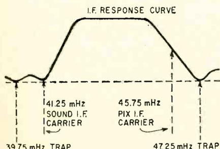
Fig. 2—Typical TV i.f. response curve showing the carrier and trap frequencies.
