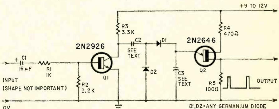
Fig. 2—Diode pump counter.
