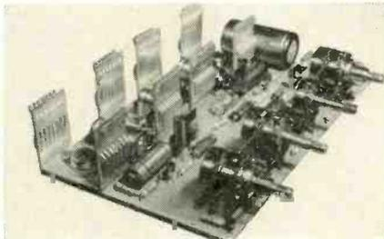
10W (per channel) at 1 kHz and 8 ohms; current: 35 mA (idle) 560 mA (max.). Frequency response: 30 Hz–50 kHz at –3 dB.—Amperex Electronic Corp., Distributor Sales Dept.
