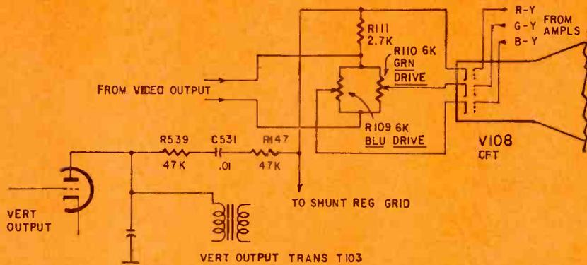
Fig. 5—Vertical blanking circuit used in the G-E 12-inch color TV CB chassis.
