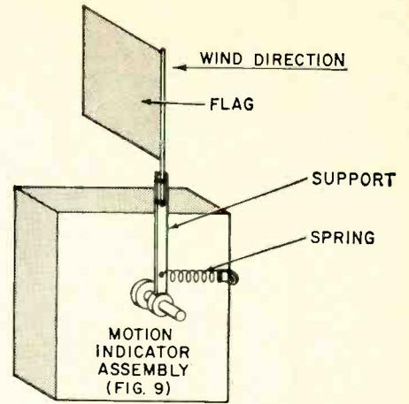
Fig. 10—Using the shaft-position indicator (Fig. 9) to show wind velocity.
