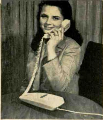
**Telephone uses IC's**—An experimental electronic telephone recently shown by Bell Labs uses hybrid integrated circuits and a tone ringer instead of an electro-mechanical bell. Buttons for Touch-Tone dialing are behind the earpiece. Automatic voice loudness circuits in the handset are among the features in the new design.
