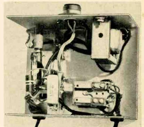
Power relays are useful in dozens of projects, but usually lack sensitivity because of heavy contacts. Find out how to soup-up relay sensitivity and trigger 30-amp jobs as little as 200  $\mu$ A.
