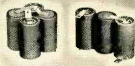
Save more than 50%. Long life—accept 300 charge and discharge cycles. 1.25 Volts per cell—750 milliampere hours capacity. Excel. charge retention. Hermetically sealed. Indefinite storage life. Multiple cells welded in series—easily cut. Combine to form battery. 7/8" dia. x 5 1/2" high. Spec. price for 100 up. Low-cost charger separate.
