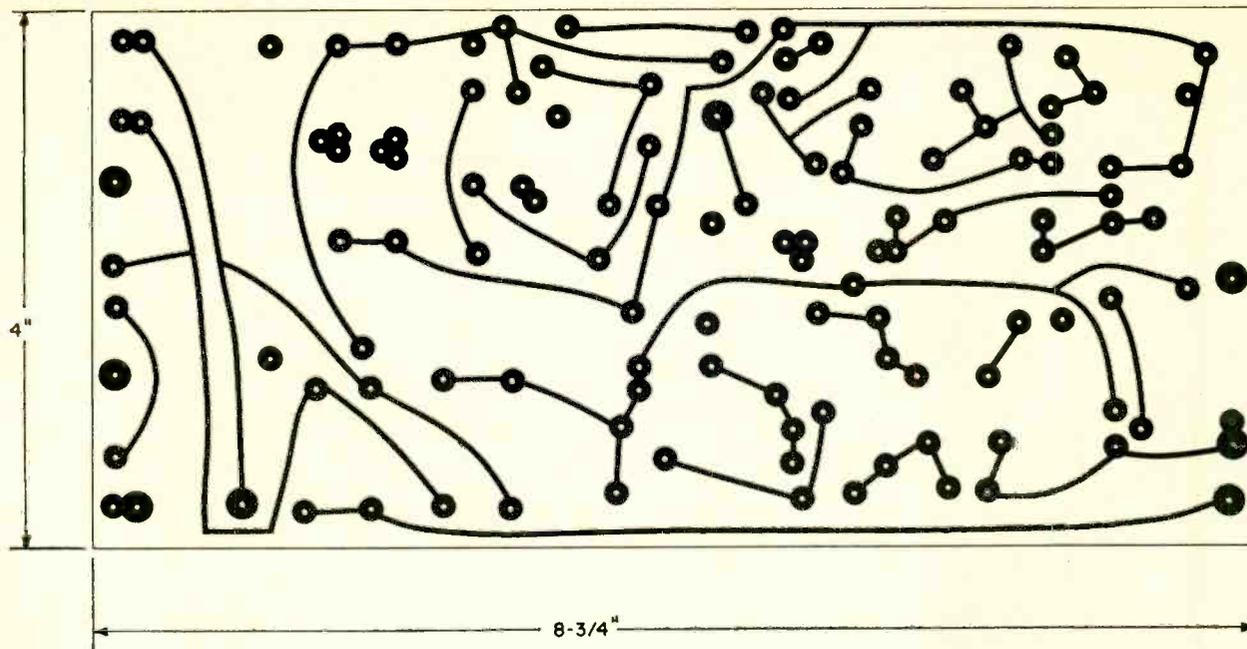
Fig. 3—Use this pattern to make the printed board for Rhythm Lights. You will need a copper-clad board 9½" x 5½", a pint of etching liquid, 1/16" resist tape, 3/16" resist circles, and a plastic container in which to immerse the board for etching.
