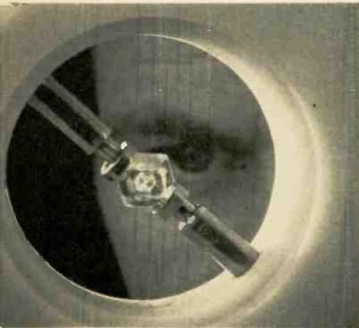
**Light transducer**—Light transmission through a "sandwich" of this crystal and Polaroid sheet can be varied by changing voltage applied to the crystal. The crystal (hexamethylenetetramine) is compressed for studying electro-optic and piezoelectric effects that influence light polarization. General Motors Research Labs "grew" material from original "seed" crystal.
