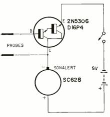
The circuit consists of a Darlington amplifier (G-E 2N5306/D16P4), a Sonalert, 9-volt battery and a spst switch in series as shown in the diagram. The plastic cap from a small spray can was used to house the switch, Sonalert and battery. A pair of thin flexible insulated leads go to the emitter and collector of the 2N-5306. The base and collector leads are used directly to form the probes.
