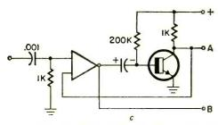
Fig. 5—These are monostable multivibrator and delay circuits. Basic circuit in a requires a brief, dc-coupled input. With circuit in b, the output is variable over a 10:1 range. High-gain transistor in c permits long time delays of output.
