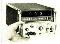
circuitry is fully floating, with more than 10,000 megohms isolation between input ground and chassis or power-line ground. Automatic polarity displays on the main frame readout on all ranges when measurement is made. \$450.—Hickok Electrical Instrument Co.
