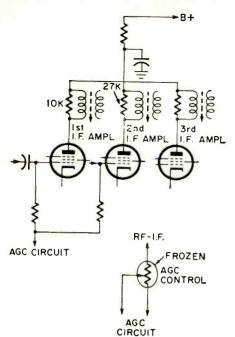
Fig. 5—Low B+ in the i.f. circuit may indicate a bad component in the agc line. Trouble here was found with bias box, pointing to a bad agc control.
