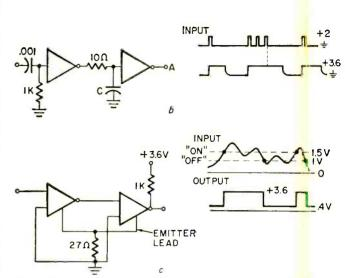
Fig. 6-a—Nonregenerative pulse stretcher in this circuit requires an input staying at ground for duration of the output. The nonregenerative monostable in b is controlled by last pulse in input chain. A Schmitt trigger is shown in d.
