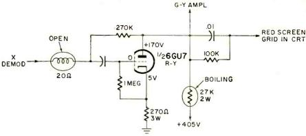
Fig. 6—A low B+ reading on the grid of the R-Y amplifier indicated the CRT was not causing loss of red in the picture. Changing the boiling 27,000-ohm resistor in plate circuit did not correct the problem. When the tube was pulled, no voltage was present on cathode or grid socket pin, indicating no voltage bleed from the previous stage. Open peaking coil upset bias and circuit operation.
