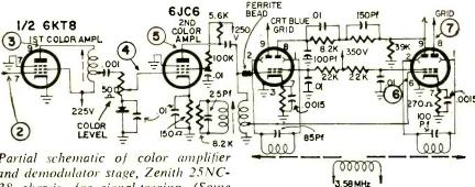
Partial schematic of color amplifier and demodulator stage, Zenith 25NC-38 chassis, for signal-tracing. (Some 3.58 MHz traps, etc. have been left out.) Numbers in circles indicate waveforms found at these points in corresponding figure numbers.
