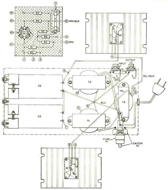
Assemble the components on perf board as shown in the drawing (upper left). Connect this board to other circuit
