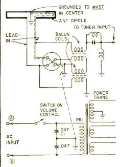
and the set is plugged in so that terminal A of the ac line is on the ground side, you have a complete circuit whether the switch is on or off. (All ac lines are ground on one side and
