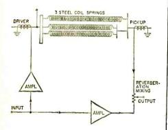
Fig. 4—A typical spring reverberator.
