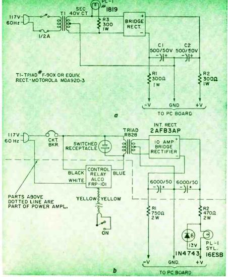
Fig. 2-a—Use this circuit to build a separate power supply if you are not building the pwr amp described last month. (Connections to this amp are in b.)
