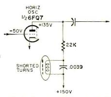
Fig. 2—Low B+ here was result of lowered hias on oscillator grid, which in turn was caused by a faulty plate-circuit component. Shorted coil had changed oscillator frequency.
