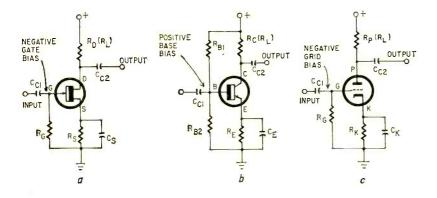
Fig. 6-a—N-channel JFET requires negative gate bias. b—Npn bipolar transistor requires positive base bias and triode tube (c) needs negative grid bias.
