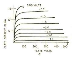
Fig. 5—Typical curves (a) for JFET, (b) for bipolar transistor, (c) pentode.
