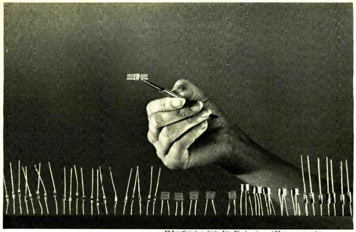
50 functions in a single chip. The functions of 50 séparate transistors, diodes, resistors and capacitors can now be performed by the tiny dot in the center of the integrated circuit held by the tweezers.
