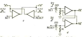
Fig. 4—Various configurations of bistable multivibrators. In a, two one-input gates are back to back. Part b shows same circuit wired for pushbutton operation. Circuit in c uses two-input gate for a pulse set-reset latch. The pulse-coupling, set-reset flip-flop in d triggers with long input pulse.
