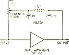
Fig. 3—A resonant filter can be made from a passive filter by adding amplifier with positive feedback. When gain exceeds circuit attenuation, oscillation occurs at filter's resonant frequency.
