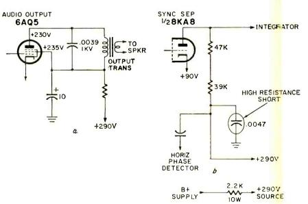
Fig. 4—Single bad component caused sound and sync trouble. The  $6AQ_5$  in a had a very low B+ since a shorted capacitor in b shunted B+ to ground.
