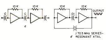
Fig. 9—Biasing scheme for class-A amplifier operation of gates is shown in a and the equivalent circuit in b. Circuit in c is gain-of-400 amplifier, and d is a crystal oscillator.
