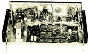
Circuit Board-Wiring Harness Construction. Note the extremely clean, another advantage of integrated circuitry. The Video board is upper left, the Divider board mounts on the chassis.
