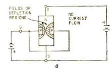
Fig. 3-a,-b-Increasing gate bias enlarges fields and pinches off the drain current. h
