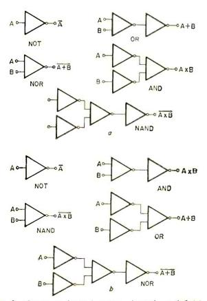
Fig. 2—Computer logic functions depend on definitions. Top (a) drawings show positive logic: "1" is positive and "0" is ground. In negative logic (b), "1" is ground and "0" is positive.
