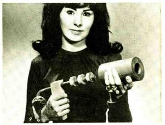
New space gun? No—a new type of piezoelectric lock being held by a pretty member of Sandia Corp.. part of the Bell System, where it was developed. The ceramic rings expand or contract, depending on the direction of applied current. Once the rings
