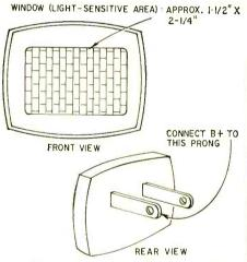
When operated on 90 volts dc (battery or simple power supply), this device passes a dark current of 14  $\mu$ A. When illumination is supplied by a 75-watt lamp 1½ ft. away, the light current is 200  $\mu$ A. Bright sunlight gives 420  $\mu$ A. This is ample current to close sensitive dc relays having internal resistance up to 2,000 ohms, and to provide a sensitive light meter.
