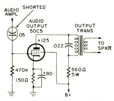
Fig. 3—Shorted blocking capacitor on control grid cut B+ to about 20 volts.
