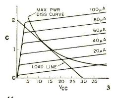
—and assuring the circuit will not allow excessive power dissipation.
