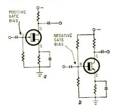
Fig. 7 (above)—Polarities of p-channel JFET (a) and pnp transistor (b) are opposite from those in Fig. 6.
