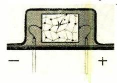
Fig. 1—If ovonic material is placed between two electrodes and a voltage is applied, the voltage exerts a pull on the trapped carriers, marked e in figure.
