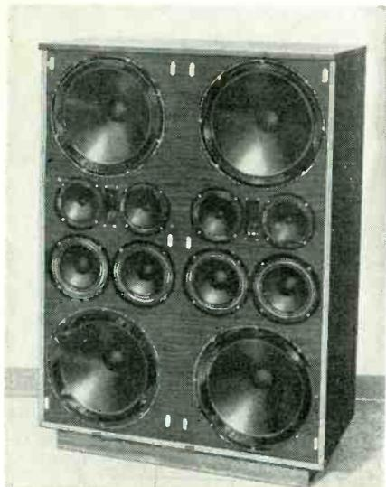
per channel minimal power requirement. Electronic network generates negative-feedback error voltages when speaker does not follow amplifier output and controls speaker cone to eliminate low-frequency distortion. Network tends to cancel effect of frequency-sensitive net-
