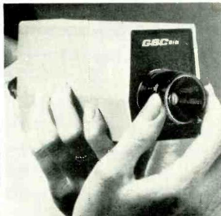
Miniature monitor camera works with a 5-inch screen set. Size keeps this compact system out of the way.
