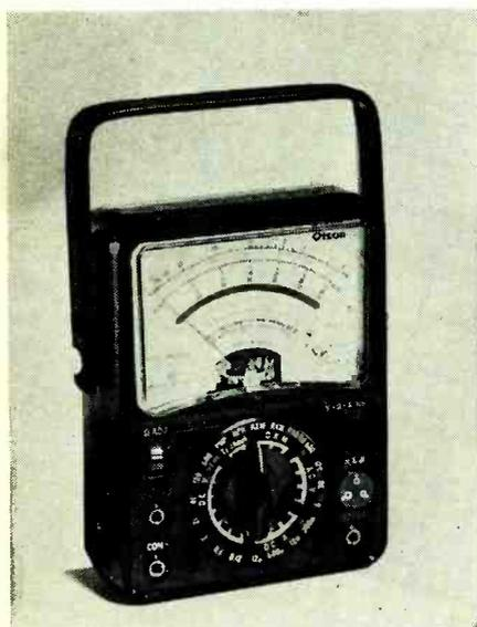
Another vom model. Used for engine tuneup, a diode must be series connected with a lead to block current from coil primary.
