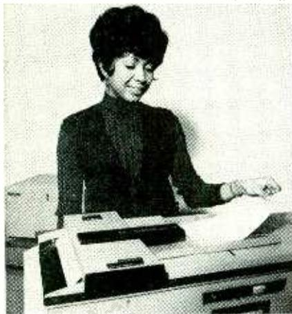
Speedy fax transmission system saves time by rapidly scanning white space between the lines.
