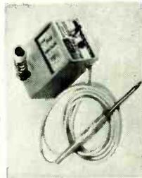
Fig. 9—Variable heat controls keep a soldering iron at a constant operating temperature so it is always ready to use. These units are particularly useful in production applications. Unit shown is made by Weller.
