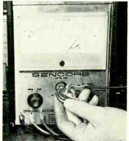
High leakage in power output transistors is spotted quickly on this beta tester.
