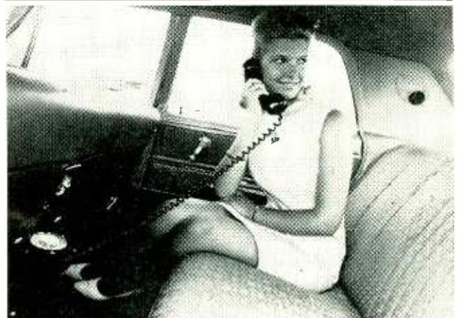
Automatic dialing with a mobile backseat extension phone is now possible with an improved radio telephone system developed at Bell Telephone Labs. With the compact units, you can have direct access to the telephone network without assistance from an operator. The units provide simplified controls, more radio channels and greater privacy. The improved mobile service is gradually being introduced in major cities across the U.S.
