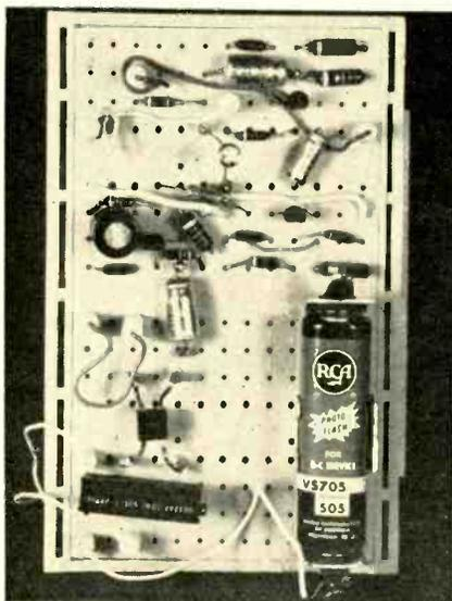
**CIRCUIT-BOARD** closeup shows how the author assembled his electronics.
