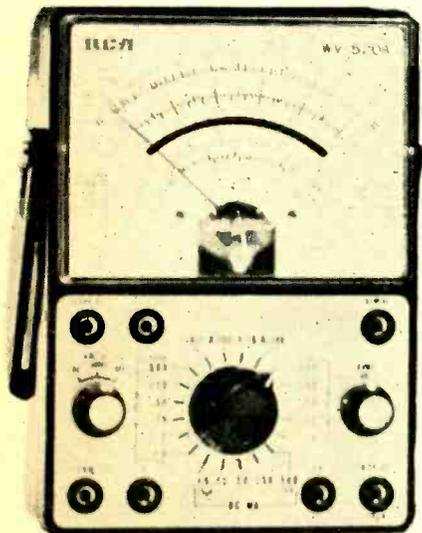
measurements and 10,000 ohms-per-volt for ac measurement; measures dc voltages from 10 mV to 1,500 volts; ac voltage (rms) from 100 mV to 1,500 V; dc current from 0.5 mA to 5 A; resistance from 0.05 ohm to 20 megohms, and decibels from -20 to +55.5. Prices are \$9.95, \$18.00, \$28.50, \$36.00, \$48.00 respectively.—RCA/Electronic Components, 415 South 5th St., Harrison, N.J. 07029.
