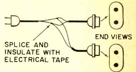
polarized. This can pose a minor irritation to the service technician as he needs to apply power to these sets to check and adjust them, and may not have at hand a cheater cord with the proper receptacle (female end).
