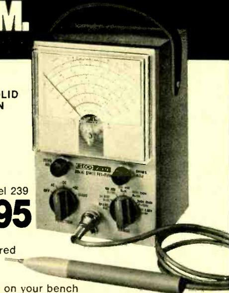
Use the new 239 on your bench or in the field. Checks semiconductor and vacuum tube circuits. 11 Megohm DC input impedance. Reads AC rms and DC voltages in seven 10db steps from 1 to 1000 volts on large 4 1/2" meter. Measures and reads peak-to-peak AC to 2800 volts. Check resistance from 0.2Ω to 1000 MΩ on seven ranges. Includes exclusive time-saving Uniprobe.
