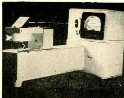
**THREE-QUARTER VIEW** shows the construction of the photo densitometer.
