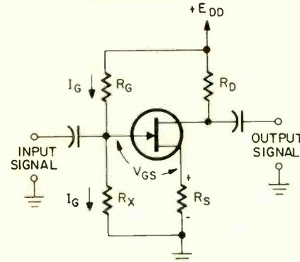
FIG. 4—PRACTICAL VERSION of circuit in Fig. 3 using only one power supply.
