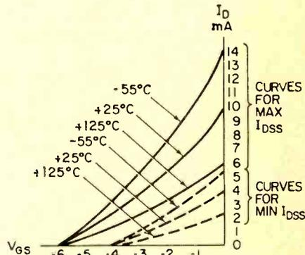
FIG. 9—THE SOLID LINE 25°C plot is the transfer characteristic curve for the maximum value of  $I_{DSS}$  of a hypothetical JFET. The broken line 25°C curve represents the transfer characteristic for the minimum value of  $I_{DSS}$ . The other curves are maximum and minimum values at extreme temperatures.
