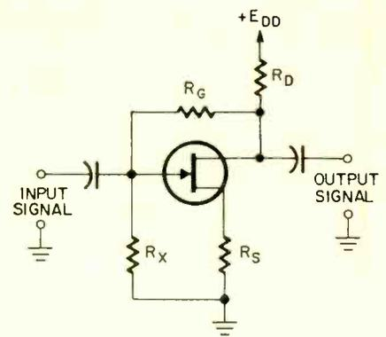
FIG. 6—THE BIAS CIRCUIT is improved by adding dc feedback from the drain to the gate of the FET.
