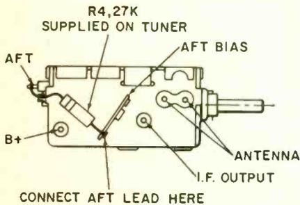
to 27,000 ohms. In first version incorporating the change, the resistor is connected directly between the aft lead from the main chassis and the aft terminal on the tuner. Current versions have the 27,000-ohm resistor connected between the aft terminal on the tuner and a terminal strip mounted on top of the tuner.
