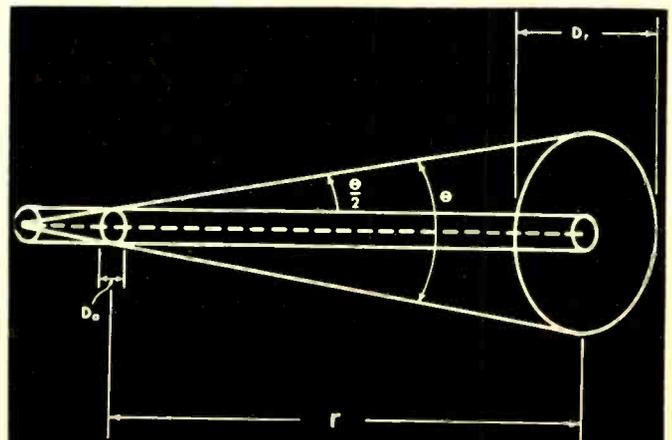
FIG. 14—LASER BEAMS DIVERGE slightly as they travel beyond the laser aperture. This diagram shows divergence characteristics
