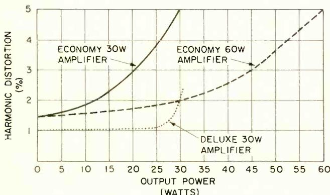
FIG. 1—DISTORTION DECREASES as amplifier output power is reduced.
