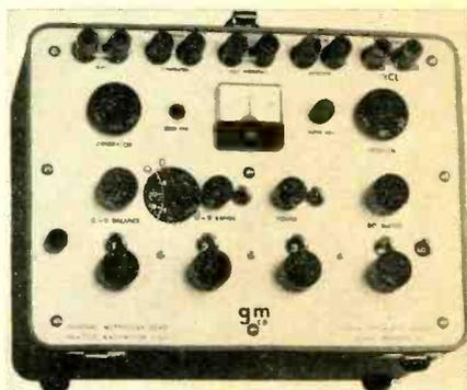
placement and range-units display. Operates from battery or ac 50 to 400-Hz power. Accuracies of  $\pm 0.05\%$  for resistance and  $\pm 0.2\%$  for capacitance or inductance. \$510.00.—General Metrology Corp., Box 471, Edmonds, Wash. 98020.
