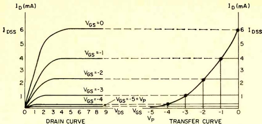
FIG. 7—THE TRANSFER CHARACTERISTIC CURVE is derived from the drain characteristic display of Fig. 1.
