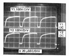
FIG. 5-TYPICAL GRID-DRIVE WAVEFORMS. Are they good or bad?
