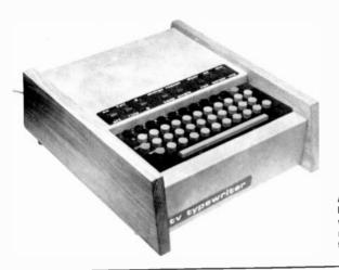
A SURPLUS KEYBOARD is used in this version of the TV typewriter. Unit on cover has a homemade keyboard based on the article in the February issue.
