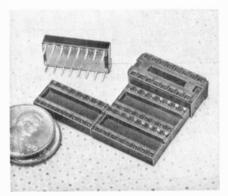
FIG. 6-NEW MOLDED SOCKETS for DIP devices are unusually shallow. They have tapered holes so the IC pins go in easily.
