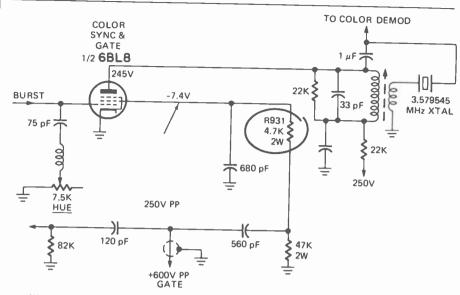
you'll have no gating pulse on the 3.58-MHz signal to the crystal and no color sync at all. This is R931.
