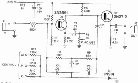
IN THE BAND-PASS FILTER, diode D1 replaces the shunt resistor in the parallel-T fliter. Control votages vary D1's impedance and modify the filter's center frequency.
