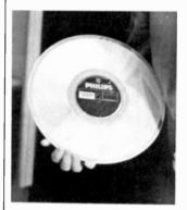
PHILIPS VIDEODISC is brightly silvered optical type used in their laser TV disc system.
