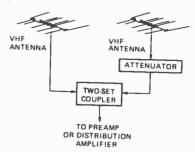
FIG. 3-TWO ANTENNAS are handy when signais come from opposite directions.
