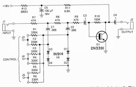
THE LOW-PASS FILTER IS A PI NETWORK feeding the base of Q1. Series diodes tune the filter by varying the impedance of the shunt (capacitive) legs.
