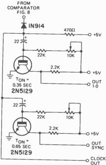
1.0 & SYNC DETECTORS USED IN ABSENCE OF PLL FLYWHEEL FIG. 10—SYNC DETECTOR extracts the 1's and 0's from the WWVB incoming signal.
