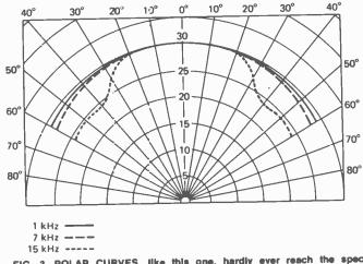
FIG. 3—POLAR CURVES, like this one, hardly ever reach the spec sheet. They show speaker dispersion. Numerals down the center are in dB.
