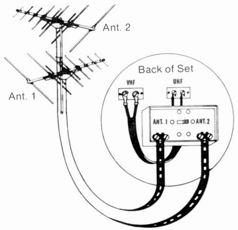
ANTENNA SWITCH-SPLITTER divides uhf and vhf signals from two separate antennas through a switching network. Photo courtesy Winegard Co.
