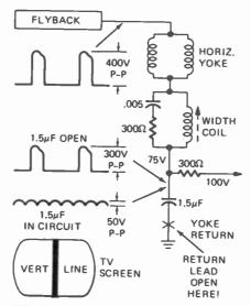
FIG. 1—TRAPEZOIDAL WAVE is a combination of sawtooth and rectangular pulses. FIG. 2-OPEN YOKE was not the trouble in this circuit. See text for details.
