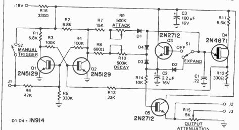
BISTABLE MULTIVIBRATOR, Q1-Q2, is the heart of this function or envelope generator. Fixed and variable outputs are at J2 and J3, respectively.
