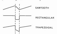
of practical inductors having both resistance (sawtooth) and reactance (rectangular) that, together, form a trapezoid.
