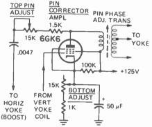
the pin-phase *transformer*, to the right of the tube in the diagram. If you'll notice, the dc path to the resistors is *blocked* by the .0047- $\mu$ F capacitor. Nothing but pulses *should* come through here.
