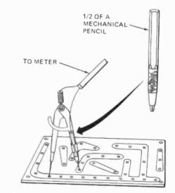
of a mechanical pencil or ball-point pen with a metal cartridge. A needle is forced into the tip of the pencil or pen. The test lead is thin coax cable with its core soldered to the pencil tip (the *positive* prod) and the shield (the *negative* lead) is soldered to the body of the compass at the top. Connectors on the other end of the cable match your meter.-Peter Legon **R-E**
