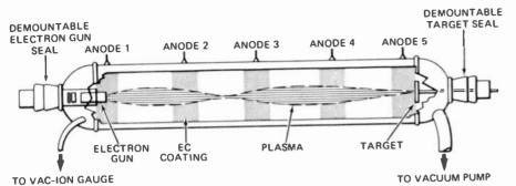
FIG. 1-CUTAWAY VIEW of a demountable plasma tube. Note that each segment has a separate anode connection.
