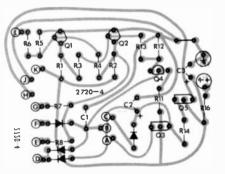
ENVELOPE GENERATOR parts layout is above. It's haif-size foil pattern is at right.
