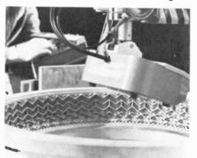
BETTER TIRES PRODUCED BY LASER. A new laser measuring instrument introduced by Siemens checks the accuracy of tire molds with precision heretofore unattainable. Because the dimensional stability of these molds vitally affects the characteristics of the tires that are made from them, the device makes it much simpler to make tires that run round. Measurements are made by a sort of radar principie, the laser beams being bounced from the tire to a reference plane.
