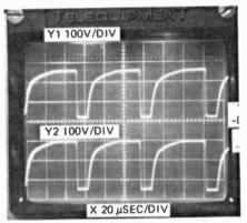
FIG. 8-NORMAL WAVEFORMS. Replacement pincushion transformer restored operation.
