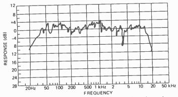
FIG. 1-FREQUENCY RESPONCE CURVE of a typical speaker system. This is a point-to-point plot.
