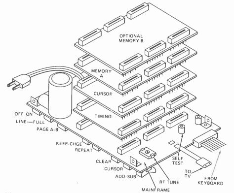
HOW TYPEWRITER ELECTRONICS IS ASSEMBLED within the case. The timing, cursor and memory boards plug into the mainframe and each other, cordwood fashion.
