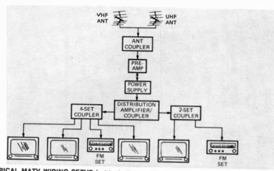
FIG. 1-TYPICAL MATV WIRING SETUP in block diagram form, Remember this is a system for a one-family home and is, therefore, relatively simple.
