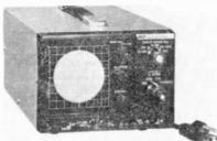
1 megohm shunted by 30 pF. Continuously variable gain control range is greater than 22 dB. There are four timebase ranges from 10 Hz to 100 kHz, continuously variable between ranges.
