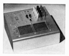
connections with external equipment such as a scope, oscillator or additional power source and 18 LED indicators which show the status of the IC under test.
