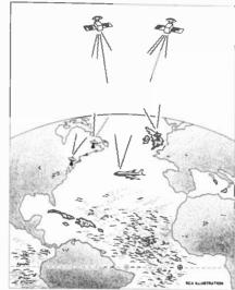
AERONAUTICAL SATELLITE PROGRAM would use two geostationary satellites, working with ground stations to provide exact position information on and direct communication with the aircraft during the whole transatiantic flight.
