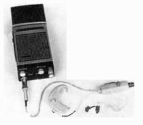
PERSONAL COMMUNICATION HEADSET uses a conventional acoustic earphone, with a bone-conduction microphone. The control unit, at left, has a push-to-talk switch and a volume control. Button shown on the earborne unit is the microphone contact, which is worn toward the head in use. Lead between the ear unit and control is longer than shown (note cut lead).
