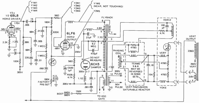
FIG. 3—HORIZONTAL DEFLECTION CIRCUIT of Motorola CATV5/6. Symptoms: no high voltage; horizontal output tube plate red. Horizontal and vertical deflection circuits are often problems. This month we will look at typical circuits used in today's vacuum tube and hybrid receivers
