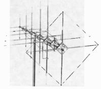
the ionosphere. When the skip changes, polarity can be changed to eliminate the unwanted interference. 311/2-foot boom; 17 dB gain over isotropic, 44 dB rejection, 24 dB side rejection and 1.2:1 SWR.-Avanti Research & Development, 33 West Fullerton Avenue, Addison, III. 60101.
