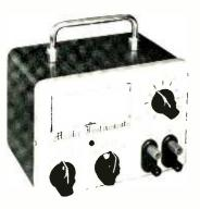
into 600 ohms and 10 mV into 250 ohms. The instrument can be used as an audio voltmeter with 400K input impedance and fullscale with 400K input impedance and ruliscale ranges of 1 mV to 100 Vrms in eleven 10-dB steps. Frequency response (-6-dB points) is 0.3 Hz to 100 kHz. The -10 to +2-dB scale is referenced to 1 mW into 600 ohms. Powered by eight "C" cells.
