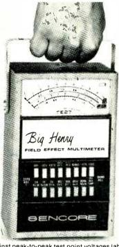
against peak-to-peak test point voltages labeled on schematics. Sensitivity provides eight overlapping voltage ranges between 0.3 volts and 100 volts full scale, dc and ac. Current range covers dc from 10 mA to 1 amp full scale and five ohm ranges measure resistances from .1 ohm to 1000 megohms. \$150.00—Sencore, Inc., 3200 Sencore Drive, Sioux Falls, S.D. 57107.
