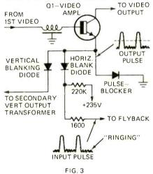
fed into the emitter of a transistor video amplifier stage.
