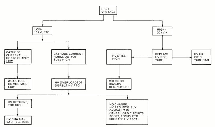
TROUBLESHOOTING CHART helps you find and eliminate defects in high-voltage regulator circuits fast and efficiently.
