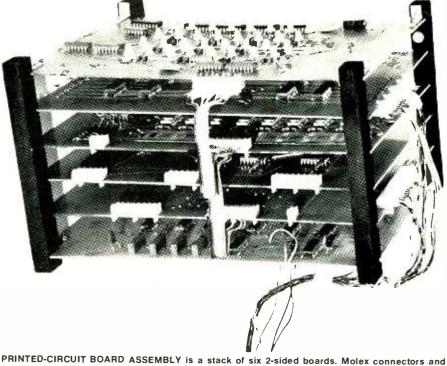
cables are used to interconnect the boards and to connect the boards to the front-panel controls.
