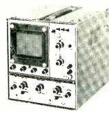
IN-LINE READING DIALS show attenuation at a glance on the *Hewlett-Packard* 4436A (shown) and 4437A decade attanuators. Both have a maximum attenuation of 119.9 dB in 0.1-dB steps. Frequency range is dc to 1.5 MHz (0 to
