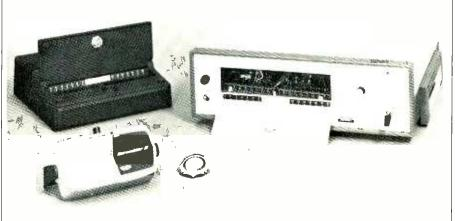
BOEING SCRAMBLER II EQUIPMENT. At left is the mode selector, normally mounted on the dashboard; behind it the code processor, with the lid raised to show its 18 code-setting switches. At right is a Scrambler base station.
