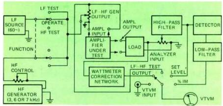
FIG. 3—BLOCK DIAGRAM of the Heathkit audio analyzer used for intermodulation measurements. The instrument also functions as an audio vtvm and as an audio wattmeter.
