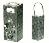
using a 3-kHz tape calibrated for 3- $\frac{3}{4}$  ips and then using the same tape as a 6-kHz test source for  $7\frac{1}{2}$  ips. Test range -3% to +3%. Input level 100 mV to 10 Vrms. Input impedance 150K.
