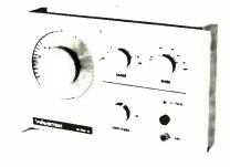
linear or logarithmic manner. Sweep speeds are 2.5 ms, 25 ms and 25 seconds. Output: High-level sinewave variable up to 1 Vrms. Low-level sinewave is approximately 1% of the high-level output setting. Squarewave with 50% duty-cycle at nominal TTL levels (0 to +0.5 V low and +3 to +4.5 V high). Triangle (output on rear panel) 1 Vp-p, less than 2 mA peak current.
