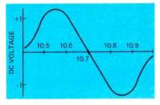
FIG. 4----TYPICAL RATIO-DETECTOR "S" curve swings over wide positive and negative dc voltage range. For proper tuning, 0 dc point must be exactly 10.7 MHz as shown.
