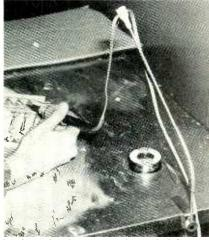
ing board. These were intended for use on the end of an ironing board to prevent ironing over the cord, etc., but works equally well holding the soldering iron cord up out of the way. The holder installs on the edge of a table or work-bench and is secured by a thumbscrew. - Kent Mitchell, W3WTO
