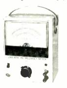
mW across 600 ohms) is -8 to +52 dB and bandwidth is  $\pm 1$  dB 10 Hz to 1 MHz. Amplifier output is approximately 500 mVp-p at fullscale. Operates from 105—125 V, 50/60 Hz.
