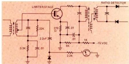
FIG. 2—CONNECTION POINT FOR TYPICAL "signal-strength" FM tuning meter.
