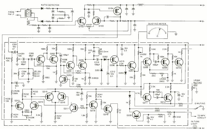
FIG. 5—PARTIAL SCHEMATIC OF HARMAN-KARDON 900+ showing complete "quieting meter" and "in-tune light" circuits.
