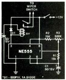
R1 and C1 set the width of the negative-going pulse and thus the period of time that power is applied to the wiper motor. The positive-going pulse width is adjustable independent of the negative-going pulse by the combination of R1, R2, R3, and C1. This is the interval between active cycles.
