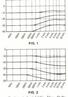
equalization at about 3 kHz. Thus, Dolby provides the full 10 dB noise reduction 2 kHz below that of the ANRS. In terms of listening sound quality, though both systems deliver excellent noise reduction, the Dolby sounds slightly more quiet or "hiss free."
