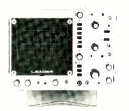
Vp-p square wave calibrating voltage is available at a jack on the front panel.
