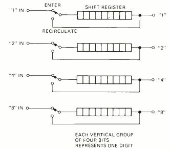
FIG. 6—TYPICAL MEMORY in memory stack. Length of shift register depends on number of numerals and sign digits to be shown.
