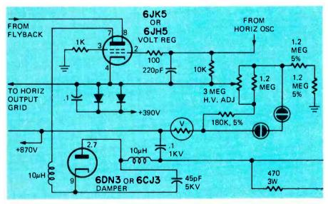
FIG. 5—HIGH-VOLTAGE HOLD-DOWN CIRCUIT used in some pulse-type high-voltage regulators. Neon lamps limit the high voltage if the adjustable control shorts.
