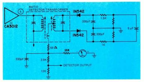
FIG. 3—CONNECTION POINT FOR CONVENTIONAL "center-of-channel" FM tuning meter.
