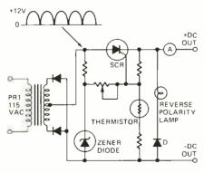
you can see, the transformer and rectifiers are still there. The positive terminal of the dc output (center-tap of the transformer) is connected to the anode of the SCR. The negative terminal of the dc output is the common anodes of the rectifiers. So now the charging current flows through the SCR.
