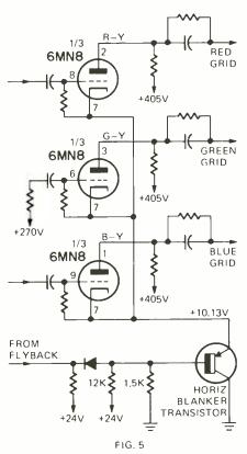
A shorted blanker transistor, in the same chassis, will cause one dark bar on the screen, with an otherwise blank raster. Same as before; it's in the cathode circuit of the 6MN8 color difference amplifier tube. Upsets the bias (see Fig. 5). **R-E**
