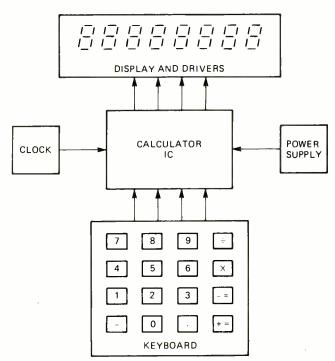
FIG. 1—CALCULATOR BLOCK DIAGRAM. Keyboard generates 4-bit BCD numerals. The clock — a multivibrator — controls operational sequence.
