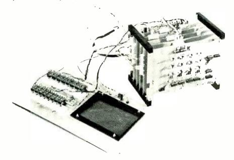
THE WORKING HEART of the computer is relatively simple. The six primary circuit boards and the front-panel controls are shown here. If additional memory is needed, more circuits boards are required.
