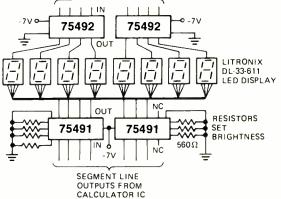
(b) FIG. 3—DISPLAY DRIVERS ARE NEEDED when the calculator IC cannot handle the current or the voltage required by the readout.
