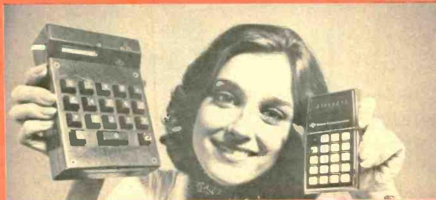
A BASIC PATENT covering miniature calculators having their main electronic circuitry in a single chip has been issued to Texas Instruments, Inc. The model is shown holding (at left) the world's first mini-calculator that contained the equivalent of thousands of discrete devices. It was the first mini-calculator at the time to have the high degree of computational power found only in large machines. The 1974 version (still smaller) is the one at the right.
