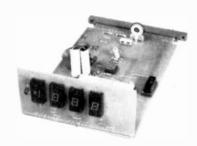
FEATURES • BASIC 2 RANGE DVM ACCURATE TO 1%. CIRCUITS FOR ADDITIONAL VOLTAGE RANGES, OHMS, D.C. CURRENT, AND A.C. VOLTS CAN BE ADDED. PARTS MOUNT ON EDGE CARD CONNECTOR P.C. BOARD. DISPLAY BOARD HAS EASY TO READ 1/3" LED'S AND CAN BE REMOTE MOUNTED.
