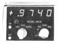
tivity is 100 milliohms. DC voltage accuracy is 0.1%. AC and DC voltage ranges of 1, 10, 100 and 1000 volts are provided. Resistance ranges
