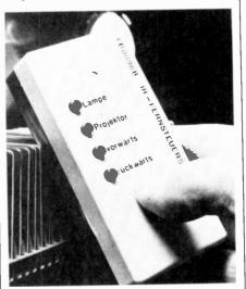
NEW INFRARED REMOTE CONTROL. Channels are Lamp (electric light for room illumination) Projector, Forward and Back.
