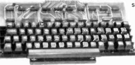
Operates on the scan principle utilizing TTL logic. With repeat key, negative/positive going data valid strobe, latch outputs, shift and shift-lock capability. True/false ASCII outputs, 6 extra control keys. With all necessary parts, including TTL components. Does not include test jigs, optional features or case and hardware. See store sales persons for parts list. 277-117. Complete Pkg. **Sale 49.95**
