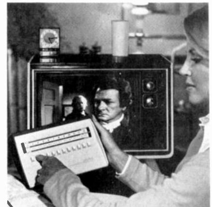
without motors, this solid-state unit provides direct-access channel changes, fine tuning and remote on-off of a TV set from anywhere in the room. The device consists of two units; an all-channel converter and a control unit interconnected by a 25-foot, plug-in, control cord. The converter is connected behind and beneath
