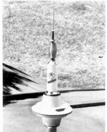
antenna mounted on the center area of the roof of a truck cab is 3 dB above isotropic. The average VSWR is less than 1.3 without making any attempt to optimize this figure. Model *A-280* is base-loaded, mobile, magnetic-mount with a 47-inch heat-treated, stainless steel whip. Antennas are factory matched to resonate at 146 MHz. A chart is provided allowing adjustments ranging from 144 MHz to 156 MHz.—Antler Antennas, 6200 South Freeway, Fort Worth, TX 76134
