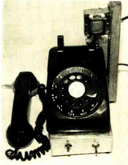
FIG. 2.—AUTODIALER WITH SOLENOID that pulses the cradle button. The two toggle switches in the base are not used.
