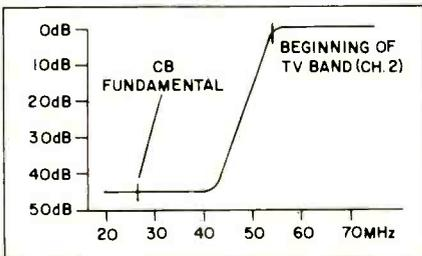
Fig. 1 High-Pass Filter
