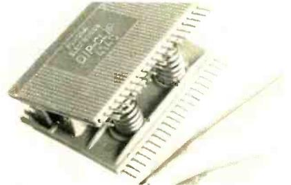
for attaching test probes permits handfree testing. Has nontarnishable nickel-silver contacts; lower contacts measure 1.022 mm wide and mate with DIP contacts, square, serrated upper-end test points measure 0.63 mm and are designed for mini test clips. Nylon casing can withstand temperatures to 240°C. Price: \$19.95.—**ITT Pomona Electronics**, 1500 E. Ninth St., Pomona, CA 91766.
