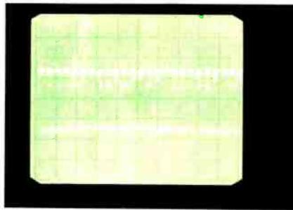
FIG. 4—CHOPPED-MODE DUAL TRACE appears like this at faster sweep speeds (shorter sweep times). Alternate mode is better when sweep time-per-division is 0.1 ms or less; chopped mode at 0.2 ms or more.
