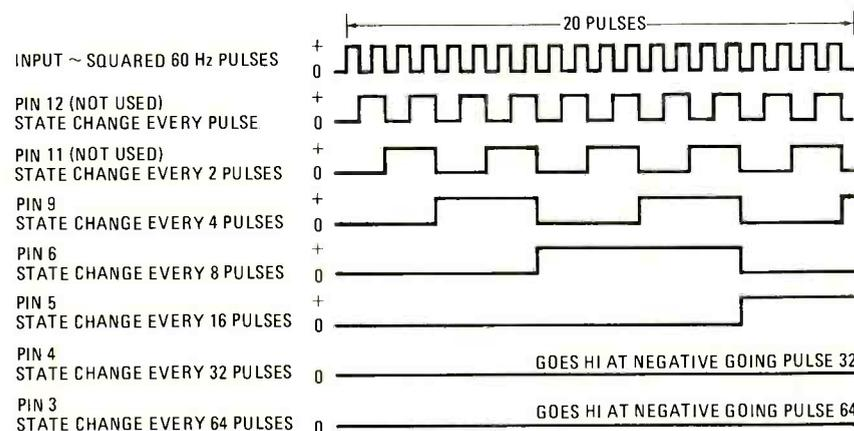
FIG. 10—OUTPUT PULSES as related to input to binary counter IC3. For example, output signal at pin 9 changes state for every four input pulses on pin 1.
