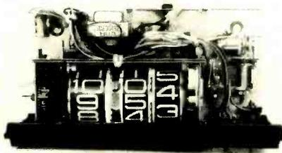
**SANKYO 803AL.** The digits are printed on translucent drums, driven by a clock motor. A single incandescent bulb lights the number drums from inside. The "chimes" are played by motor-driven music box.
