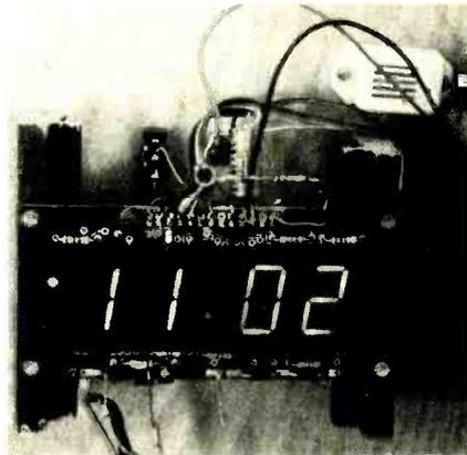
**SOLID-STATE TIME** alarm buzzer is driven by a simple transistor circuit wired directly to clock module.
