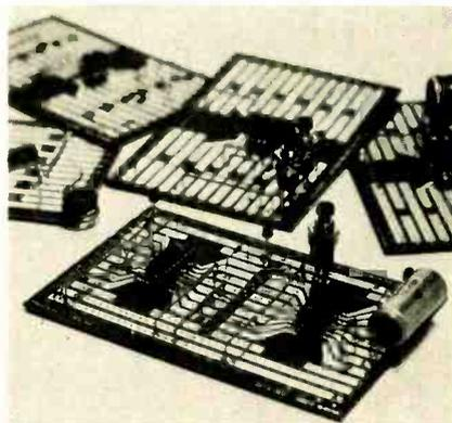
BLOB-BOARDS with prototype circuits built on them.
