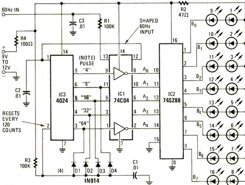
NOTE: EACH FOURTH NEGATIVE-GOING INPUT PULSE CAUSES ONE OUTPUT LINE TO GO POSITIVE IN BINARY SEQUENCE. SEE FIGURE 10.
