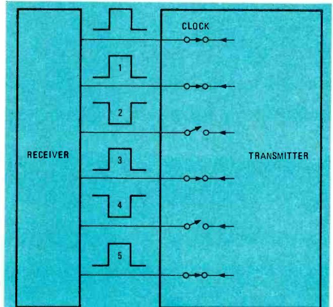
**FIG. 2—BIT-PARALLEL TRANSMISSION.** All data bits are transmitted simultaneously over five individual circuits.
