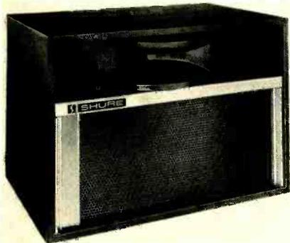
FIG. 3—SIDE WALLS OF HORN define horizontal radiation pattern while top and bottom walls define vertical radiation pattern.
