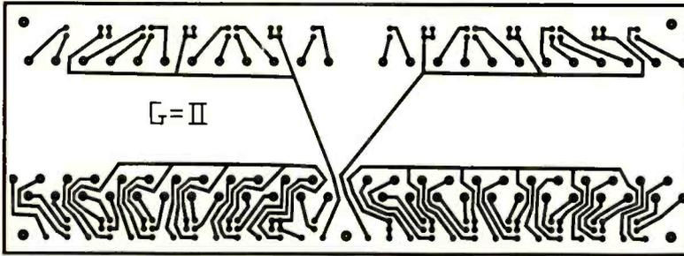
FIG. 6—HALF-SIZE pattern for control board that holds the slide pots.
