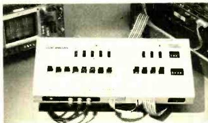
The *model 10* captures and displays the instruction and data flow on the microprocessors data bus at the occurrence of a particular 16-bit address. The combination *model 10/model 100A* package can display a 16-word deep data-domain truth table of both lower and upper
