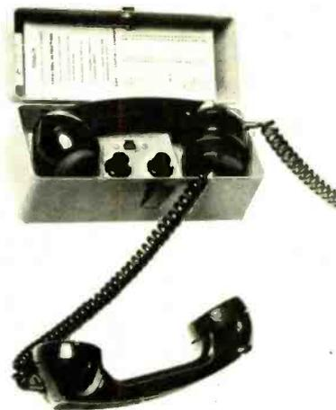
telephone from *Privacom* unit and place conventional handset into unit and talk. Unit measures 3<sup>1</sup>/<sub>2</sub> X 4<sup>1</sup>/<sub>2</sub> X 9 in. and contains 4-volt mercury battery. Price per unit, \$325 (two units needed for operation).—**Mountain West Alarm Supply Co.**, Box 10780, Phoenix, AZ 85064.
