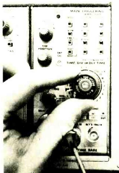
You simply delay the trigger until the signal fed into the oscilloscope reaches line 19 (or the preceding line). To view the VITS signal on lines 17 and 18, you delay the trigger slightly less.
