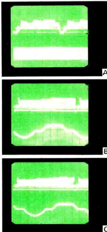
**FIG. 3—DUAL-TRACE DISPLAY LOCKS on one signal or the other, unless both are in phases. (a) Horizontal line on trace A, supply ripple on trace B and triggering from trace A; also, timebase is too fast for ripple. (b) Timebase set to accommodate 16.7-ms duration of both TV field and ripple waveform; but slight phase variance lets one crawl. (c) Composite triggering locks both displays despite minor phase difference.**
