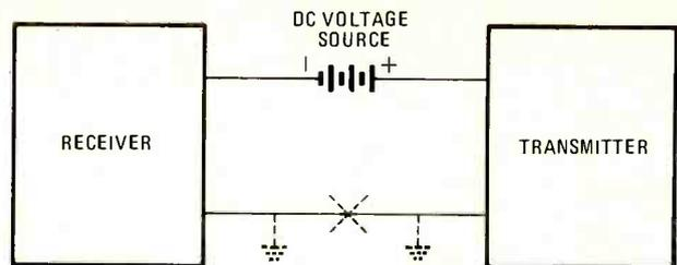
**FIG. 4—20-MIL CURRENT LOOP for serial data transmission. Some systems replace the return path with a common ground. This reduces the number of wires running between the transmitter and receiver to one.**
