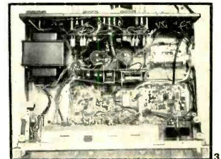
front contains the entire FM-IF, stereo multiplex, AM and tone-control amplifier circuits. Two identical vertically mounted power-amplifier modules are located near the rear of the chassis, with the power transformer on one side and the separate RF front-end on the other side. A pair of 10,000- $\mu$ F filter capacitors (for the B+ and B- output-transistor power supplies) are nestled between the two power amplifiers.
