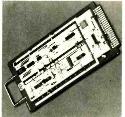
nents having lead diameters to 0.032 in. Also featured are protective rubber feet and extractor handle; predrilled buses, tin-plated copper printed circuits and glass-epoxy bases. Prices start at \$31.50 for *Unicard I*.—**A P Products, Inc.**, Box 110, 72 Corwin Dr., Painesville, OH 44077.
