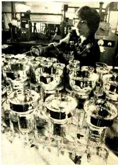
**GLASS SURFACES OF PHOTOMULTIPLIER TUBES** being treated at RCA Electro-Optics and Devices plant in Lancaster, PA. When installed in nuclear detection instruments, tubes can "see" nuclear radiation as blue flashes of light.
