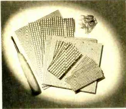
**A SELECTION OF VEROBGARDS** with various hole sizes, a spot face cutter used to break foil strips and discrete terminals.
