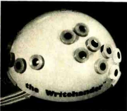
UNUSUAL DESIGN OF ASCII-encoded keyboard permits typing alphanumeric characters with one hand.
