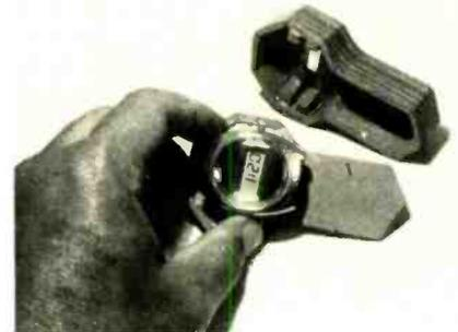
DO-IT-YOURSELF case made from balsa wood. "Clock module" is LCD wristwatch.
