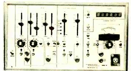
MODEL 101 AUDIO TEST SYSTEM consists of two sine/square/triangle function generators, pulse generator, frequency counter and AC voltmeter. As a system it will generate a frequency response plot on an X-Y recorder or scope.
