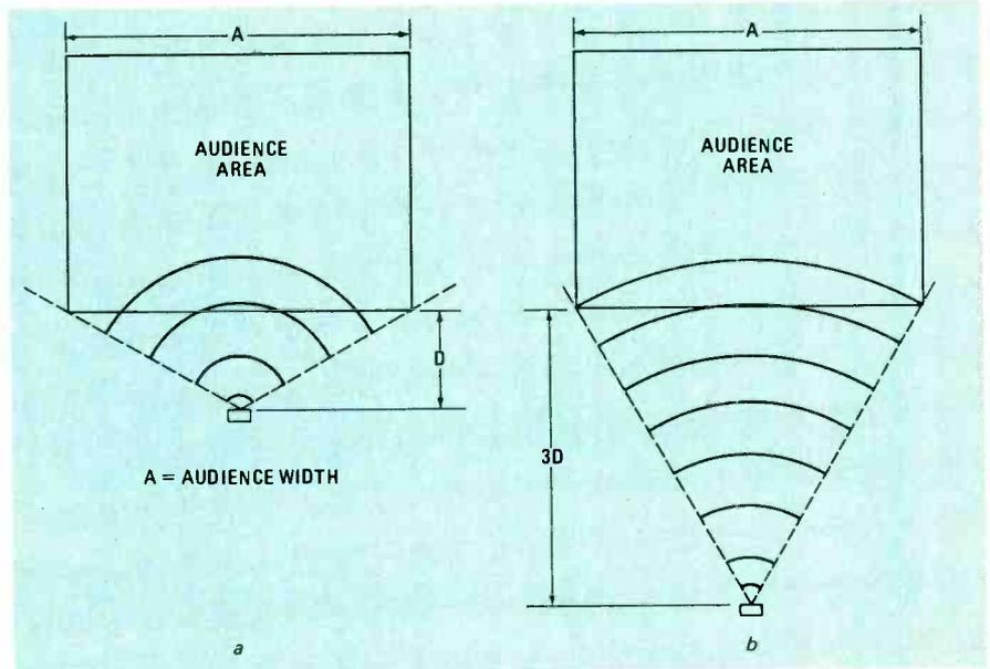
**FIG. 2—WIDE POLAR RESPONSE** enables speaker to cover greater area from a shorter distance as shown in **a**. **Narrow polar response** requires greater distance between speaker and audience to cover same area as shown in **b**.
