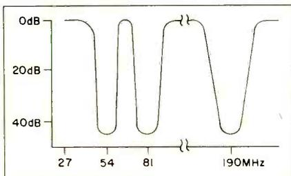
Fig. 3 Harmonic Traps for CB Transceiver
