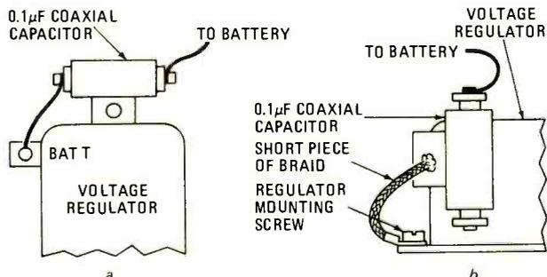
**FIG. 5—REGULATOR CAUSED NOISE** is reduced by adding a 0.1- $\mu$ F coaxial capacitor in series with the battery terminal. Two possible methods for mounting the capacitor is shown in *a* and *b*.
