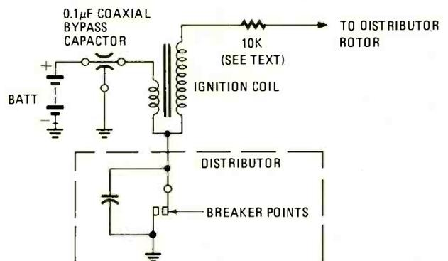
FIG. 3—KETTERING IGNITION SYSTEM was the most common before the electronic ignition system was introduced. Noise suppression involves adding a 0.1- $\mu$ F capacitor on the primary side of the ignition coil and some resistance in series with the spark plugs if the engine does not already have this resistance present. The series resistance can take the form of resistance-type ignition wires or barrel-type resistors that are inserted in the spark plug wires.
