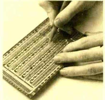
A VEROWIRE PEN being used to route heat strippable wire on a DIP board.
