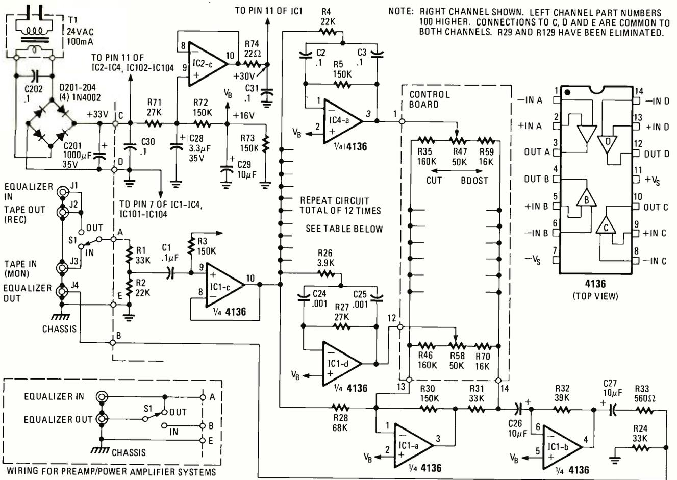
NOTE: RIGHT CHANNEL SHOWN. LEFT CHANNEL PART NUMBERS 100 HIGHER. CONNECTIONS TO C, D AND E ARE COMMON TO BOTH CHANNELS. R29 AND R129 HAVE BEEN ELIMINATED.
