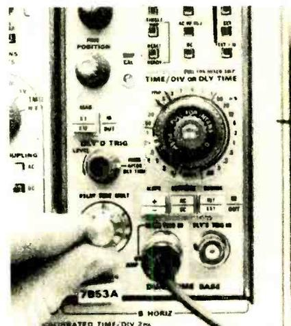
FIG. 6—VARIABLE DELAYED TRIGGER is a feature of more costly triggered scopes. Basically, a timebase determines how much of a waveform is to be viewed and a delay multiplier sets the time allowed to elapse before triggering fires the sweep.
