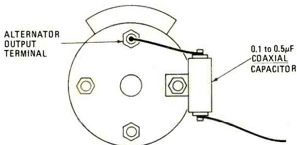
**FIG. 4—ALTERNATOR WHINE** is reduced by adding 0.1 to 0.5- $\mu$ F coaxial capacitor to alternator as shown. Check with auto manufacturer for correct value or damage may result. To further reduce noise, an L-section filter can also be added at the input power line feeding the radio.
