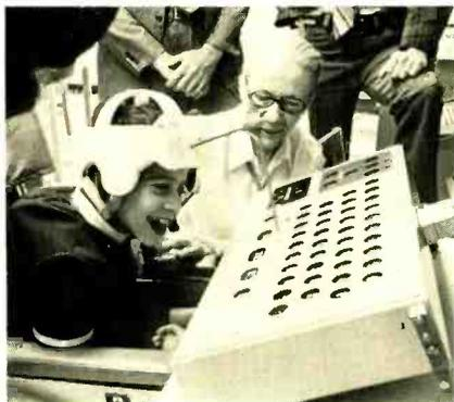
**BELL LABS COMMUNICATIONS SYSTEM, *Unix*, contains a large keyboard with recessed keys that can be used by severely handicapped persons. Here a cerebral-palsied child uses a cap pointer to type a message on the keyboard.**
