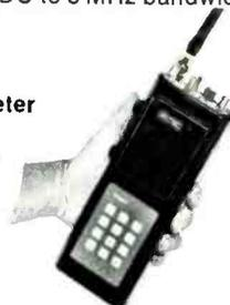
Superb features specifications and a great low price make the VF-2031 a terrific buy in a hand-held two-meter transceiver. Features 8-channel simplex with  $\pm 600$  kHz offset using one crystal per channel, minimum 2 watts out, and 0.5  $\mu$ V sensitivity for 20 dB quieting. Includes built-in antenna, nickel-cadmium batteries and battery charger. An optional tone encoder and other accessories also available.
