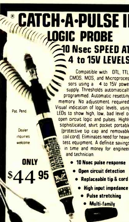
Compatible with DTL, TTL, CMOS, MOS, and Microprocessors using a 4 to 15V power supply. Thresholds automatically programmed. Automatic resetting memory. No adjustment required. Visual indication of logic levels, using LEDs to show high, low, bad level or open circuit logic and pulses. Highly sophisticated, shirt pocket portable (protective tip cap and removable coil cord). Eliminates need for heavy test equipment. A definite savings in time and money for engineer and technician.
