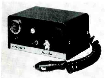
tory alert signal. Bearfinder works on all 12-volt systems, can be plugged into car's cigarette lighter, requires no license to operate, and is guaranteed not to interfere with car radio performance or CB transceivers. The Bearfinder Two + Two comes in rugged heavy-gauge metal case and carries a 90-day warranty. Suggested retail price: \$149.95.—Bearfinder, Inc., 221 Crane St., Dayton, OH 45403.
