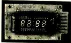
Simple to apply; requires only 3 time-setting switches and 12V DC. Ideal for car, van, or other portable use thanks to built-in timebase. Four 0.3" blue-green fluorescent digits. Extra features (such as automatic dimming) included for car use. With applications data. \$16.50 ea., 3/\$46.
