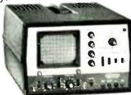
Low-priced dual-trace scope ideal for audio and TV servicing. Features outstanding sensitivity, extra-bright traces, selectable triggering, 7-position variable time base, DC to 5 MHz bandwidth.
