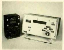
FIG. 1—PREFABRICATED PC BOARDS were used in building these two test instruments. The PC boards were "repackaged" so that they would fit inside the cabinets.
