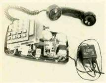
INSIDE VIEW of the Superphone 7710. The buzzer is used as an alarm signal. Rechargeable batteries retain memory if the power fails.
