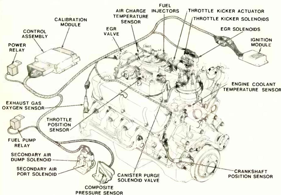
**ELECTRONIC COMPONENTS** of the new Ford V-8 engine used in the 1980 Lincoln Continental and Mark VI. No less than six of these are sensors of the various engine conditions, information from which is used to control the electronic fuel injection and other functions to limit emissions while promoting fuel economy. Electronic components are also used to control the entertainment apparatus, remote-control the CB equipment, and even to open the doors.
