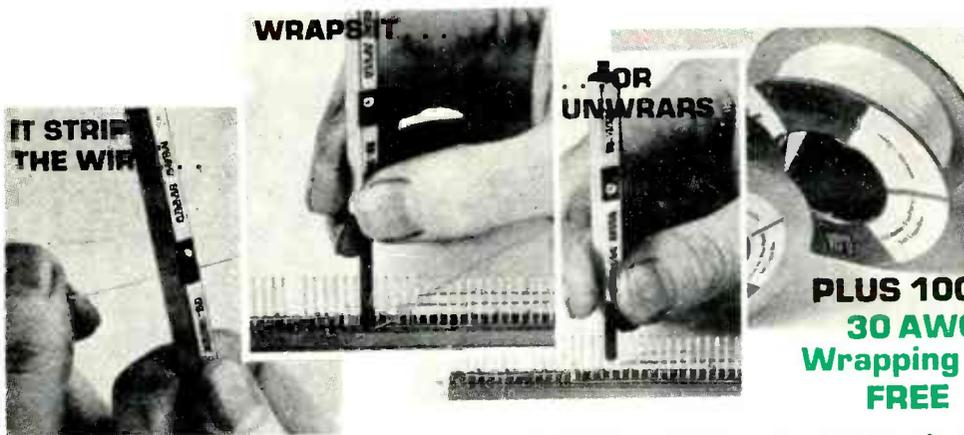
Perfect for the engineer, experimenter, or serious amateur who needs a high quality tool for detailed wiring projects. This versatile tool strips the wire, then wraps it around the stake or unwraps existing connections. PLUS—for a limited time only we'll include, at no extra cost, a free roll of our best wrapping wire.
