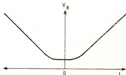
FIG. 9—LOGARITHMIC COMPRESSION-BIAS circuit varies the bias voltage of the output stage in accordance with the output current.
