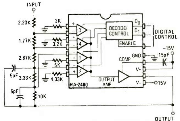
**AMPLIFIER, INVERTING WITH PROGRAMMABLE GAIN**
