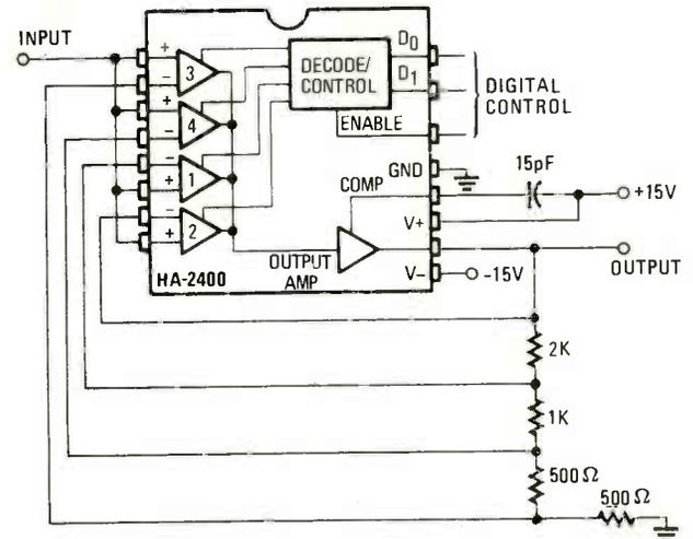
**AMPLIFIER, NON-INVERTING WITH PROGRAMMABLE GAIN**
