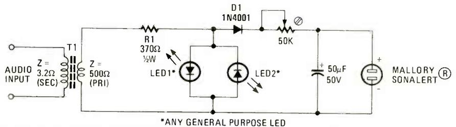
**FIG. 1—THUNDERSTORM ACTIVITY indicator and alarm.** The audio input terminals are connected to the speaker terminals of any AM broadcast radio receiver.
