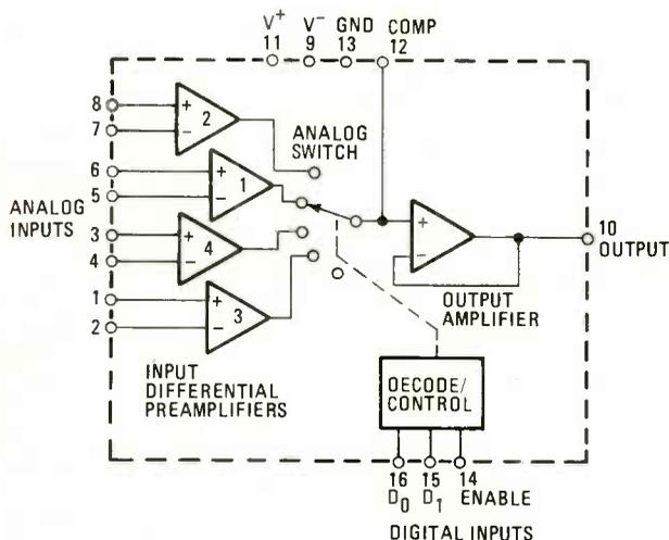
In actuality, the circuit consists of four conventional op-amp input circuits connected in parallel to a conventional op-amp output circuit. The decode/control circuitry furnishes operating current only to the selected input section.
