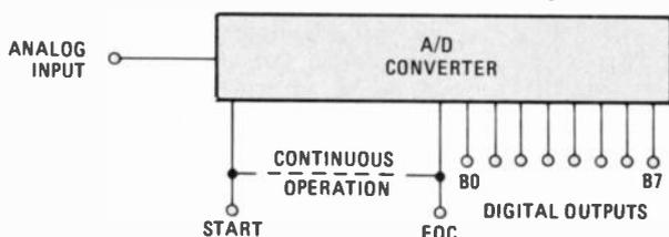
FIG. 1—TYPICAL A/D CONVERTER provides 8-bit digital representation of analog input signal. Start and EOC lines control the converter's operation.
