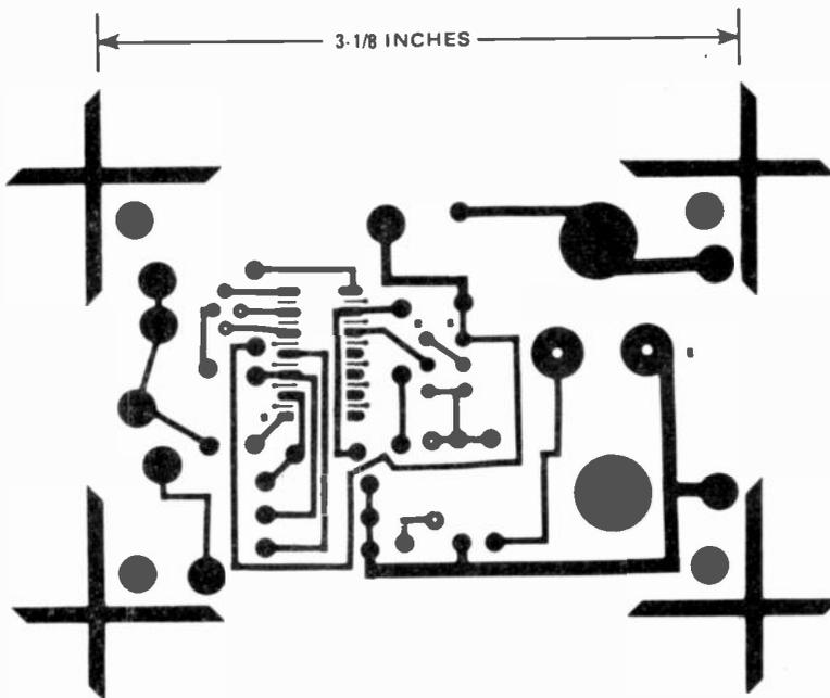
FIG. 4—FOIL PATTERN for the regulator printed circuit. The finished board measures 3-1/8 by 2-1/16 inches.
