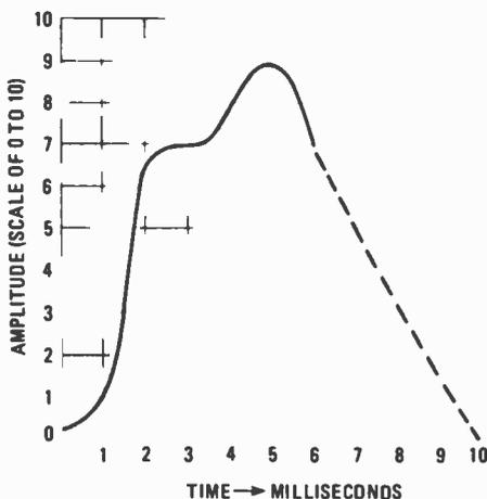
FIG. 2—DIGITAL CONVERSION of analog signal requires sampling the amplitude of the analog signal at discrete time intervals.
