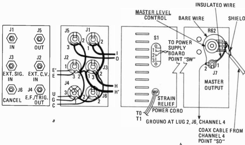
FIG. 10—HOW COMPONENTS ARE MOUNTED on the rear panel. Drawings at a show the jacks: how they are positioned and connected to coded points on the circuit board. Four sets of jacks are used—one set of six for each synthesizer module. The drawings at b show components on the ends of the rear panel.
