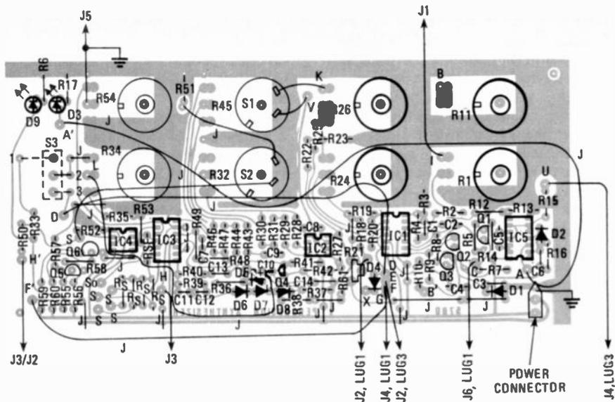
FIG. 6—HOW PARTS ARE POSITIONED on the synthesizer modules. The four  $R_2$  resistors are installed only on the module for the fourth channel. The diagram also shows jumpers and connections to off-board components.
