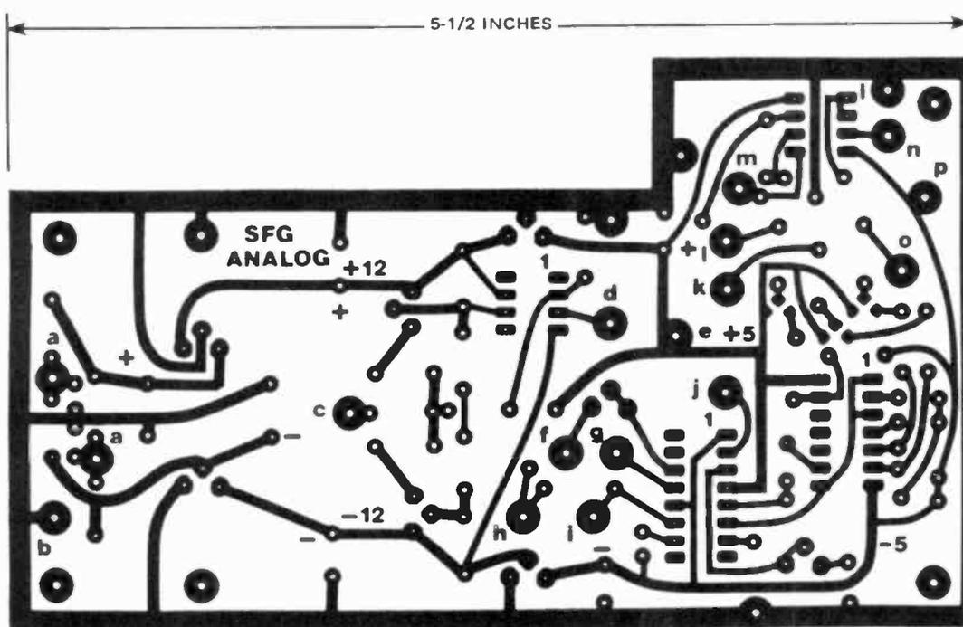
FIG. 3—FOIL PATTERN for the analog circuit board.
