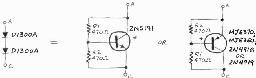
\* BE SURE TO MOUNT USING MICA INSULATING WASHER
