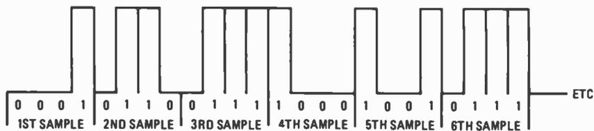
FIG. 4—PCM FORMAT is recorded on magnetic tape as the presence or absence of pulses. The PCM format shown divides each sample into a 4-bit digital word.
