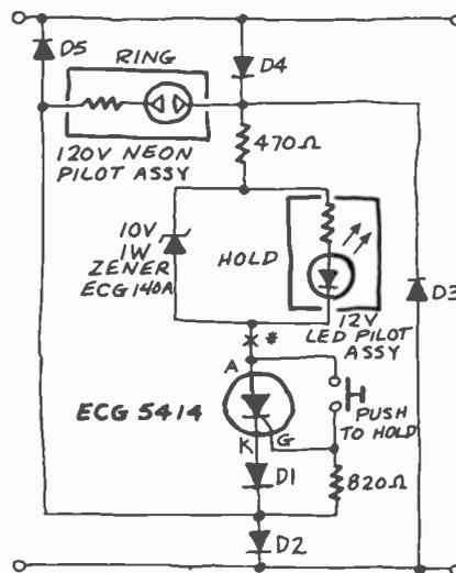
\* BREAK HERE TO INSERT TRANSFORMER WINDING. D1-D5 SWITCHING DIODES; 1 AMP, 600 PIV, SILICON
