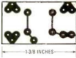
FIG 43—WHEN YOU MAKE THIS BOARD, be sure that pads *do not touch* rectangular border.
