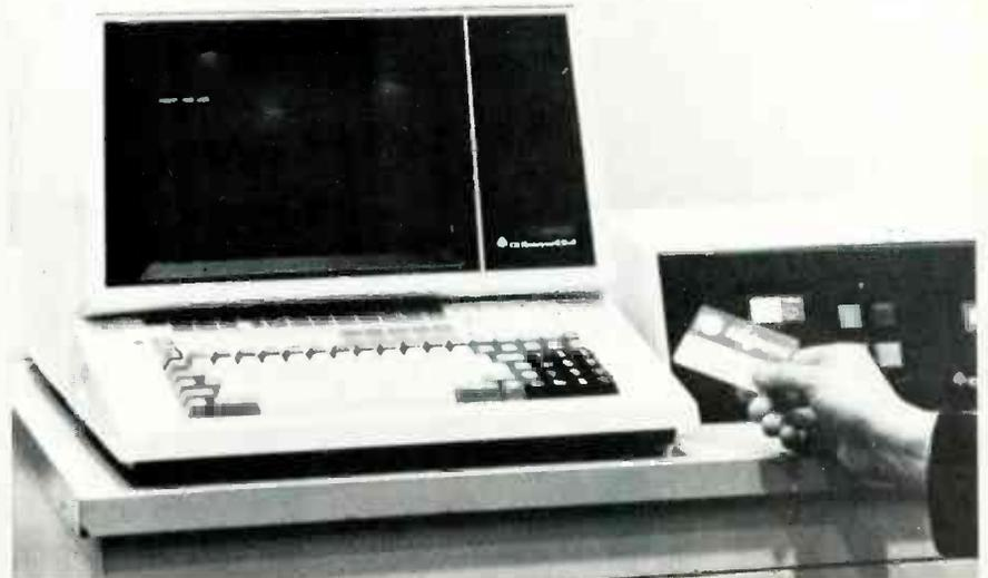
INSERTING THE SMART CARD in the reader to the right of the display terminal shows the cardholder his bank balance. It also supplies any other information for which the system may be programmed, or may transfer funds according to his instructions.
