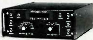
THE INFO-TECH model M200-F video converter does not require a terminal unit.
