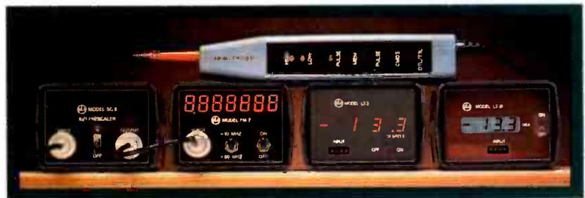
Operator convenience is the key to our line of frequency and temperature meters, too. Pictured left to right, SC-5 prescaler, FM-7 frequency meter, LED format LT-3 digital temp meter, and its LCD cousin, the LT-31. Top, the MLB-1 digital logic probe.
