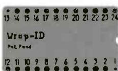
Slipped onto socket before wrapping to identify pins.
