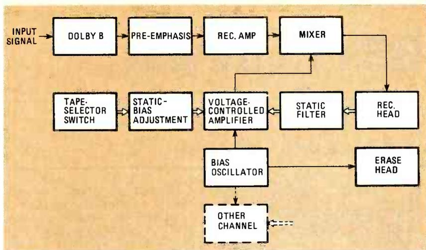
FIG. 5—BLOCK DIAGRAM of the *Dolby HX Professional* system. Unlike *Dolby HX*, this system measures the sum of the audio signal, including any preprocessing, and the bias at the record head.
