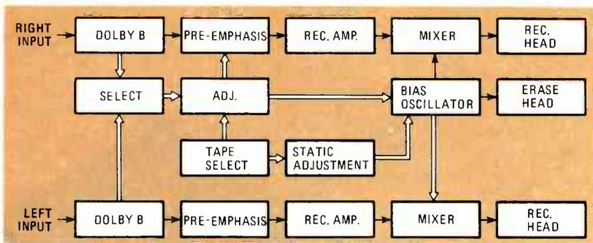
FIG. 2—THE ORIGINAL DOLBY HX system is shown in this block diagram. For the system to work, a control signal that is sensitive to amplitude and frequency content is required.
