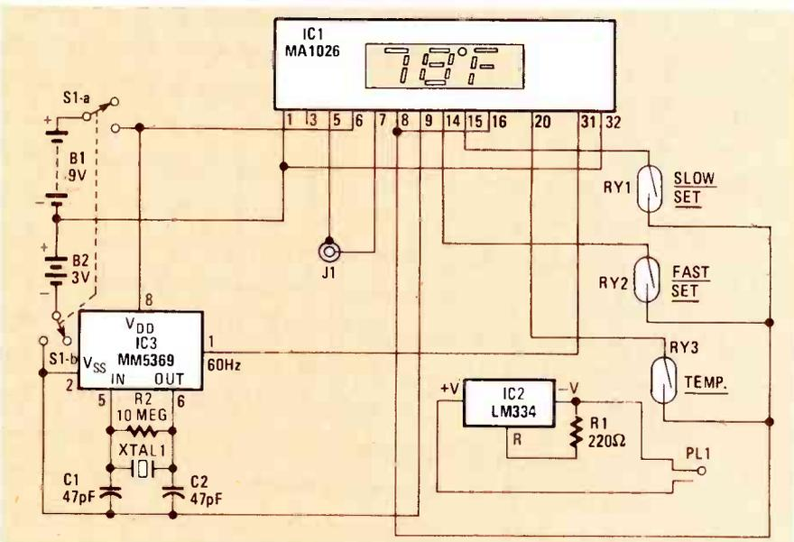
FIG. 3—FOR PORTABLE OPERATION, build this version of the clock/thermometer project. The oscillator circuit draws just 1.5 milliamperes.
