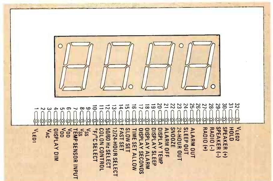
FIG. 1—THE COMPLETE PIN-OUT for the National MA1026 clock module is shown here.
