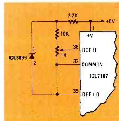
FIG. 9—USED HERE in an A/D converter circuit, the ICL8069 is well suited for such an application.
