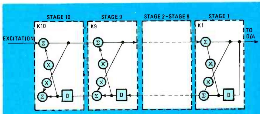
FIG. 5—TEN-STAGE LATTICE FILTER used in Texas Instruments' linear-predictive-coding synthesizer simulates the resonant effects of the mouth and nasal cavities.
