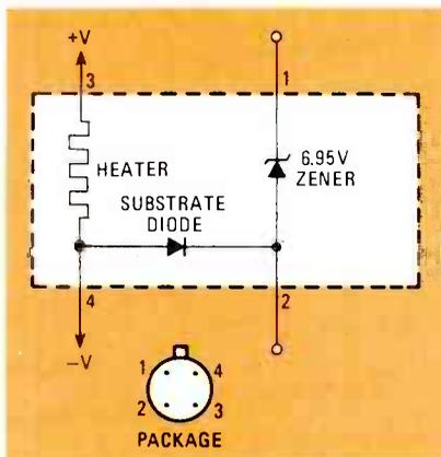
FIG. 5—A ZENER DIODE and an on-chip heater element are combined in the LM-199. The resulting IC is a highly stable voltage-reference device.
