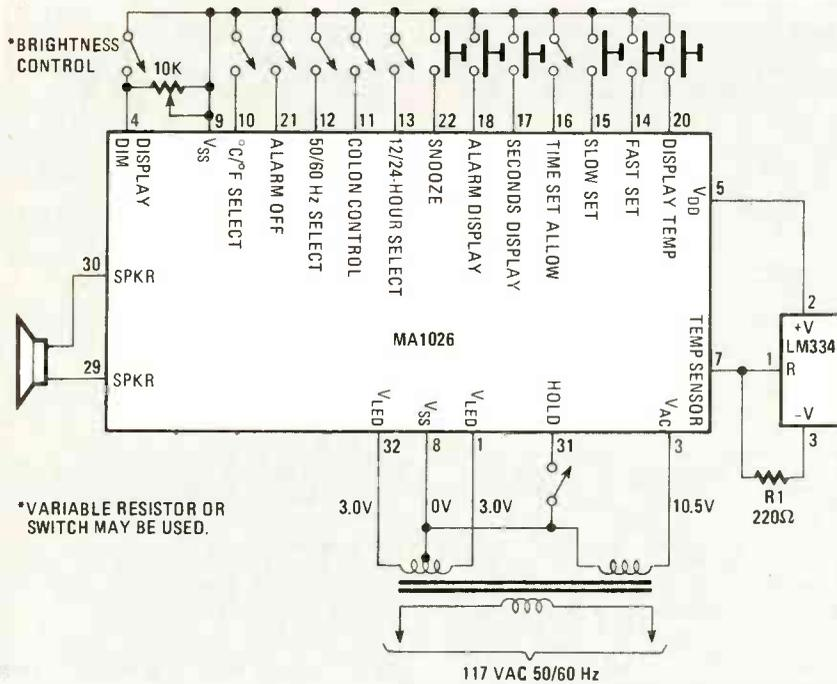
FIG. 5—EXPAND THE BASIC CLOCK/THERMOMETER project and make a full-function alarm clock with snooze alarm, using this circuit.
