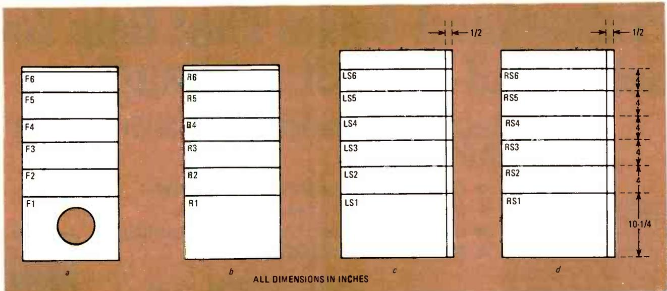
FIG. 8—PARTITION MOUNTING STRIPS for the front are shown in (a), rear are shown in (b), left side are shown in (c) and right side are shown in (d).
