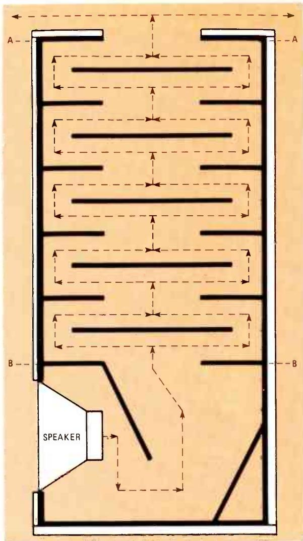
FIG. 1—SIDE VIEW OF SAFE ENCLOSURE showing speaker back-wave path. Path is symmetrical between points A and B.
