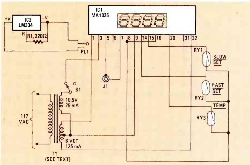
FIG. 2—SCHEMATIC DIAGRAM of the digital clock/thermometer and the temperature sensor. To make the temperature sensor, mount IC2 and R1 on a small piece of perforated construction board.
