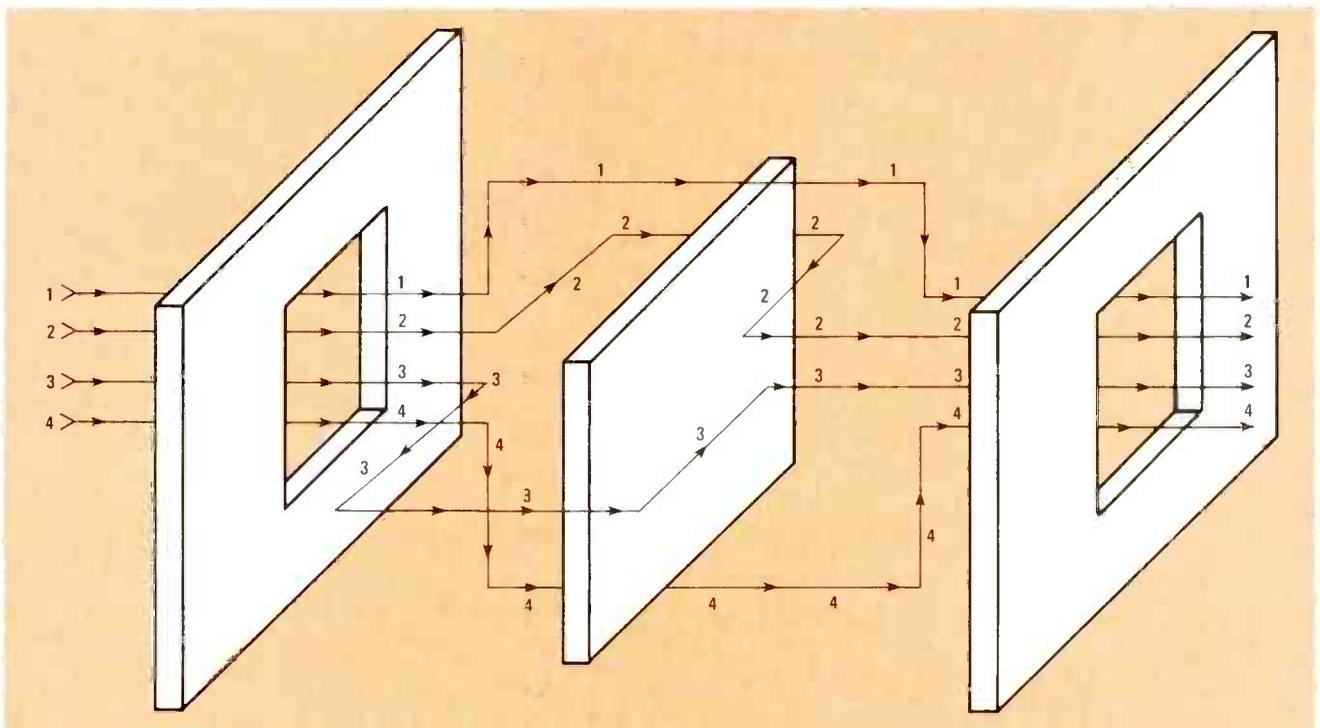
FIG. 2—SPEAKER BACK-WAVE is alternately combined and separated as it passes through and around SAFE enclosure's baffles.
