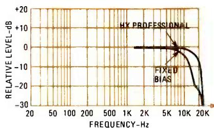
FIG. 6—HIGH-FREQUENCY CAPABILITIES of a cassette recorder equipped with *Dolby HX Professional* versus a conventional machine of the same quality.
