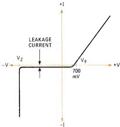
FIG. 2—WHEN THE REVERSE BIAS exceeds  $V_Z$  the negative current through the Zener increases rapidly.
