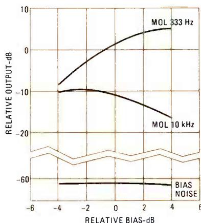
FIG. 1—THE BIAS LEVEL that provides the highest output with acceptably low distortion for a 333-Hz tone is quite different than the bias level required by a 10-kHz tone.
