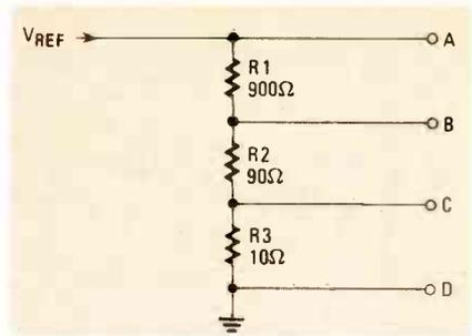
FIG. 11—A RESISTOR NETWORK can be used to get a multiple-output voltage reference. The voltage at each tap is 10 times higher than the voltage at the tap below it.
