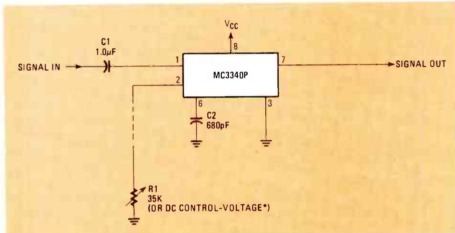
\*ATTENUATION PROPORTIONAL TO VOLTAGE AT PIN 2 WHEN 3.5VDC <math>V\_C</math> <math>6.0</math> VDC, OR PROPORTIONAL TO RESISTANCE FROM 0 TO 33K OHMS
