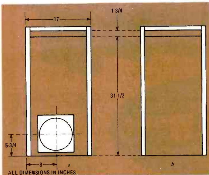
FIG. 9—SPEAKER SHOULD BE MOUNTED slightly off-center to prevent standing waves. Center figure shows distance between partition 1 and top of enclosure.
