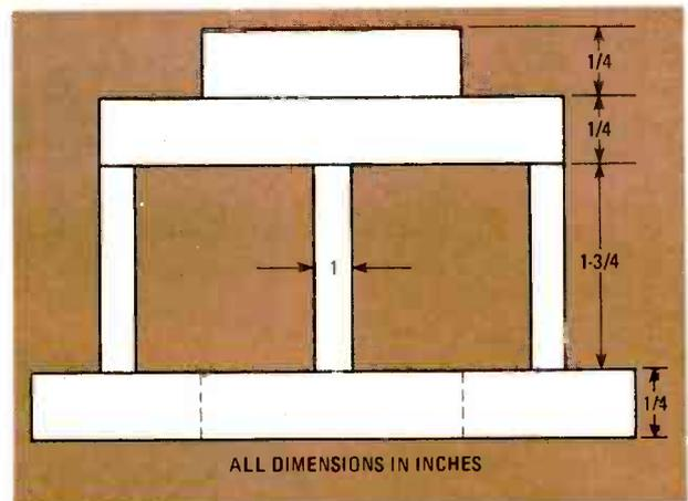
FIG. 11—SIDE VIEW of even-numbered partition mounted atop odd-numbered partition using partition mounting strips. Each strip is located as shown in Fig. 10 and measures 1 x 1 x 1/4 inches.
