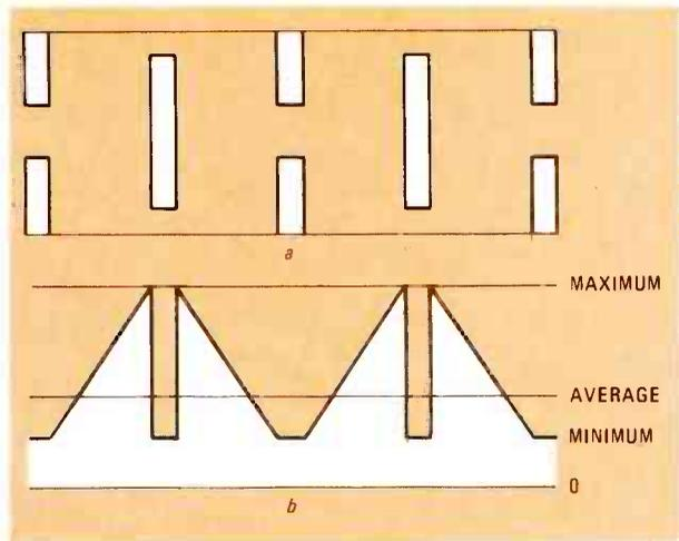
FIG. 3—PARTITIONS USED IN SAFE ENCLOSURE (a) affect its effective cross-sectional area (b).
