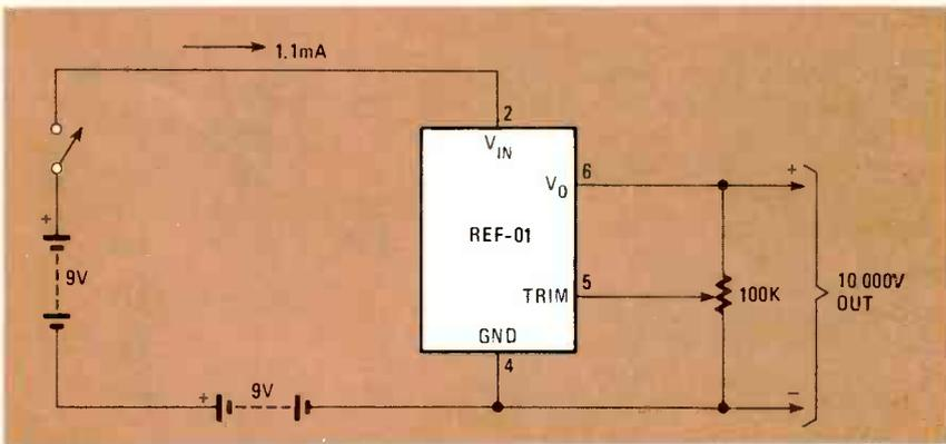
FIG. 10—A SIMPLE POTENTIOMETER is used to trim the output of the PMI REF-01 voltage reference to exactly 10.00 volts.
