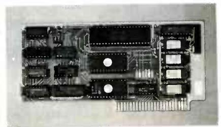
**The Microbuffer II** is an intelligent buffered parallel printer interface for the Apple II computer. Includes 16K of on-board RAM. Buffer memory size is user expandable to 32K. Compatible with Applesoft, CP/M, and Pascal. Includes advanced high resolution graphics print routines for the Epson MX-80 with Graphtrax, Anadex, IDS Paper Tiger, NEC Prowriter. Price: \$259. Contact Practical Peripherals, Inc., 31245 La Baya Dr., Westlake Village, Calif. 91362 (213) 706-0339.
