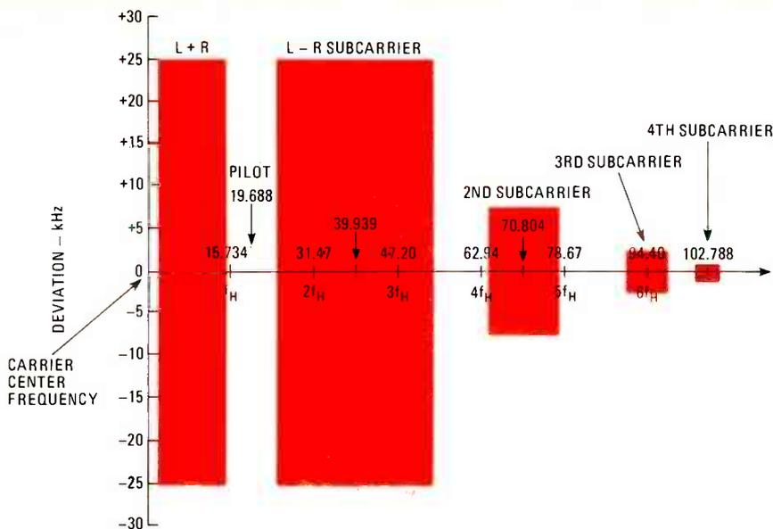
FIG. 3—TELESONICS SYSTEM uses amplitude modulation for its subcarriers. The scheme allows as many as four subcarriers.
