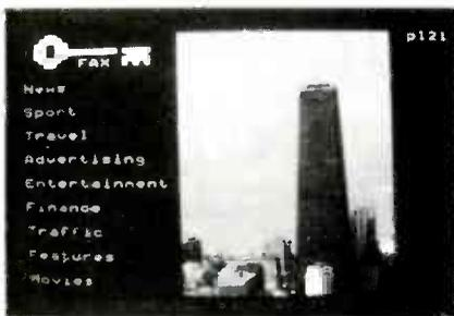
FIG. 17—THE ALPHA-PHOTOGRAPHIC mode allows photographs to be included as part of the videotex material. The picture shown took about two seconds to transmit.
