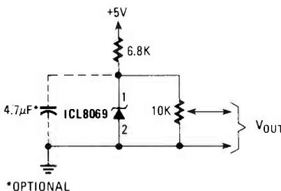
FIG. 7—A 1.2-VOLT temperature-compensated voltage reference, the Intersil ICL8079 used in this circuit is well suited to high-speed A/D and D/A converter projects.
