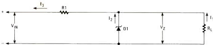
FIG. 1—THE ZENER DIODE is often used as a voltage reference or as a simple voltage regulator. A basic circuit for a Zener diode regulator is shown here.
