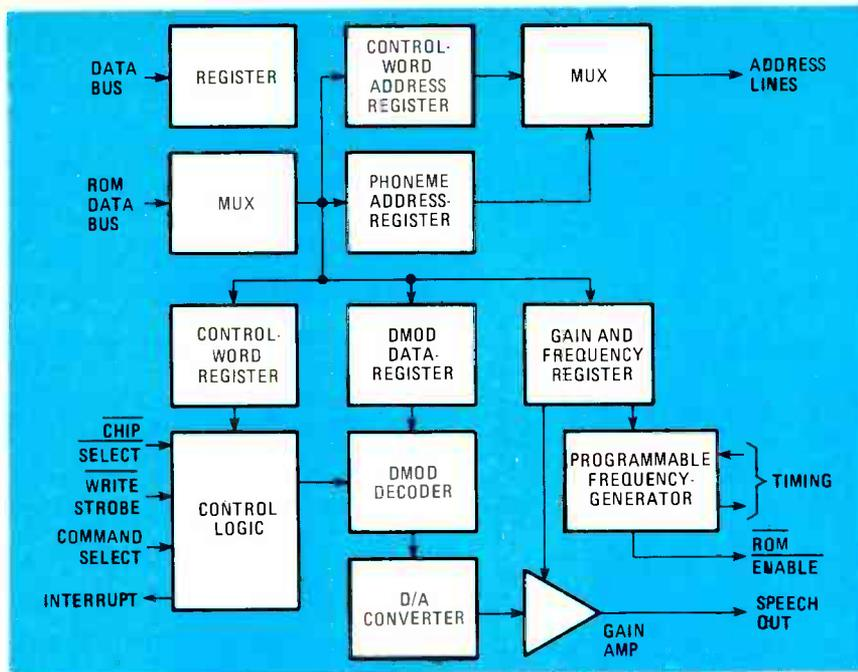
FIG. 2—NATIONAL SEMICONDUCTOR'S DIGITALKER has a fixed vocabulary in ROM; several different ROM's are available. Programmable frequency-generator (lower right) is used to add inflection to speech.
