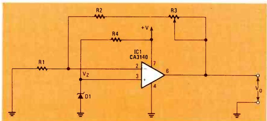
FIG. 4—AN OPERATIONAL AMPLIFIER can be used to scale the voltage from the Zener diode to whatever value is needed.
