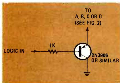
FIG. 4—THIS CIRCUIT can be used to drive a digital volume attenuator's control lines. Almost any PNP transistor can be used.
