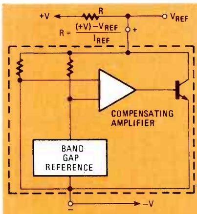
FIG. 6—THIS TWO-TERMINAL REGULATOR from Ferranti Electric can be used just like a Zener diode. It has a stability as great as 10 ppm per 1000 hours of operation.
