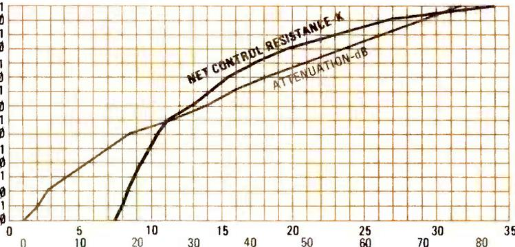
FIG. 3—NET CONTROL RESISTANCE and calculated attenuation plotted against four-bit control signals. Note that the calculated attenuation curve is nearly, but not quite, linear.
