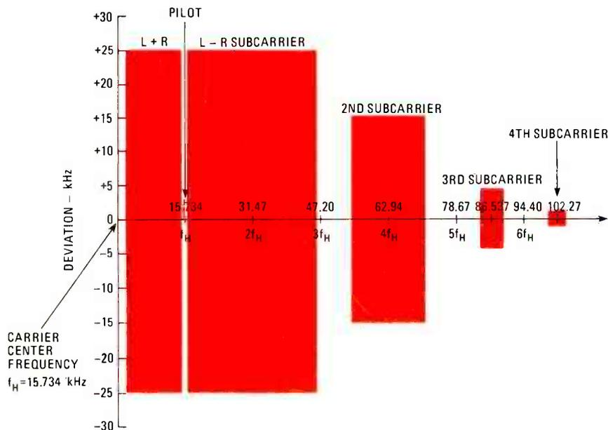
FIG. 4—ZENITH RADIO CORPORATION'S system uses the horizontal line-frequency, 15.734 kHz, for the pilot tone.
