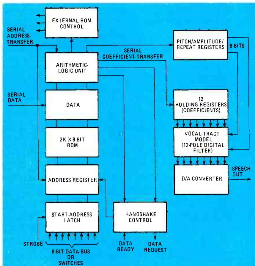
FIG. 3—A PHONEME-BASED synthesizer, such as General Instruments' SP0256, uses the sound elements that make up words to provide an almost unlimited vocabulary.
