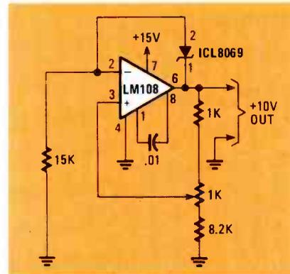
FIG. 8—A ICL8069 IS PLACED in the feedback loop of an LM108 op-amp in this voltage reference circuit. The potentiometer is used to trim the output to exactly 10.00 volts.
