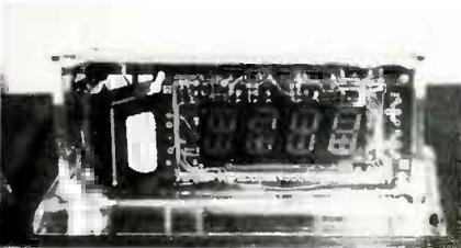
FIG. 4—THIS IS HOW the project will look when it is finished. The clear case—an acrylic butter dish—makes the clock more interesting visually.
