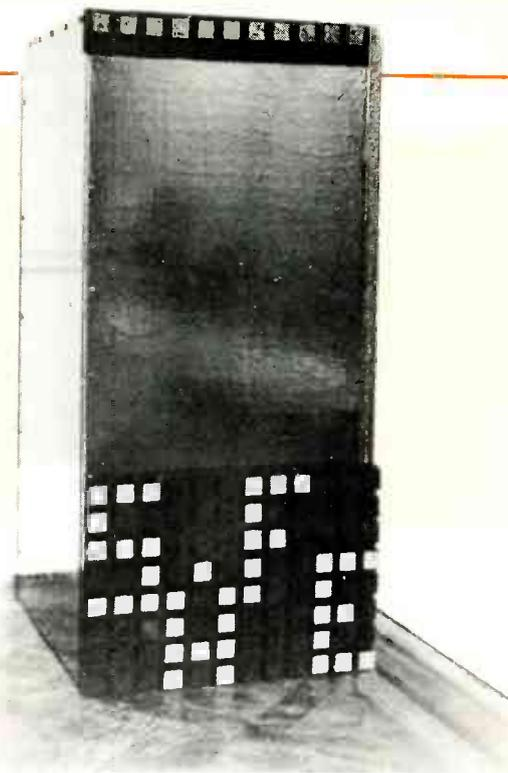
IN THE DECEMBER 1981 ISSUE, **RADIO-ELECTRONICS** PUBLISHED plans for constructing a speaker that used the SAFE (Symmetrical Air Friction Enclosure) principle (U.S. patent no. 4,168,761, other patents pending) to obtain good sound from a small enclosure. This article deal with a companion subwoofer using the SAFE principle that provides extended bass response from a relatively small enclosure.
