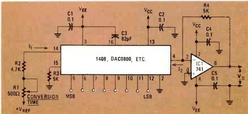
FIG. 12—A DIGITALLY SELECTABLE voltage reference. Once the input current ( $I_1$ ) to the D/A converter is set, the output from the circuit ( $V_O$ ) is determined by digital input (pins 5-12) to the D/A converter.
