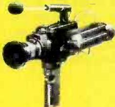
Video cameras have entered the all-solid-state age in the United States with the start of marketing of Hitachi's MOS camera, which uses a single  $\frac{2}{3}$ -inch metal oxide silicon IC as an image sensor. The MOS sensor has 180,000 picture elements, providing a claimed 260-line horizontal resolution. The camera weighs 3.96 pounds.
