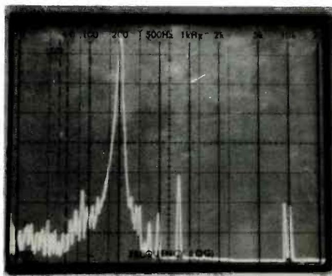
FIG. 4—MUTUAL BIASING is demonstrated here. Two low-level, higher-frequency (9 and 10 kHz) tones were mixed with the 300-Hz tone.
