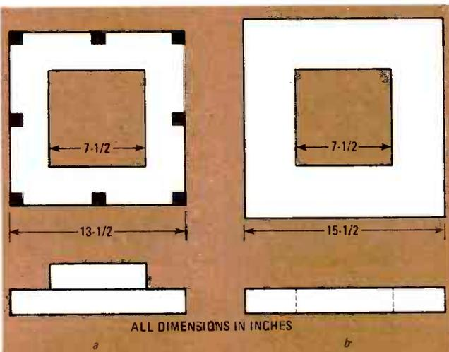
FIG. 10—EVEN-NUMBERED PARTITIONS (a) have "top hat" structure caused by using center piece cut out of odd-numbered partitions.
