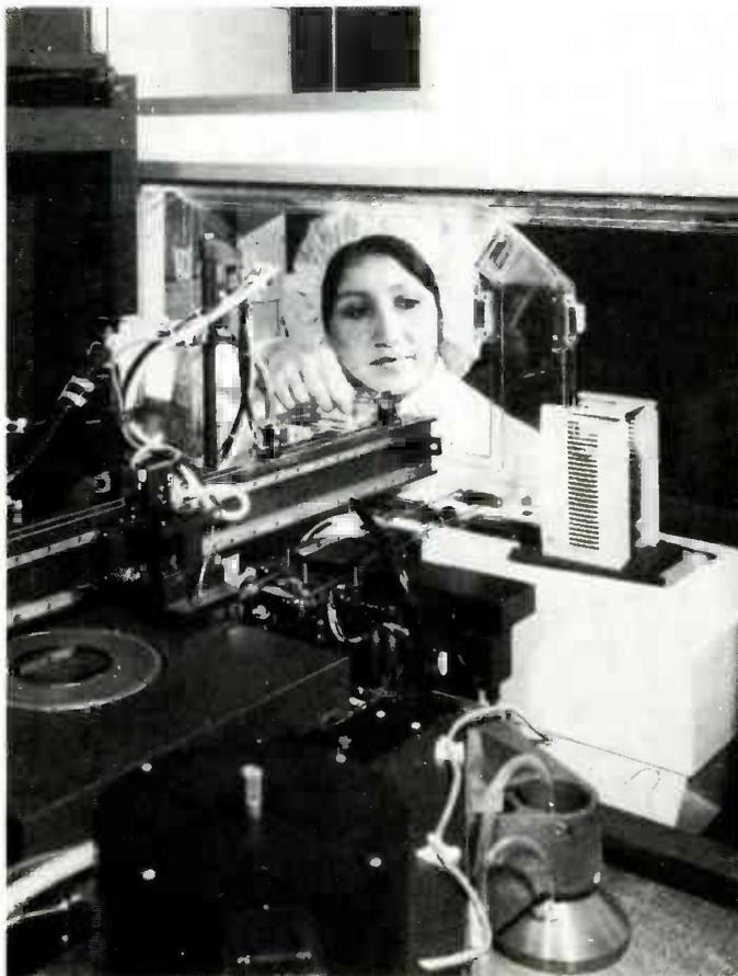
PHOTO-LITHOGRAPHY MACHINE that will be used to etch VHSIC circuits on chips the size of a thumbtack. Hughes and five other firms are in the program conducted by the Defense Department to develop the high-speed superchips. The machine is being operated by Hughes technician Margaret Sanchez.
