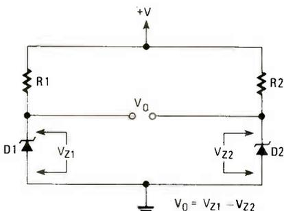
FIG. 3—THIS CIRCUIT shows one way to overcome the problem of temperature drift in Zener diodes.
