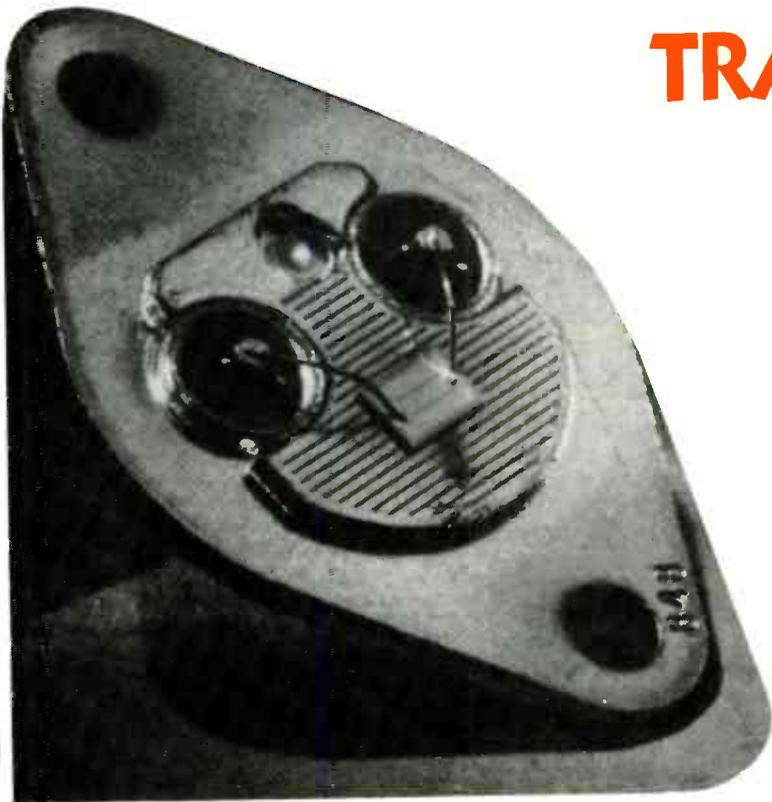
*This month, we turn our attention to a slightly more complex solid-state component—the transistor. We'll begin by looking at the structure and operation of both bipolar and FET devices.*
