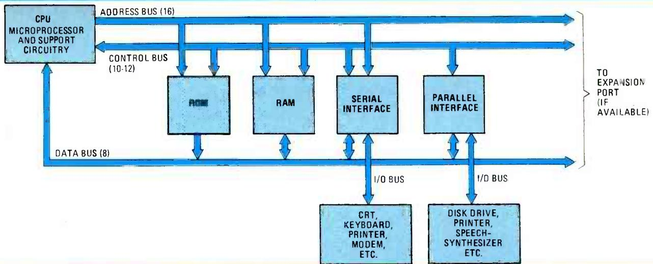
FIG. 1—BLOCK DIAGRAM of a basic microcomputer system. Note the arrows on the bus lines. They indicate the direction of information flow.
