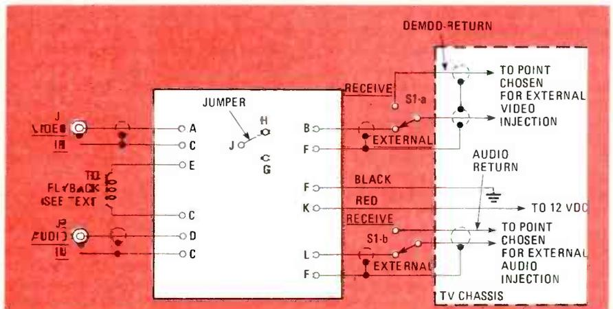
FIG. 8—WIRING DIAGRAM shows jumper wired for positive video.
