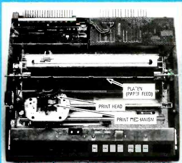
FIG. 1—THE MAIN PARTS OF A PRINTER are the print head, the print mechanism, the platen, and the paper-feed mechanism.
