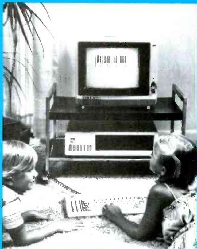
FIG. 4—THE IBM PERSONAL COMPUTER is a component-type system that can use a standard TV for display.
