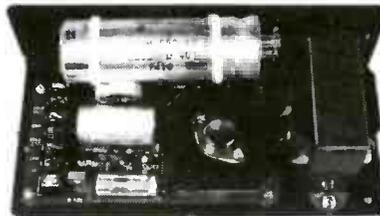
The JE224 is a high-efficiency power supply utilizing a LH1605 5 amp switching regulator. The LH1605 provides high current output while maintaining a small physical configuration. Open frame type to allow mounting into restricted areas.
