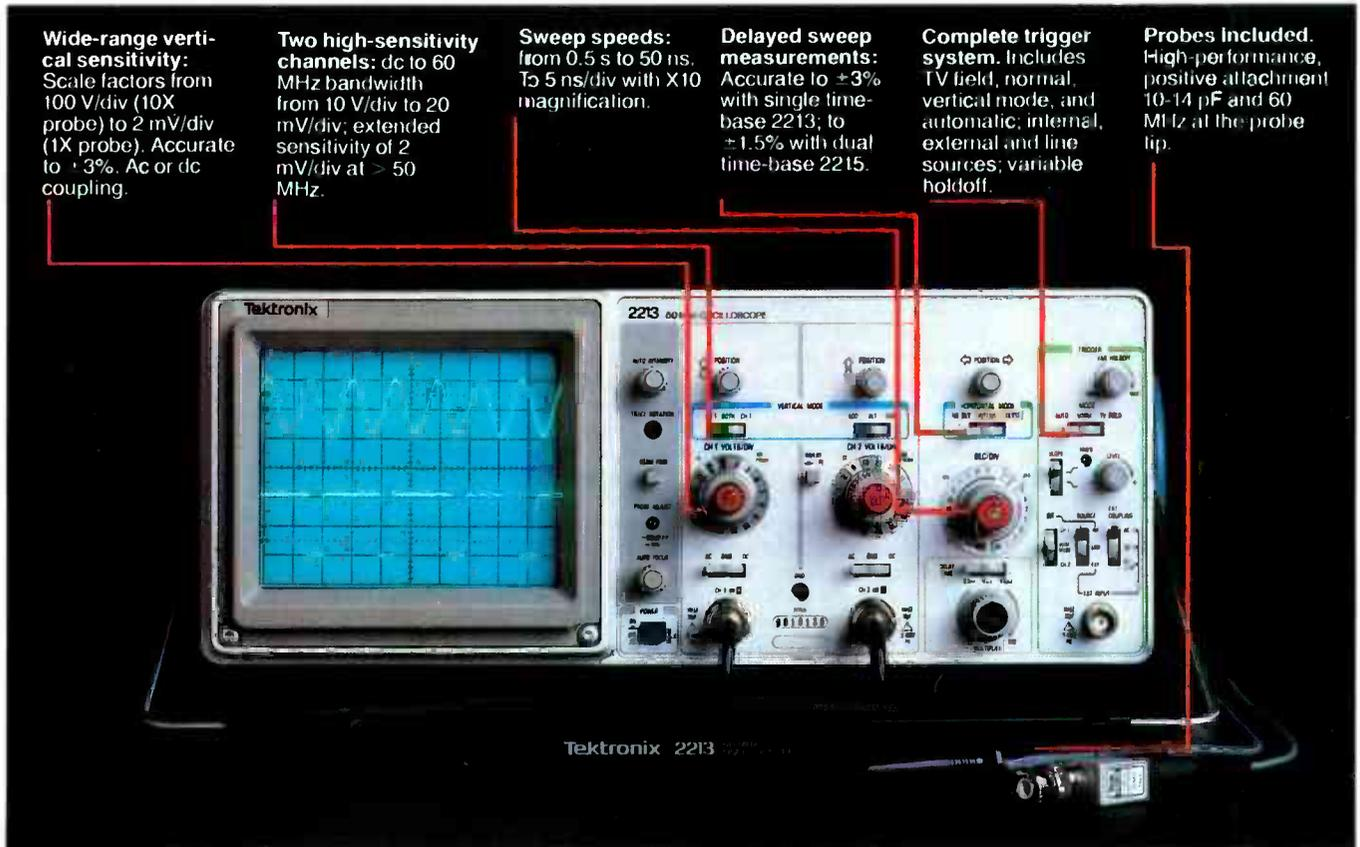
**Wide-range vertical sensitivity:** Scale factors from 100 V/div (10X probe) to 2 mV/div (1X probe). Accurate to  $\pm 3\%$ . Ac or dc coupling.
