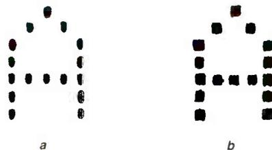
FIG. 2—DOT-MATRIX CHARACTERS (a) are formed by an array of pins that press against the ribbon to form an image; print offsetting can provide a much higher quality output (b).
