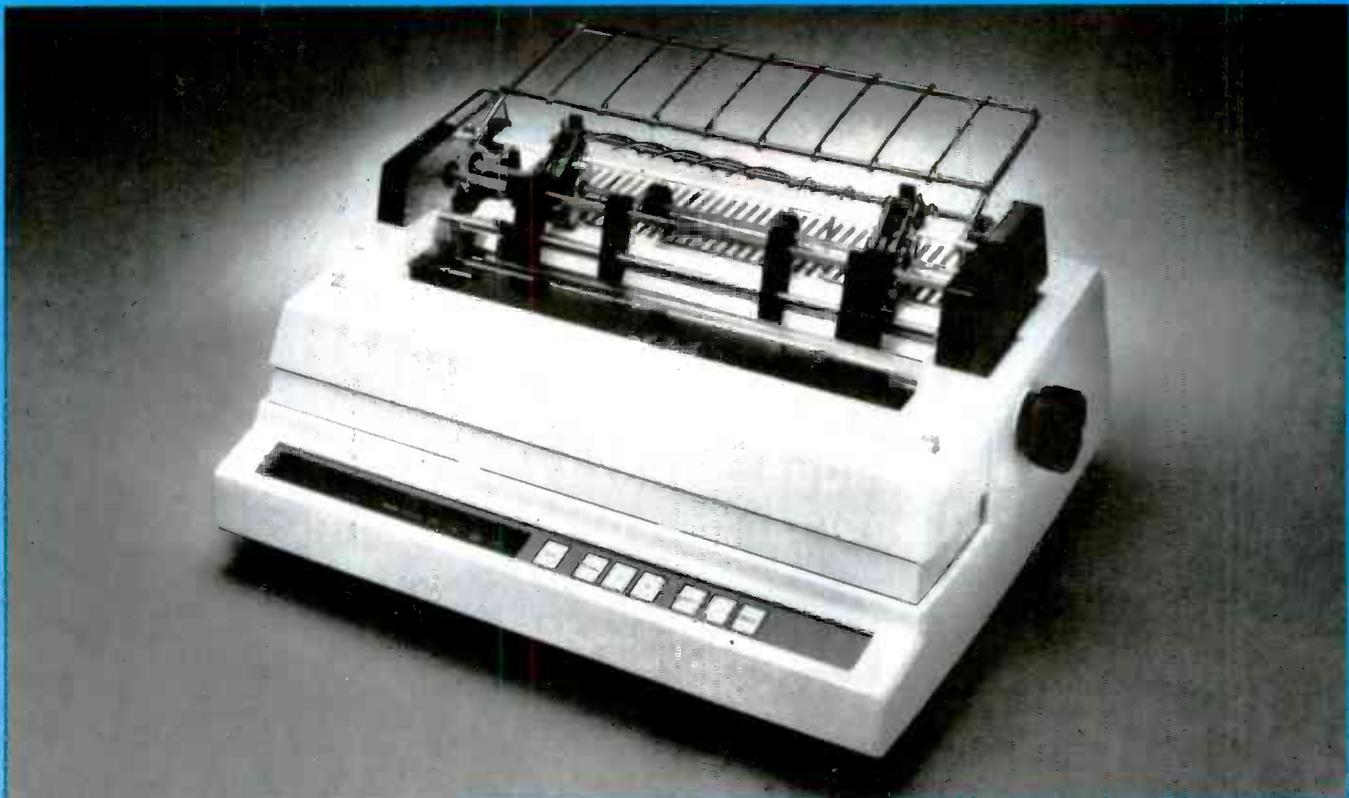
FIG. 6—A TRACTOR-FEED MECHANISM allows continuous-form paper to be pulled through the printer evenly without slipping from side to side. Thus, it allows long unattended runs.
