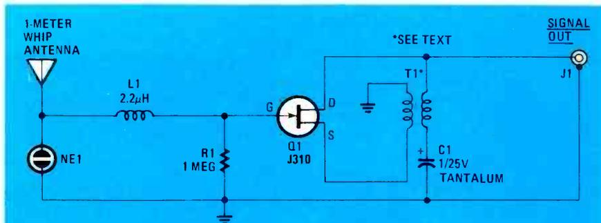
FIG. 1—WIDEBAND PREAMPLIFIER SCHEMATIC. The neon bulb, NE1, provides adequate input static charge protection.
