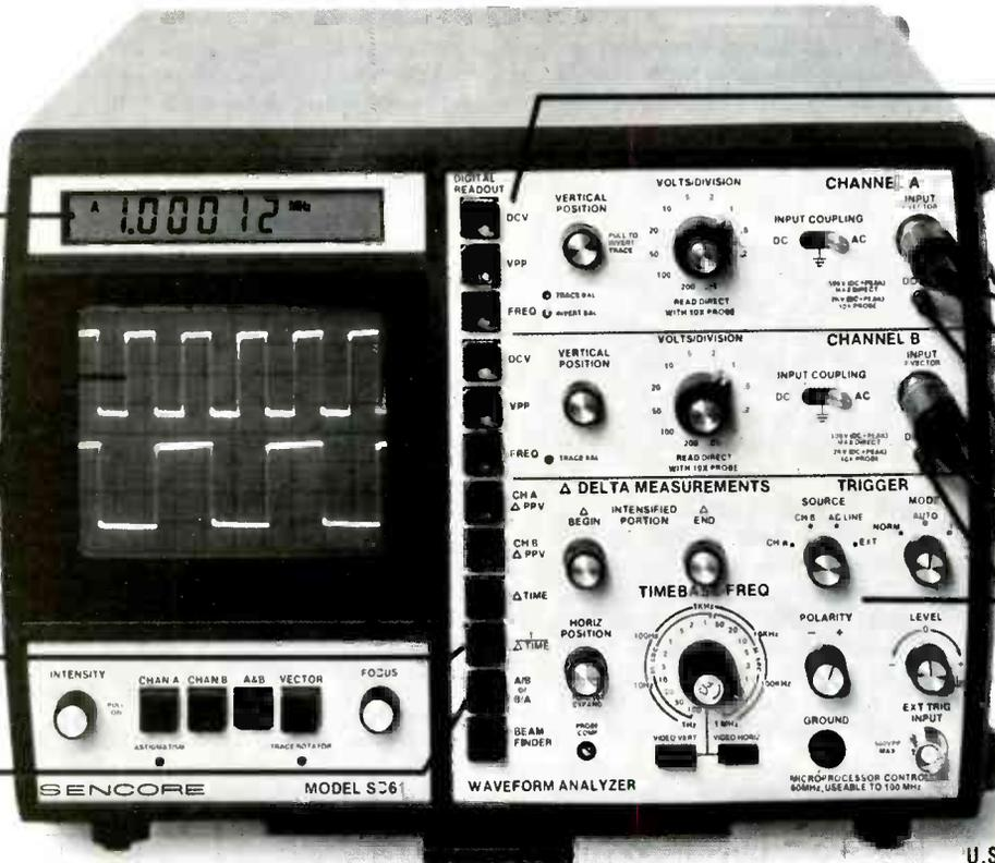
**Autotracking DCV, PPV, Freq:** Measure DCV to .5%; PPV to 2%; freq. to .001%. Just push a button for either Channel A or B.
