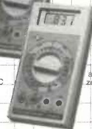
Circuitmate DM 45—3 1/2-digit multimeter; 0.5% Vdc accuracy, diode test, continuity beeper, 10 amps AC and DC ranges, auto-polarity, auto-zero, auto-decimal
