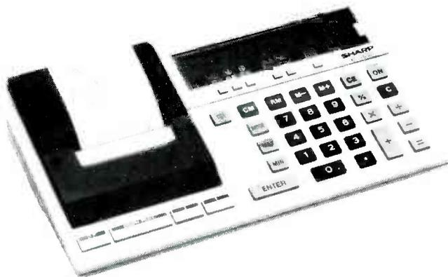
**THIS SHARP EL-7050** calculator can generate a variety of graphs and print them out in an array of colors.
