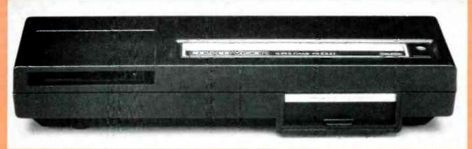
COLECO'S SUPER GAME MODULE on Expension Module #3) uses water tapes instead of cartridges.
