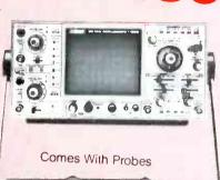
• 100 MHz response, 3.5nS rise time • 2nS/div. sweep rate with 10X magnifier • Trigger views or four separate inputs ● Dual time base ● 1 M ohm inputs or 50 ohm inputs • 1mV/div sensitivity to 100 mHz • CH 1 frequency counter output • Delayed sweep, 20 nS to 0.5 seconds • Alternate timebase Switching power supply
