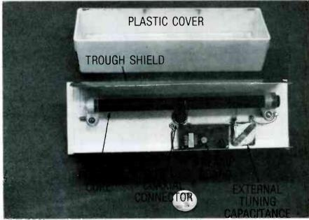
FIG. 8—AN ACTIVE ferrite-core loop antenna in its trough shield.
