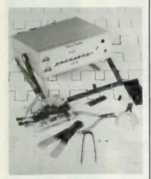
8 Channel Logic Analyzer To Be Used With Your Scope As The Display Media
