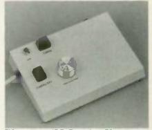
FIG. 5—TO MAKE THEM EASIER TO FIND in the dark, cluster the unit's operating controls around NE1.
