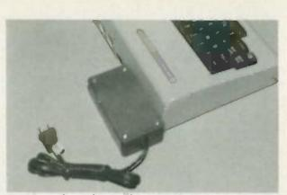
FIG. 11—THIS ILLUSTRATES the power controller connected to the computer. Be sure the connector location is such that the box does not cover the opening for the cassette interface.
