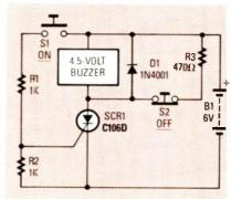
FIG. 7—ADDING A RESISTOR (R3) to the previous circuit allows you it to latch on. Turn it off by pressing \$2.
