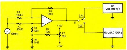
FIG. 6—TO MEASURE CMRR, use this test setup. With the 1000-Hz source off, adjust R7 for zero volts DC. Next, apply the test signal and measure the output with the oscilloscope. Last, calculate CMRR as discussed in the text.
