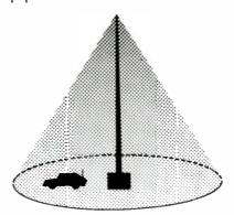
FIG. 1—EAFLY, NON-CELLULAR, MOBILEphone systems used a centrally located highpower transmitter. Only a few communications channels could be accommodated within a service region.
