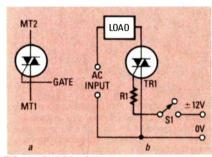
FIG. 12—THE TRIAC'S symbol (a) and basic control circuit (b) are shown here.
