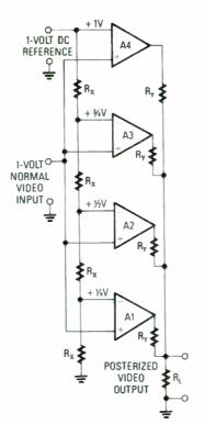
FIG. 6—AN ELEMENTARY POSTERIZER circuit. The value of the DC reference voltage determines the width of each step.
