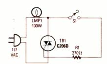
FIG. 15—SIMPLEST TRIAC CIRCUIT is composed of a switch, a resistor, and a Triac.
