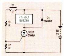
FIG. 6—A BUZZER (or other self-interrupting device) can be used to build an SCR power controller that remains on only so long as S1 is pressed.
