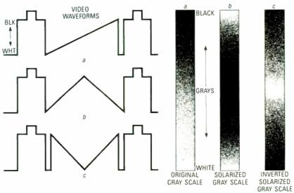
FIG. 7—SOLARIZATION FOLDS THE SIGNAL back on itself so that white remains white, gray becomes black, and black becomes white, or vice versa. The original signal is shown in a. The solarizied signal is shown in b. An inverted solarized signal is shown in c. The original waveform for each condition is shown in d.
