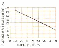
FIG. 4—INPUT BIAS CURRENT is a function of temperature.
