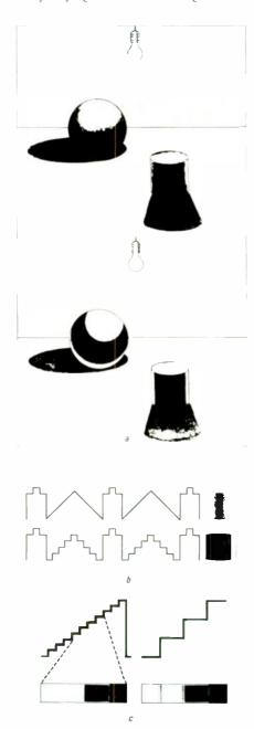
FIG. 5—POSTERIZATION CHANGES GRADUAL shading to discrete transitions (a). In b we see how the normal video signal, which originally represented increasing and decreasing ramps, is changed to a stairstep. In c we see how posterization creates grain at each transition. The grain isn't necessarily a problem because it's often used as a special video effect.
