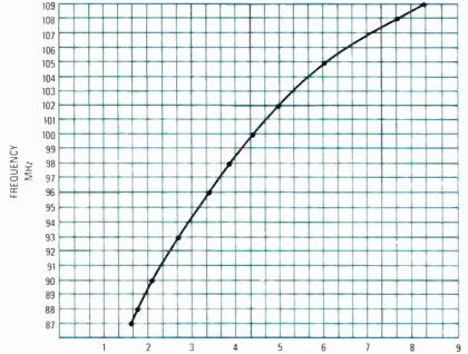
FIG. 5—USE THIS CHART to find the tuning voltage for the frequency of interest. Then adjust the setting of R71 so that voltage appears at the junction of R16 and R17 and tweak C17 until the station is received.
