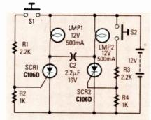
FIG. 5—A BISTABLE LATCH (or flip-flop) can be built from two SCR's.
