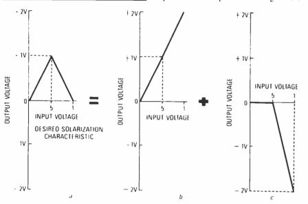
FIG.8—THE DESIRED AMPLIFIER characteristic needed for solarization, shown in a, can be attained by using two amplifiers having the characteristics shown in b and c. The video palette, however, accomplishes the same task using single controlled-gain amplifier.
