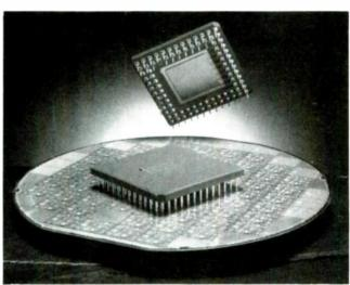
FIG. 2—INTEL'S 82786. The complexity of graphics-processor IC's requires a large number of input and output pins.
