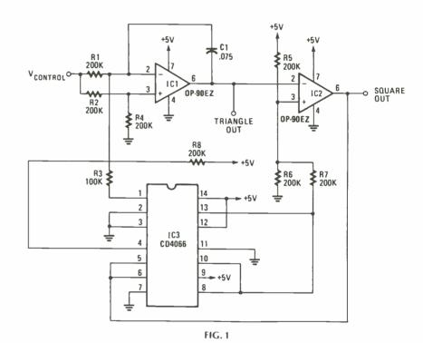
and OP-90EZ; those are hermetic 8-pin DIP's with the former operating in the military temperature range and the latter in the industrial range. Both have  $V_{OS(max)}$  of 150  $\mu V$  at 25°C available. Another version, the OP-90FZ, also in a hermetic DIP; that device operates in the industrial temperature range and has 250- $\mu V$  maximum voltage offset.
