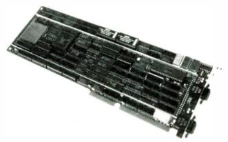
FIG. 3—NUMBER NINE COMPUTER'S SGT Pepper Graphics System uses both a TMS34010 and an 82786 in order to achieve high performance.
