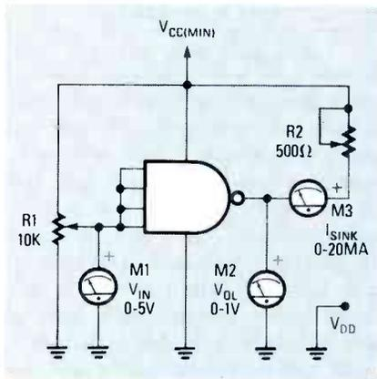
FIG. 4—THE TEST CIRCUIT used for measuring  $V_{IL}$ ,  $V_{OH}$ , and  $I_{OH}$ .
