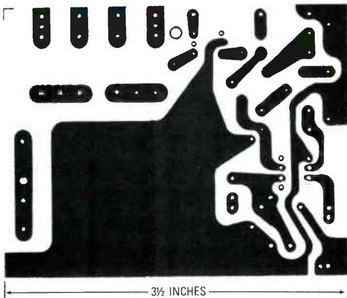
THE FOUR BOARDS on this page are used to build the Uninterruptible Power Supply. The board shown here is the power-supply board.
