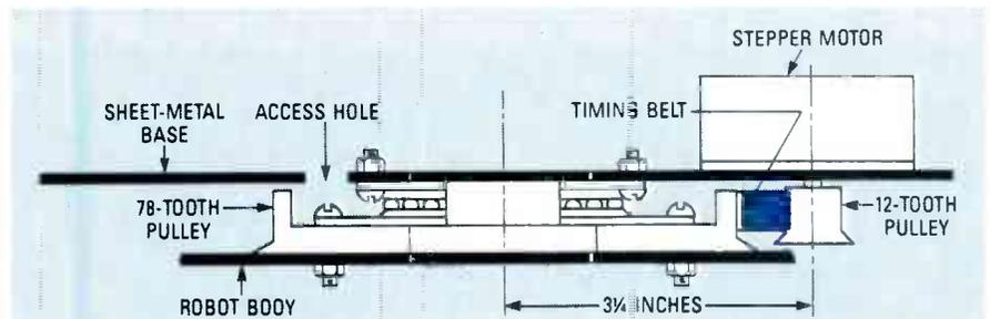
FIG. 1—THE HEAD UNIT mounts on a 78-tooth pulley. The pulley is secured to the base unit and does not rotate; instead the head rotates around it.
