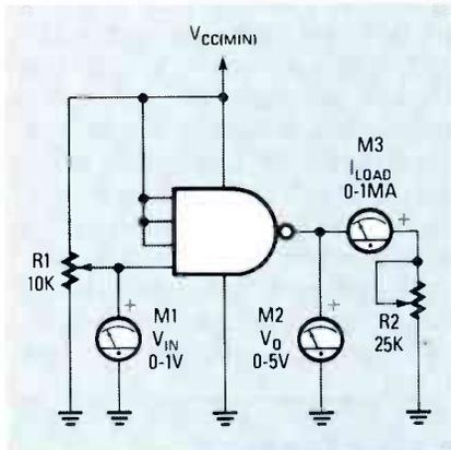
FIG. 5—THIS TEST CIRCUIT is used for measuring  $I_{IL}$ .
