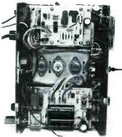
**THE AMPLIFIER OUTPUT TRANSISTORS** (one is under the function switch) are mounted on the top of a small chassis box that serves as the heatsink. The cooling fan is positioned on the cabinet cover directly over the transistors.
