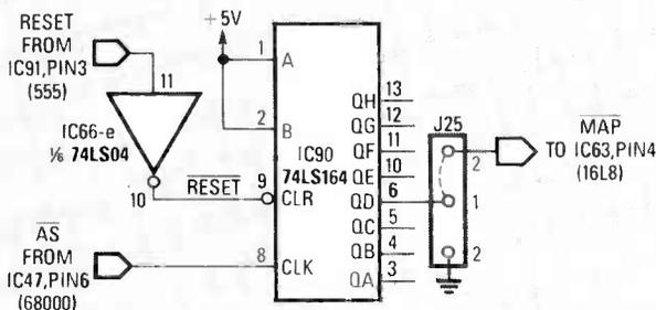
FIG. 1—THIS CIRCUIT GENERATES THE  $\overline{MAP}$  SIGNAL that forces the microprocessor to address ROM rather than RAM at power up and on subsequent resets.
