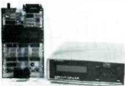
**BUILD STEVE CIARCIA'S NEW SUPER IC TESTER** Tests over six hundred 7400-series TTL, L, S, H, C, HC, HCT, F, AS, and ALS devices, 4000-series CMOS and PALs. Identifies unmarked chips and bad IC pins. User definable test sequence and user expandable ROM library. Tester operates standalone with LCD display, or with IBM PC or terminal. Partial kit—\$99. Full board kit—\$179. **CCI, 4 Park St., Suite 12, Vernon, CT 06066. (203) 875-2751.**
