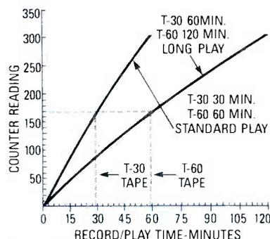
**FIG. 1—IT'S ONLY NECESSARY to calibrate the highest speed. The calibrations for a slower speed are simply a linear multiple of the highest speed.**
