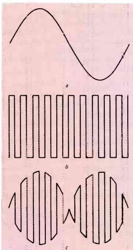
FIG. 2—HOW THE SCRAMBLER'S modulation works. If the audio signal shown in *a* is used to modulate the square-wave carrier in *b*, the resultant output is the signal shown in *c*: the original audio chopped by the carrier.
