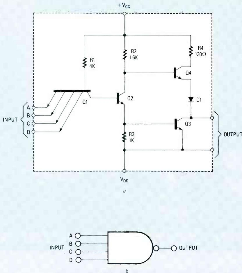
FIG. 1—THE INTERNAL STRUCTURE of a TTL 4-input NAND gate is shown in a. The equivalent logic diagram of a 4-input NAND gate is shown in b.
