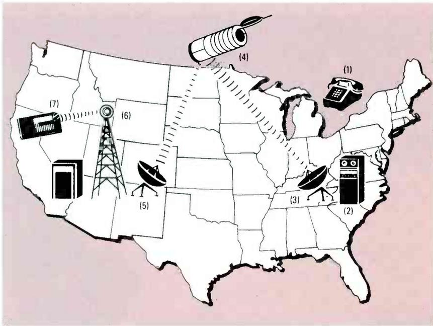
FIG. 1—NATIONAL RADIO PAGING depends on FM stations rebroadcasting the data received from a satellite.
