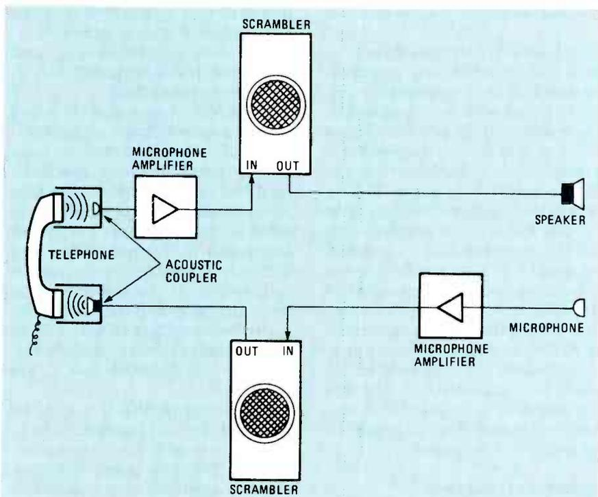
FIG. 8—TWO SEPARATE UNITS are needed in order to provide full-duplex telephone scrambling/descrambling.
