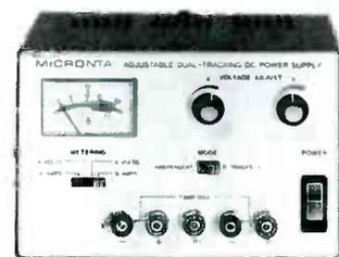
Delivers rock-steady DC that's easy to adjust to the exact voltages you need. Variable split 0-15 VDC or series up to 30 VDC. Offers choice of independent or slave operation; a single knob lets you adjust both voltages simultaneously, or use independent mode to adjust voltages separately. Switchable volt/amp meter for monitoring the voltage or current of either output. Fuse protected. UL listed AC. #22-121 ..... 69.95
