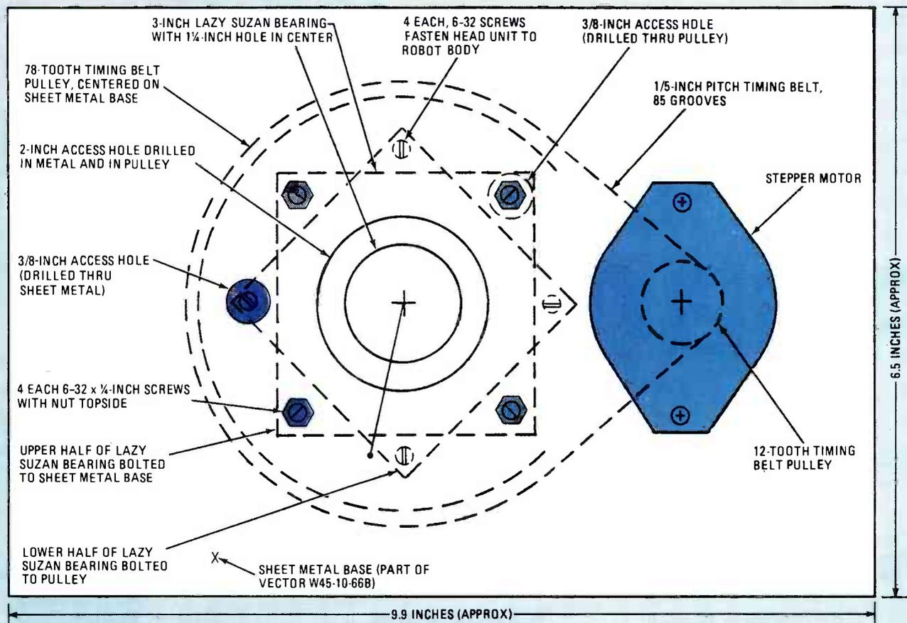
FIG. 2—THE HEAD'S DRIVE-TRAIN is detailed in this top view.
