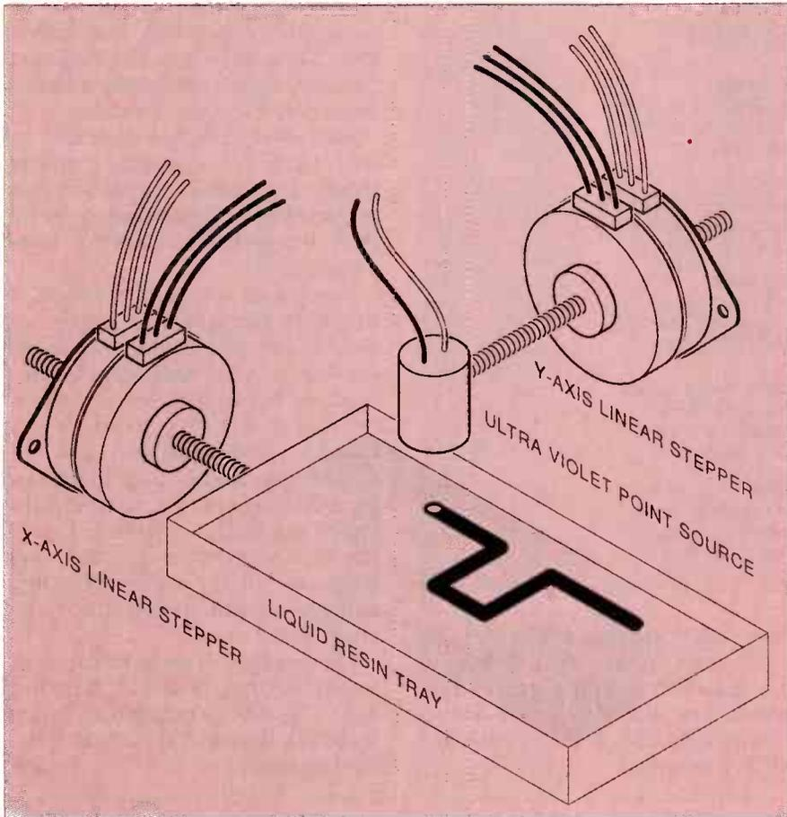
FIG. 4—TWO-DIMENSIONAL SANTA-CLAUS MACHINE can create a replica of virtually any flat object through the selective ultraviolet hardening of a liquid plastic resin.
