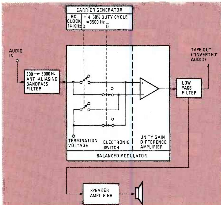
FIG. 4—FUNCTIONAL DIAGRAM OF THE SCRAMBLER. The switching is actually done by a balanced modulator that is driven from the carrier generator.
