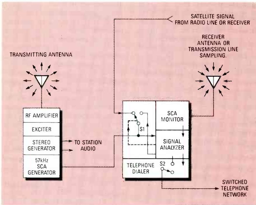
FIG. 4—THE FUNCTIONAL CUE PAGING MONITORING SYSTEM at the FM station. In the event of SCA signal failure, the equipment automatically dials a central monitor, who can instruct the equipment to switch to a dial-up telephone signal feed if necessary.
