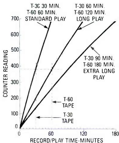
FIG. 3—THIS IS HOW the calibrations for "short" tapes work out for a particular Magnavox 3-speed VCR.
