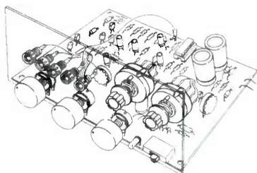
**1 MHz FUNCTION GENERATOR KIT.** Covers 0.1 Hertz to 1 MHz in 6 ranges. 100:1 frequency ratio. Sine, Triangle & Square waves available. (with DC offset). TTL output. FM & AM modulation inputs. 47 ohm output. Includes all parts, board, power supply and face plate decal. Excellent detailed assembly and theory of operation manual included. Superb classroom project. \$99.95 (Free Shipping). **OCTE ELECTRONICS, Box 276, Alburg, VT 05440. (514) 739-9328**
