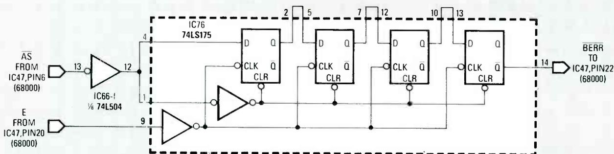
FIG. 2—A BUS ERROR (BERR) IS GENERATED if the address strobe (AS) continues through four E cycles without a data acknowledge (DTACK).
