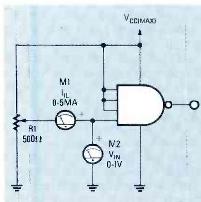
FIG. 6—THIS IS THE TEST CIRCUIT for measuring  $I_{IH}$ .
