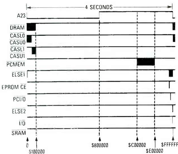
**FIG. 4—VARIOUS OUTPUTS OF THE ADDRESS DECODER** are shown here; these waveforms will be seen only with the test circuit (shorted data bus, etc.) installed.
