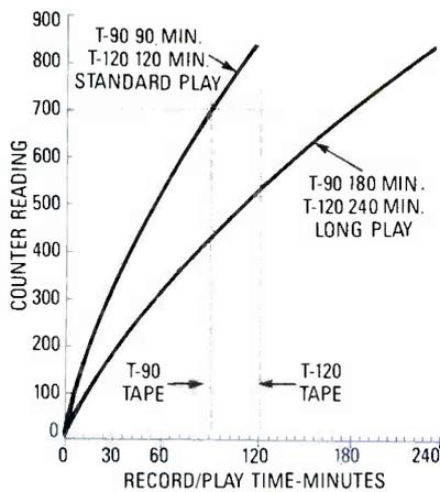
FIG. 2—BECAUSE THE SAME SIZE hubs are used, the curve for a T-90 tape is the same as the first three-fourths of a T-120 tape.
