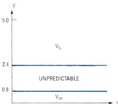
FIG. 2—THE MINIMUM AND MAXIMUM voltage limits of  $V_{IH}$  and  $V_{IL}$  for TTL negative logic (NAND, NOR). For positive logic (AND, OR) the values are reversed.
