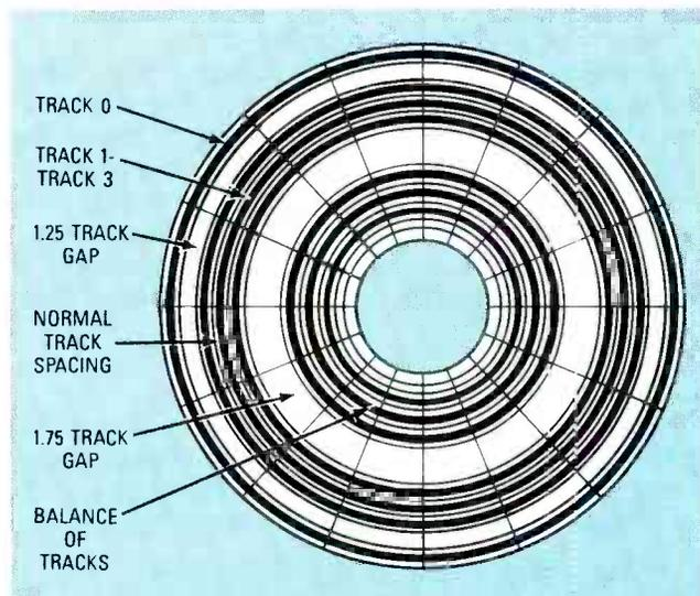
**FIG. 6—NON-STANDARD TRACK WIDTH** is achieved by stepping the read/write head in 1/4-track increments.
