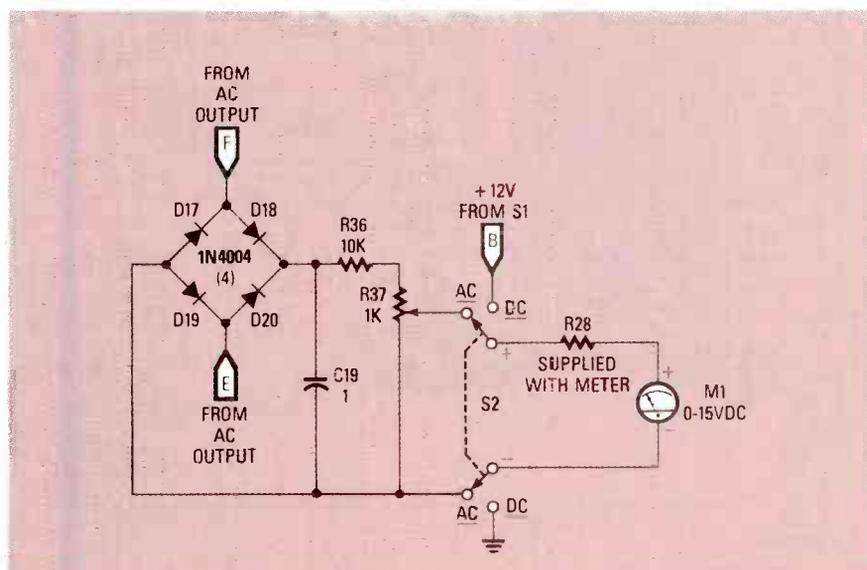
FIG. 4—THE METER CIRCUIT MEASURES both the battery voltage and the UPS output voltage. It is calibrated to the output voltage by potentiometer R37.
