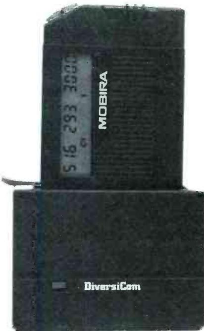
FIG. 3—THE LCD DISPLAY LOOKS LIKE THIS when data is received. In addition to the numeric data, the display shows the memory it's in and the access ("C") code being used. The unit is shown in its charger base, which permits simultaneous reception and charging of the NiCd batteries.
