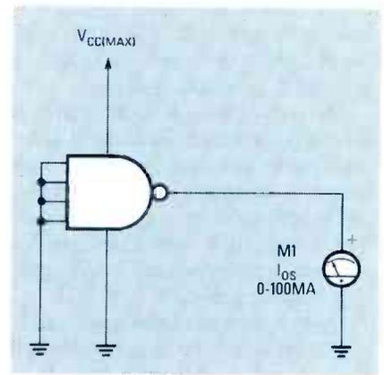
FIG. 7—THE TEST CIRCUIT for measuring  $I_{OL}$ .
