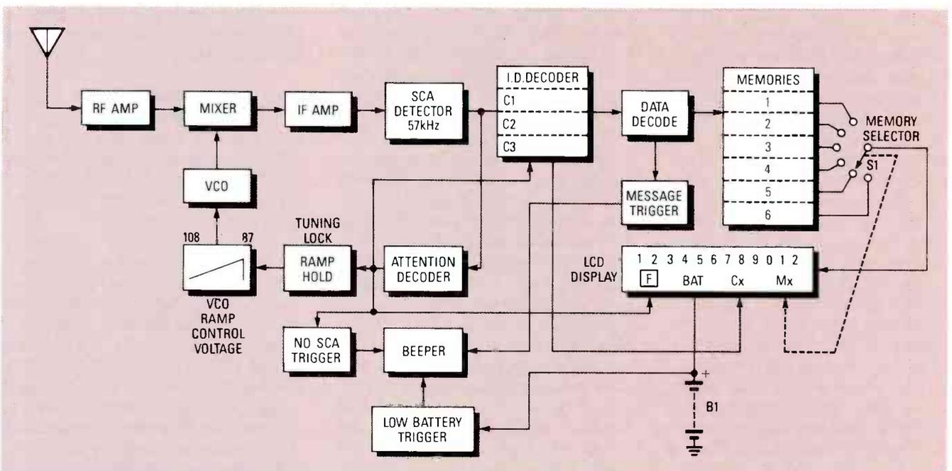
FIG. 2—THE PAGING RECEIVER'S FUNCTIONAL CIRCUIT. The six memories are arranged in a stack so that the most recent message fills the first memory, pushing the other messages down the stack until the one at the bottom, in memory 6, "falls out."
