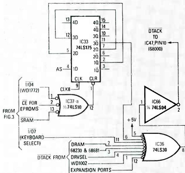
**FIG. 5—THE DTACK GENERATOR** is similar to the BERR circuit shown in Fig. 2. Here, however, the shift register (IC33) prevents the computer from locking up should a memory or I/O device not supply a data acknowledge.
