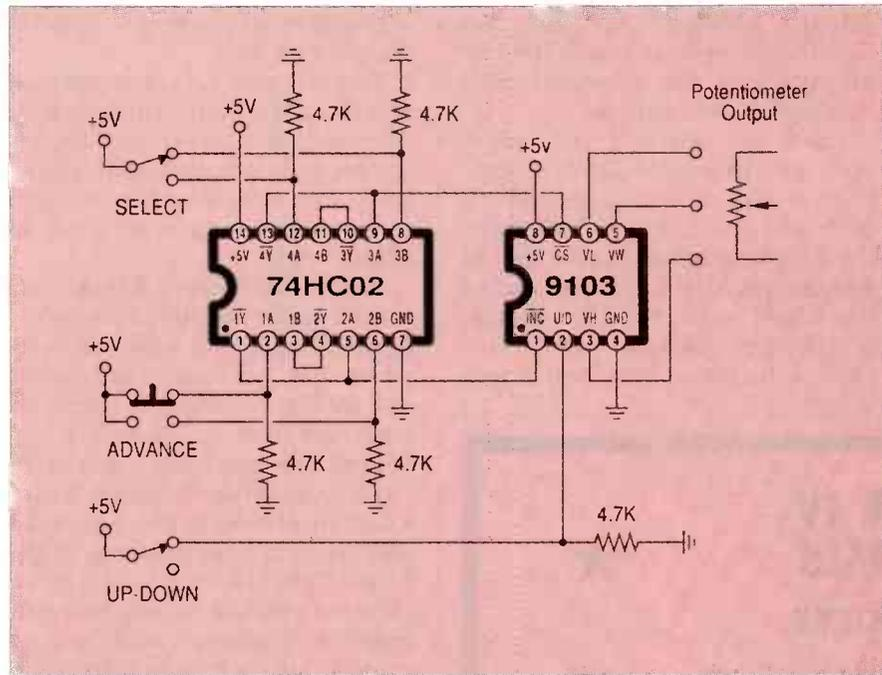
FIG. 3—USE THIS CIRCUIT to test your EEPOT. The debouncing shown is only needed when you are using mechanical contacts.
