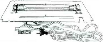
Complete, functioning assembly includes ballast, on-off switch, power cord, sockets and F4T5-BL blacklight. Mounted on a 7 1/8" X 3 1/8" metal plate. Use for special effects lighting or erasing EPROMS.
