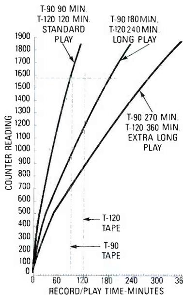
FIG. 4—USING "LONG" TAPES on the Magnavox VCR, we find that the calibrations for the 0-500 reading are exactly the same as those for the shorter tapes.
