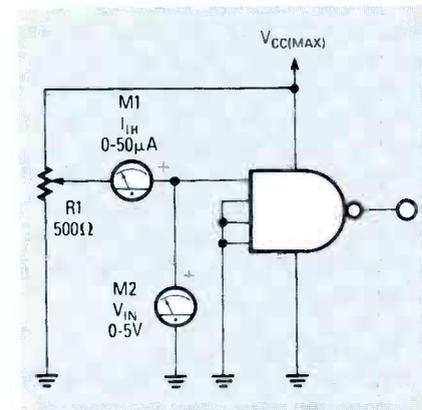
FIG. 3—THE TEST CIRCUIT used for measuring  $V_{IH}$ ,  $V_{OL}$ , and  $I_{OL}$ .
