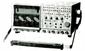
PANASONIC MODEL VP-5720A is a 2-channel, 50-MHz repetitive bandwidth DSO featuring a 15-MHz single-shot bandwidth and a 40 Ms/s sampling rate. It has a 8K × 3 memory storage and an expandable memory option.
