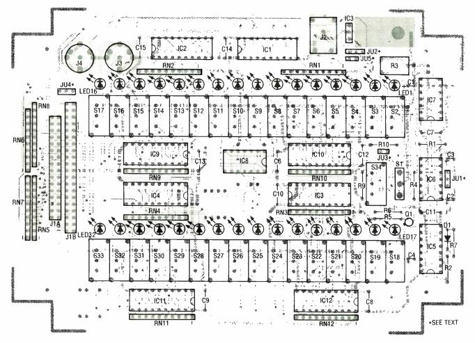
FIG. 5—MOUNT ALL COMPONENTS as shown here. Note that C4, J2, and all five jumper headers mount on the foil side of the board.
