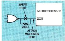
FIG. 6—CONNECT MICRO-MON to the target system directly, or insert a resistor in series with the watt line.
