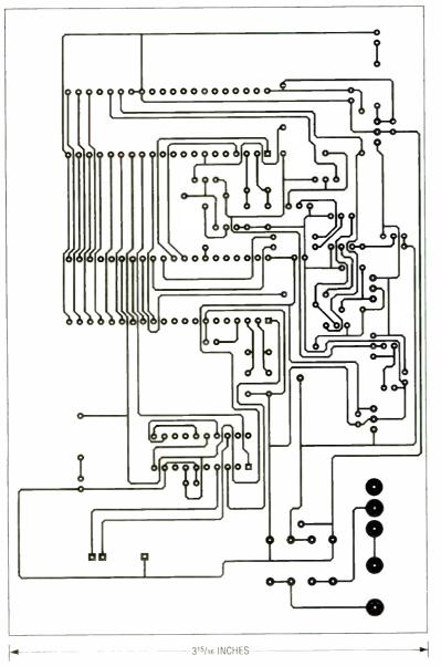
FOIL PATTERN for the microcontroller programmer, shown actual size.
