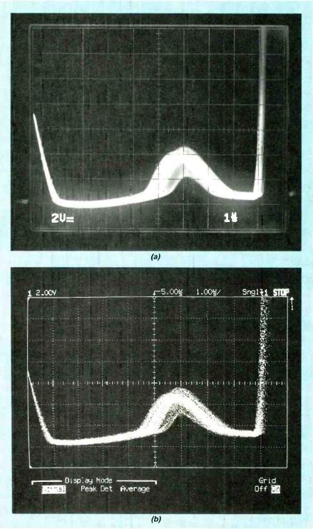
FIG. 1—REAL-TIME DISPLAY OF PULSE JITTER on an amalog scope shows far more detail (a) than on a digital scope display (b).
