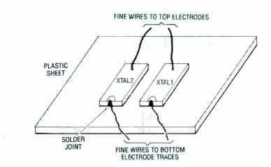
FIG. 3—TRANSDUCER CONSTRUCTION. Silver-bearing solder is used to avoid lifting the silver electrode from the ceramic crystal surface. Energy conversion is most efficient when crystals are "air-backed" resulting in energy being radiated from the front of the crystal.
