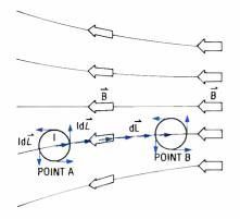
FIG. 1—A MAGNETIC DIPOLE IN A B FIELD is moved from point A to B along the path composed of  $d_L$ . The force vector on any small segment of the current loop is  $dF_m = IdI \times B$ .  $dF_m$  is directed out of the page as is the total force  $F = \oint IdI \times B$ . The force vector is perpendicular to dL, so the work done on  $F \cdot d_L$  is zero. If the dipole is rotated so that F was not normal to the paper, then work would be done.
