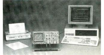
TEKTRONIX' ANALOG 2252 4-channel scope with a 12-bit A/D converter, an Epson FX-series printer, and an IBM remote PC all combined to form a complete recording package.
