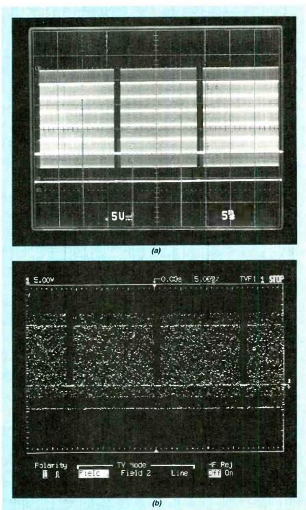
FIG. 2—THE FIVE MODULATED COLOR LEVELS OF A VIDEO SIGNAL are clearly / sible in the intensity variations of an analog scope display (a), while a dots-only digital scope display conveys little information about the signal's actual complexity. A digital scope's vector display would connect the dots for a clearer outline of the waveform, but still wouldn't provide the intensity variations that distinctly show the modulated color levels.
