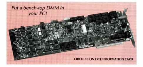
here is no turning back the clock: PC-based test equipment is here to stay. The reason for that is flexibility of the sort available from the PCI-DMM from Global Specialties (70 Fulton Terrace, New Haven, CT 06512).
