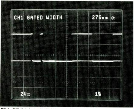
FIG. 6—THE ANALOG PRECISION of a gated width counter measurement allows a narrow spike (276 ns) to be measured with nanosecond resolution, even at a 1 ms/division sweep speed. A digital scope would need a 10-megapoint record length for the same resolution on the same display.
