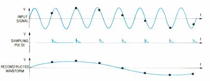
FIG. 6—A RECONSTRUCTED WAVEFORM is shown from an input signal that has been sequentially sampled.
