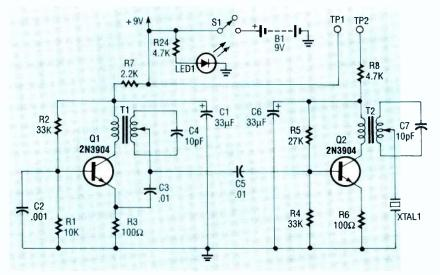
FIG. 1—THE TRANSMITTER CIRCUIT. Q1 is an RF oscillator whose 2.25-MHz frequency is determined by C4 and T1. A secondary tap on T2 provides a low-impedance output to drive XTAL1 in the transducer.
