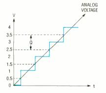
FIG. 7—QUANTIZING BY A/D converters transforms analog voltages into digital binary bits at selected levels.
