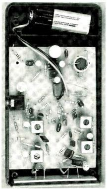
FIG. 4—THE AUTHORS' PROTOTYPE. Note that LED1 and S1 are mounted on the foil side of the PC board. The transducer is mounted on the end plate of the enclosure with its leads close to their solder pads.
