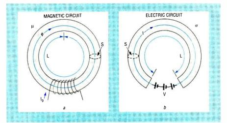
FIG. 2—MAGNETIC FLUX IS ANALOGOUS TO ELECTRIC CURRENT. In (a) the magnetic path of length L and cross-sectional area S is in a material of permeability  $\mu$ . The source of magnetomotive force nl<sub>o</sub> is the current l<sub>o</sub> encircling the material n times. In (b) the electrical path is in a material of conductivity  $\sigma$ . The source of electromotive force nV is a battery of n cells each with a voltage V.
