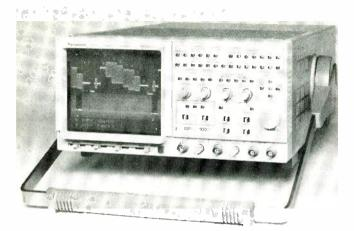
PANASONIC MODEL VP-5741A has the same features as the 5720A except it has an analog bandwidth of 100 MHz with a sampling rate of 100 Ms/s and a 10K × 3 memory storage.
