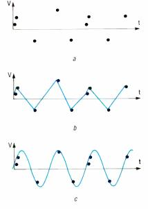
FIG. 2—INTERPOLATION METHODS; a dot display (a) has no interpolation, a linear interpolator connects the dots with vectors (b), and sine interpolation (c).
