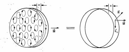
FIG. 5—ELECTRIC CURRENTS associated with individual magnetic dipoles cancel inside the material. At the surface, however, the currents are in the same direction resulting in a net surface current  $I_b$ .  $I_b$  is bound to the surface since it consists of pieces of the dipole currents bound in the material.
