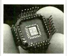
THIS EXPERIMENTAL PROTOTYPE of a high-temperature superconducting device, developed by researchers at Bellcore using an experimental process called pulsed excimer laser deposition, could be used to create new generations of powerful computerized switches.
