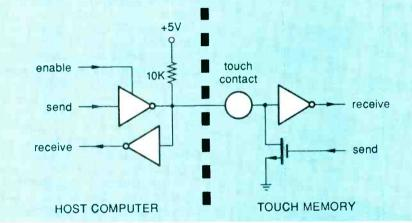
FIG. 5-ONLY A SINGLE CONTACT IS NEEDED to read from or write to your touch memory. Here is how it gets done.
