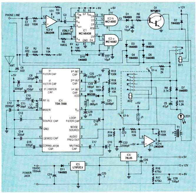
FIG. 2—SCHEMATIC OF THE FM ON-HOLD unit. The output of IC1, a DTMF decoder, is a 4bit word that controls the on-hold logic. The FM receiver, IC4, uses a frequency-locked loop system with a 70-kHz intermediate frequency, which is tuned by a tank circuit consisting of L2 and D9. Spurious reception is eliminated by a mute circuit in the IC.
