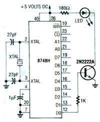
FIG. 5—EXPENSIVE LED BLINKER circuit. While it is somewhat overkill, it is very useful as a teaching tool. The software for this circuit is shown in Listing 2.
