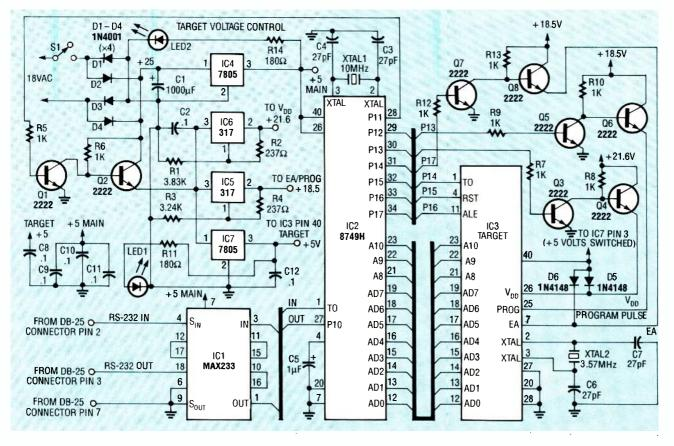
FIG. 1—PROGRAMMER SCHEMATIC. The MAX233 RS-232 driver/receiver (IC1) converts the signals from your serial port to TTL levels for the 8749H and vice versa.
