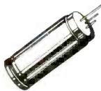
A low power collimator pen containing a MOVPE grown gain GaAlAs laser. This collimator pen delivers a maximum CW output power of 2.5 mW at 820 nm. The operating voltage of 2.2-2.5V @ 90-150mA is designed for lower power applications such as data retrieval, telemetry, alignment, etc.
