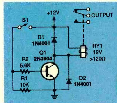
FIG. 12—TRANSISTOR-DRIVEN RELAY with a coil damper.
