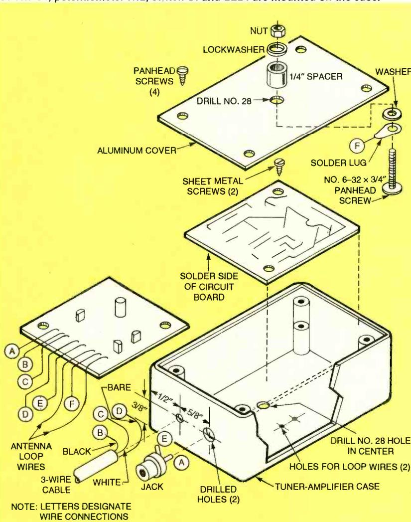
FIG. 6—ASSEMBLY DIAGRAM FOR THE TUNER AMPLIFIER. The circuit board is mounted in an inverted position, and the complete unit moves with the loop antenna.
