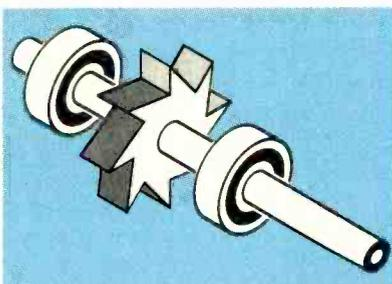
**FIG. 1—THE \$14 ORALSAFE DENTAL handpiece can be cut down to provide an air turbine the size and mass of a plotter pen. Air blown tangentially across the nylon pawl rotates the hollow shaft at extremely high speeds.**
