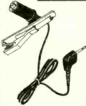
Miniature electret condenser microphone designed for use with cellular phones but they are great in other audio applications. Black 0.3" diameter X 0.43" mike and 12 foot flexible cord with 3.5 mm mini-plug. Includes chrome-plated alligator clip which can be used for attachment to auto visor or clothing.
