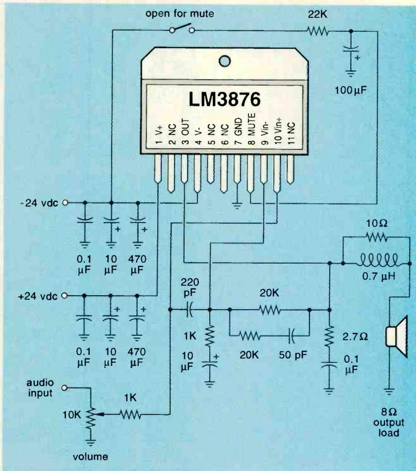
FIG. 3—NATIONAL SEMICONDUCTOR CORP. has a new line of exceptionally rugged Overture audio amplifiers. Here is a typical 40-watt circuit.
