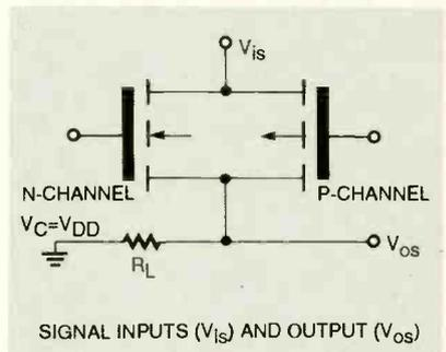
FIG. 20—CD4066B BILATERAL SWITCH power connections for digital and analog signals.
