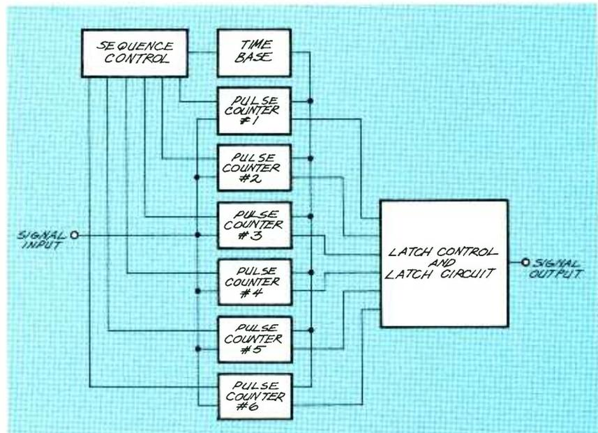
**FIG. 1—YOU NEED SIX COUNTERS** to update the display every second. The first counter counts pulses 1 to 6, the second counts pulses 2 to 7, the third 3 to 8, and so on.
