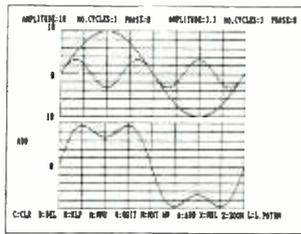
Figure 1. Addition of Sine Waves
