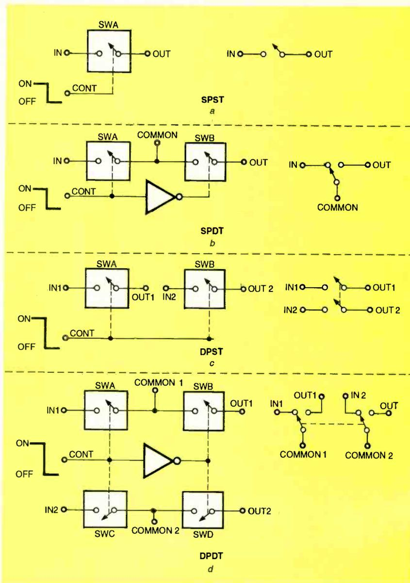
FIG. 22—FOUR BASIC SWITCHING functions organized on a CD4066: SPST (a), SPDT (a), DPST (a), and DPDT (a).
