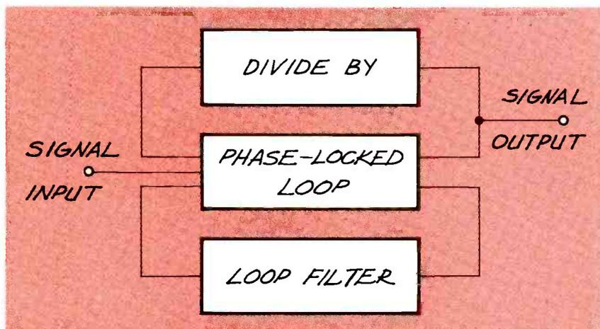
FIG. 2—THE HEART OF THIS DESIGN is a PLL with a divider circuit inserted between the VCO output and the PLL's comparator input.
