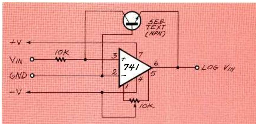
**FIG. 2—LOGARITHMIC AMPLIFIER** built with a single op-amp. The current in the feedback loop of the op-amp is equal to the current flow at the input of the op-amp.
