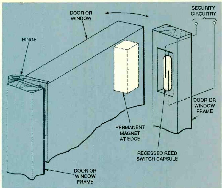
FIG. 15—REED-SWITCH CAPSULE RECESSED in a door or window frame is triggered by a permanent magnet recessed in the door or window edge. Together they function as an input switch in an intrusion detection system.
