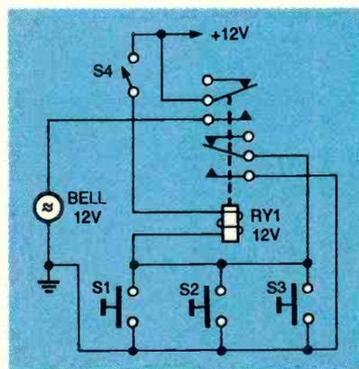
FIG. 8—BURGLAR ALARM that includes a self-latching relay.
