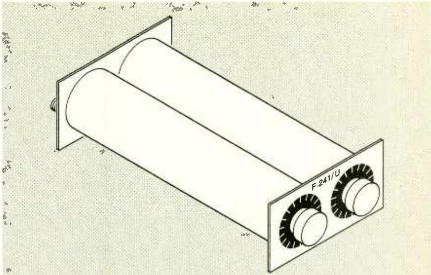
FIG. 4—SURPLUS F-241/U OR F-243/U TWIN CAVITIES are easily converted into tuning preselectors that can improve long-distance FM reception.
