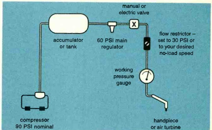
FIG. 2—A TYPICAL SUPPLY SYSTEM that will drive air turbines.
