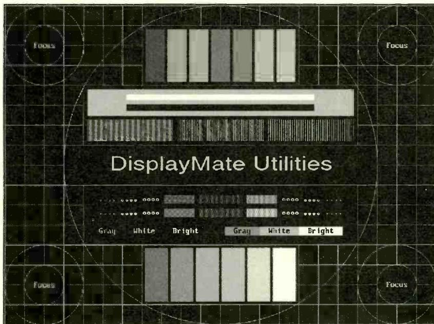
FIG. 4—DISPLAYMATE SERVES UP a slide show of test patterns that show you how to adjust your monitor for optimum brightness, contrast, color balance, and other variables for the best possible image.
