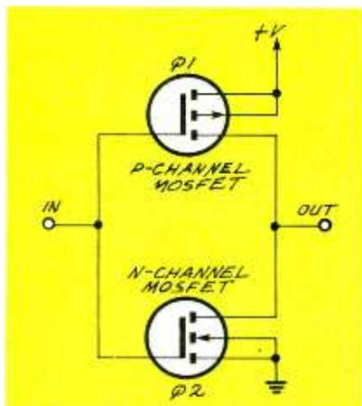
**FIG. 1—A TYPICAL CMOS INVERTER.** Each transistor has a small gate capacitor at its input. The input capacitors are extremely fragile, and it doesn't take much ESD to damage them permanently.
