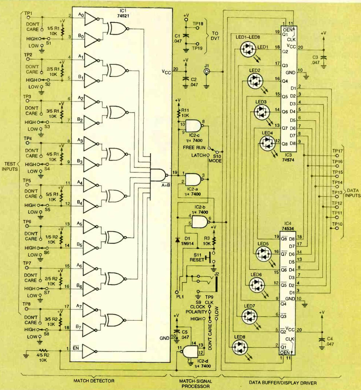
FIG. 1—THE DIGILYZER HAS THREE FUNCTIONAL SECTIONS: a match detector, a match-signal processor, and a data buffer that performs double-duty as a display driver.
