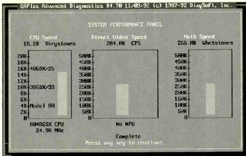
FIG. 1—THE DHRYSTONE AND WHETSTONE benchmarks are available in QAPLUS. The diagnostic software can also measure hard-disk drive performance and it comes with a CMOS editor.
