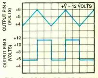
FIG. 13—GRAPH OF VCO OUTPUT waveforms for the generator circuit of Fig. 9.
