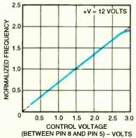
FIG. 11—GRAPH OF NORMALIZED frequency of the Fig. 9 circuit as a function of control voltage.
