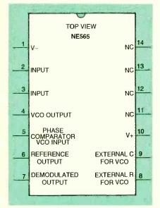
FIG. 2-PINOUT DIAGRAM of the NE565.
