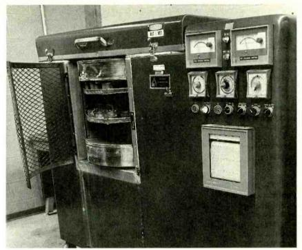
AMBIENT TEMPERATURES inside a chamber at Motorola Semiconductor typically range from -65°C to 150°C.
