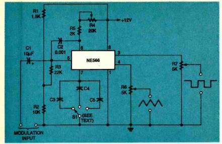
FIG. 14—THREE-BAND FM GENERATOR based on the NE566 general-purpose function generator.
