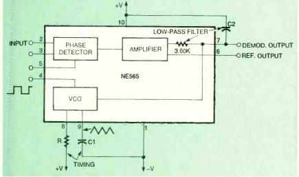
FIG. 1-BLOCK DIAGRAM OF THE NE565 phase-locked loop IC.
