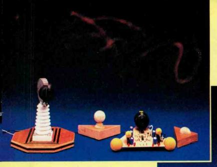
FIG. 1—WATCH THE DANCING BALL on the end of the spring. An erratically oscillating solenoid on the Bonker sends the ball into unpredictable gyrations captured with time exposure (left). The Bonker at rest (below). Spring-mounted balls on stationary bases add to the chaotic effect.
