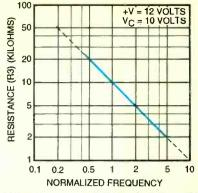
FIG. 12—GRAPH OF NORMALIZED frequency of the Fig. 9 circuit as a function of resistance R3.
