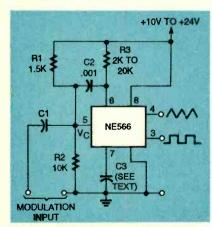
FIG. 9—FIXED FREQUENCY GENER-ATOR circuit based on the NE566 function generator.
