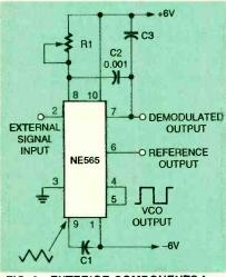
FIG. 3—EXTERIOR COMPONENTS for a signal trackerand FM-demodulator.
