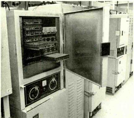
BURN-IN CHAMBER at Motorola Semiconductor exposes test devices to thermal stress under power.
