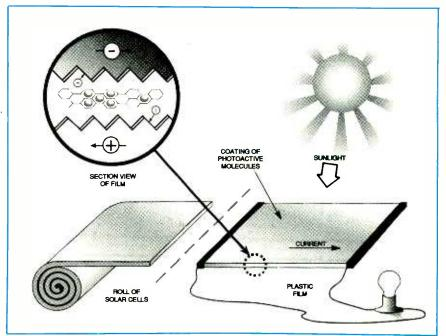
FIG. 1. SUNLIGHT STRIKES PHOTOACTIVE MOLECULES on a thin plastic film causing positive and negative charges to separate and jump to electrically conductive strands in the plastic film. Positive charges flow one way and negative charges flow the other way, causing current to flow.
