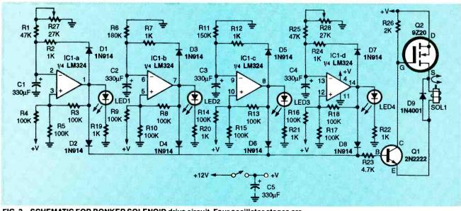
FIG. 3—SCHEMATIC FOR BONKER SOLENOID drive circuit. Four oscillator stages are formed from a quad LM324N op-amp IC. LEDs provide a visual indication of the pulse output of each stage.
