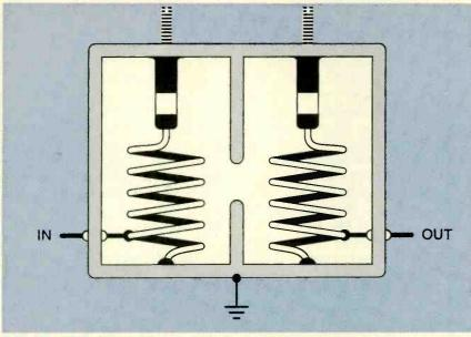
FIG. 4-A TWO-STAGE FILTER made from helical resonators. Energy is coupled between resonators by the hole in the wall. The input and output taps serve as impedance step-up and step-down transformers.
