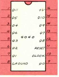
FIG. 1—4040 PINOUTS. The only control pins the chip has are the clock input (pin 10) and an active-high reset (pin 11).
