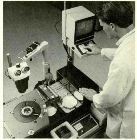
ELECTRICAL TESTS are made on a semiconductor device wafer to eliminate faulty units prior to environmental testing.
