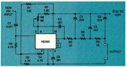
FIG. 6—60 kHz FM DEMODULATOR with a single-ended power supply.
