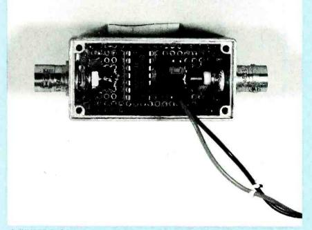
A JUMPER BLOCK was substituted for a triple-throw switch to conserve space.
