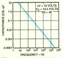
FIG. 10—GRAPH OF FREQUENCY as a function of capacitance for an NE566 when R3 = 4 kilohms.
