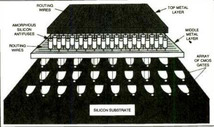
FIG. 2. A THREE-LAYER, STACKED, FIELD-PROGRAMMABLE GATE ARRAY economizes on silicon. Current programmed to flow through the amorphous silicon antifuse layer forms permanent connections that dedicate the array of CMOS gates for a specific application.
