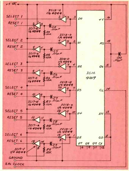
FIG. 3—THE 4017 IS THE MAIN PART of the sequence control section. The 4017 is clocked at an update rate of half a second, or 2 hertz.
