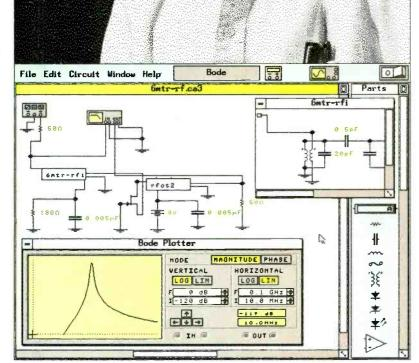
Analog Module: Tuning an RF front end.
