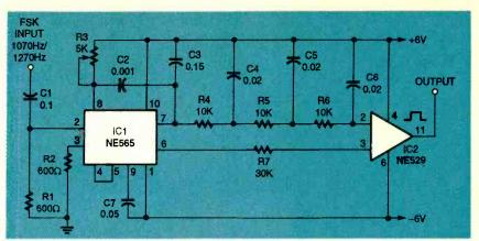
FIG. 5—FREQUENCY SHIFT KEYING (FSK) demodulator circuit.
