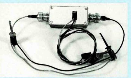
FIG. 3—COMPLETED FREQUENCY DOUBLER. The power leads are fitted with microclips and attached to two extra pins on the jumper block.
