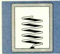
FIG. 3—THE HELICAL RESONATOR is a cavity variation that is more suitable for VHF and UHF. They can be easily made from wire and printed circuit board stock.
