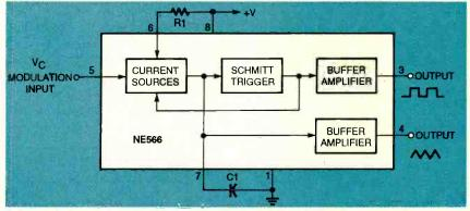
FIG. 7—FUNCTIONAL BLOCK DIAGRAM OF THE NE566 function generator.
