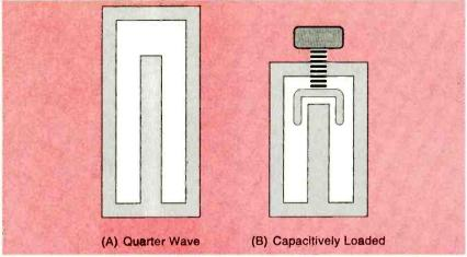
FIG. 2—A CAVITY is any conductive enclosure that can support resonance. These are common at microwave frequencies. Energy can be coupled in or out with magnetic loops, electric probes, or electron beams. Here are cross sections of two examples of simple coaxial cavities.
