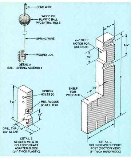
FIG. 5—DETAILS OF MECHANICAL PARTS: ball-spring assembly (Detail A); solenoid shaft adapter block (Detail B); solenoid/PCB support post (Detail C).
