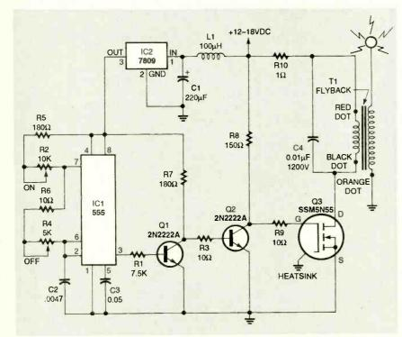
FIG. 2—THE SOLID-STATE TESLA CIRCUIT consists of a pulse generator, a driver circuit, and a high-voltage transformer. The 555 timer (IC1) runs in its astable mode, producing a continuous pulse train.
