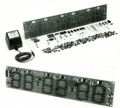
FIG. 1—183 PARTS (top) are combined to make an eye-catching clock (bottom).
