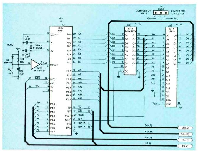
FIG. 6—FIRMWARE FOR THE 8031 MICROCONTROLLER is contained in EPROM IC14. Jumper J4 allows the use of larger EPROMs.
