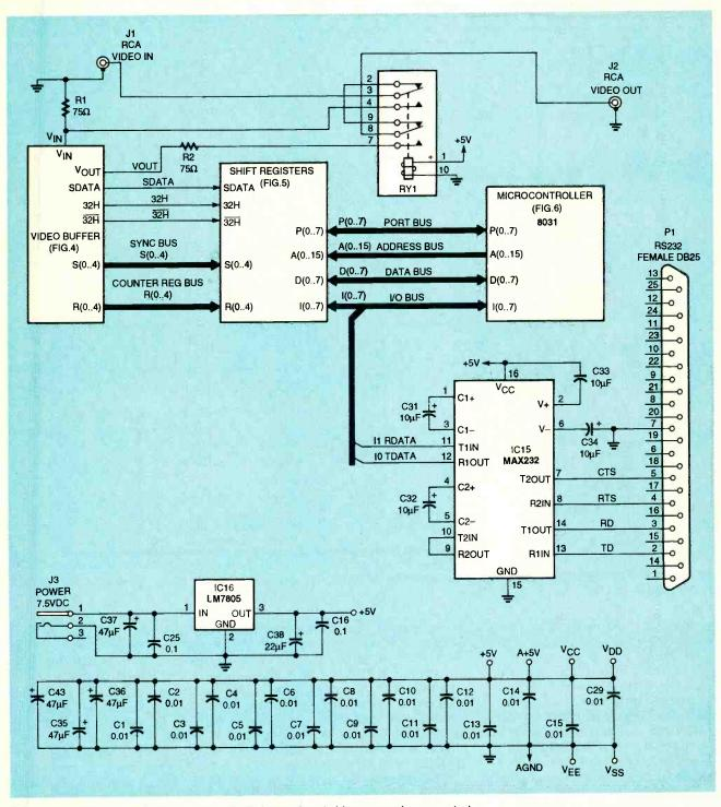
FIG. 3—TEXTGRABBER BLOCK SCHEMATIC. A base-band video source is connected to J1. The video signal is terminated on the TextGrabber, and a buffer drives the video back out to J2.
