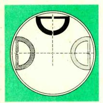
Fig. 6. Finding the center of the tray using a protractor and a straight edge; the point where the lines cross is the center of the circle.
