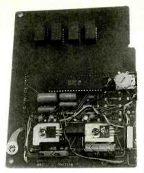
Fig. 13. A section of an alarm board, bought through surplus, that contains a 7107. This particular board also contains the ± 5-volt power supply.
