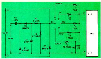
Fig. 4. Adding this circuit to the 7107 produces a versatile digital voltmeter (DVM). Both AC and DC voltages in five ranges up to 2,000 volts are accurately measured.
