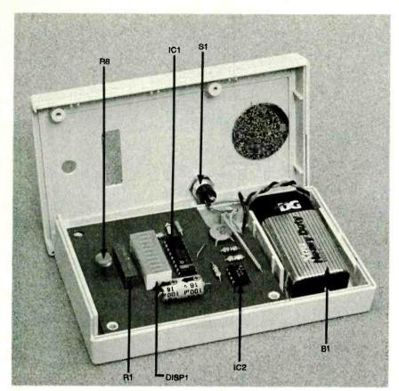
The Zonal Enlarging Meter with PC circuit board and battery B1 in position just prior to closing the plastic case. Note the holes cut for the photoresistor R8 and LED bargraph display DISP1. The photoresistor is mounted above the PC board to be flush with the inside surface of the case's cover.
