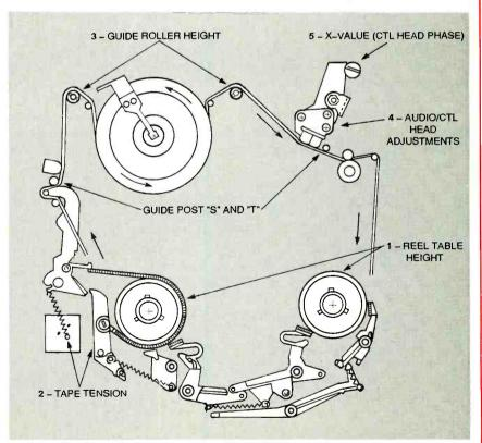
FIG. 1—THE VHS TAPE PATH shown here is from a Hitachi unit, but it is common to many VHS VCR's. Note the five major adjustment points.
