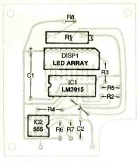
Fig. 2. Parts location diagram shows that the PC board is uncluttered and easy to assemble. Mounting holes align with the screws used to close the plastic case.
