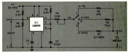
Fig. 12 To measure higher frequencies than the LM2917 can handle, this circuit does the job quite well. Frequencies in 3 ranges up to 2 MHz (1.999 x 1000) can be measured.
