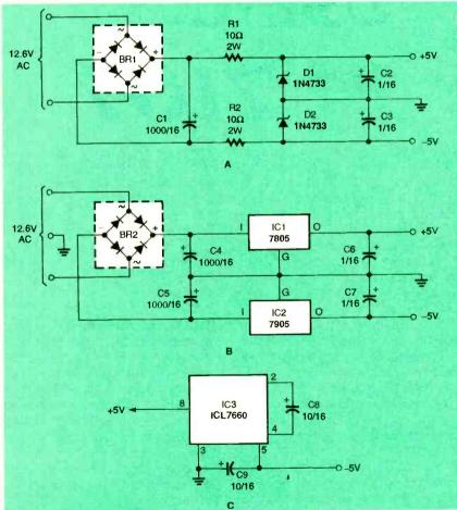
Fig. 2. Here are a few different methods of generating the + and -5-volt power required by the 7107. A pair of Zener diodes (A) are handy if the transformer you want to use does not have a center tap. A pair of three-terminal regulators (B) and a center-tapped transformer also work well. An interesting alternative is the ICL7660 chip (C), which generates a negative-voltage output from a positive-voltage input.
