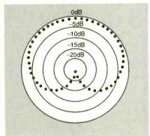
FIG. 7—A CARDIOID PICKUP PATTERN reduces the likelihood of acoustic feedback.
