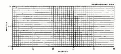
**FIG. 4**—A LOW-PASS FILTER built by cascading three trisamps. This is a "distortionless" or linear-phase filter that is extremely difficult to build using older analog techniques. To simplify your final design, using ordinary algebra easily reduces three cascaded trisamps into a single, seven-sample "septsamp." Additional samples improve response shape.
