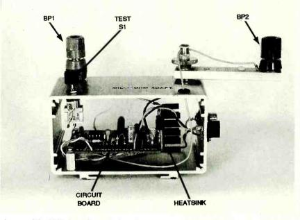
A view of the Milliohm Adapter before the side covers are installed. Note that the heat sink has been attached to the Darlington transistor Ql and stands free of any metallic contact.
