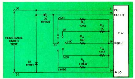
Fig. 6. Although you could measure resistance with a simple voltage-divider circuit, the use of a Zener diode and a switch-selectable resistor to change the 7107's reference voltage makes it easier to measure resistances up to 2 megohms.
