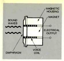
FIG .2—MICROPHONES CONVERT sound waves into electrical signals.
