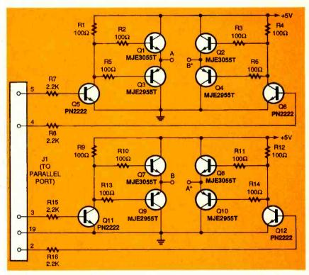
Fig. 3. The driver circuit allows a standard PC parallel port to alter the direction of current flow in both windings of the stepper motor according to the states of the four inputs.
