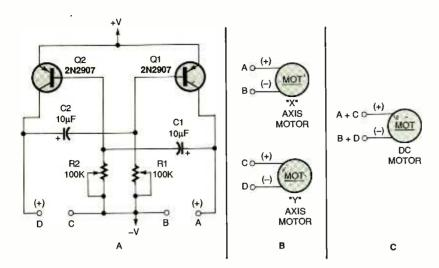
**FIG. 5**—THE MOTOR-CONTROL CIRCUIT (A) can be used to alternately turn two motors on or off (B). It can also be used to make one motor turn first in one direction and then the other (C).
