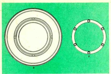
Fig. 5. The rotating tray—the complete assembly is shown in a, and the ball-bearing ring in b.
