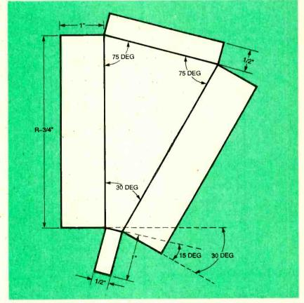
Fig. 7. Use this pattern to create the bins. The length of a side is given by the radius of the tray minus three-quarters of an inch. You'll need twelve of these.
