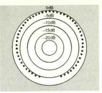
FIG. 6—A MICROPHONE WITH AN OMNI-DIRECTIONAL pattern like this one picks up sounds from all directions.
