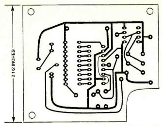
Same-size foil-pattern diagram for the meter's PC board. Carefully drill holes so that integrated-circuit chips and display chip mount quickly.
