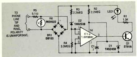
FIG. 1—AT THE HEART of the circuit is an ultra-low-current voltage-level sensor that draws only about 5  $\mu$ A when the phone line is not in use.
