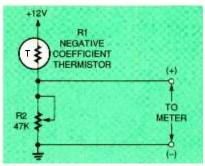
Fig. 7 A simple voltage-divider circuit using a negative-temperature-coefficient (NTC) thermistor is a low-cost and accurate method of measuring temperature with the 7107. An NTC thermistor's resistance drops as its temperature rises. If you switch the locations of RI and R2, the reading on the 7107 will drop with rising temperature.
