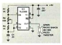
**FIG. 1**—THIS OSCILLATOR emits a tone that can be varied between 6 and 25 kHz. The higher frequencies can not be heard by most humans, although dogs can hear it just fine.
