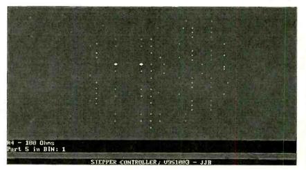
Fig. 1. The automated-parts-tray screen displays a grid overlaid with mounting holes for each component. The current component is highlighted.
