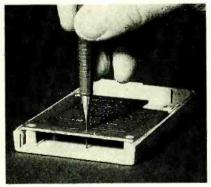
Fig. 3. Prior to inserting parts onto the PC board, extend the lead of an automatic pencil through the holes in the board to locate openings in the case cover for the LED bar-graph display DISP1 and photoresistor R8.
