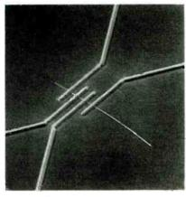
NEC RESEARCHERS MEASURE the electrical conductivity of individual carbon nanotubes by attaching four 80-nanometer-wide tungsten leads to each nanotube.
