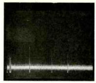
THE OSCILLOSCOPE'S DISPLAY of the HSA output when a short-wire antenna is connected to the BNC connector. The extreme left burst is an unknown signal. Local radio-control signals from left to right are at 27.995 MHz, 53.4 MHz, and 72.280 MHz.
