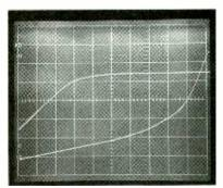
THE SWEEP-CIRCUIT OUTPUTS as viewed on an oscilloscope. The lowermost curve is the varactor (sweep) drive waveform—the bottom grid line is 0.0 volts, 5-volts per division. The uppermost waveform is the local-oscillator boost waveform—l-volt/division, top of trace is 4.5 volts. Both curves are displayed on a 1-ms/division time base.
