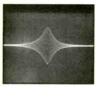
THE OSCILLOSCOPE'S VIEW of the bubble sampled from the preamplifier assembly's test point after the 145-MHz IF filter alignment. The oscilloscope's  $10 \times$  time-base magnifier is switched on. You should be able to see the zero beat at the center of the bubble.
