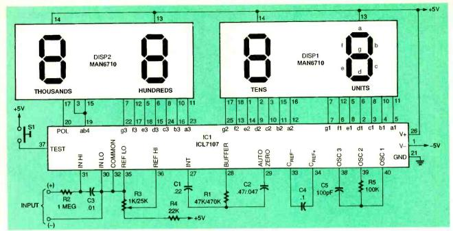
Fig. 1 The 7107 was originally designed to be a self-contained, highly accurate voltmeter. By changing the values of C2, R1, and R3, the 7107 can have a range of 200-mV or 2 volts.
