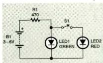
FIG. 3—THIS SIMPLER SOLUTION to the switch-operated LED problem takes advantage of the fact that red LEDs have a lower voltage drop than green ones.
