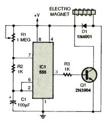
FIG. 3-A SIMPLE TIMER built around a 555 gives you a switching electromagnet to use to create laser-light patterns.
