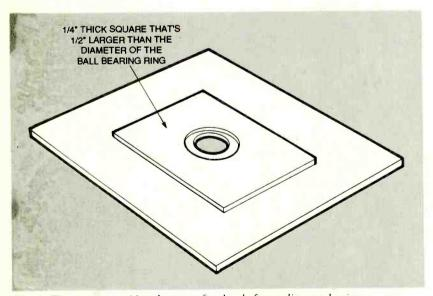
Fig. 9. The spacer provides clearance for the shaft-coupling mechanism.
