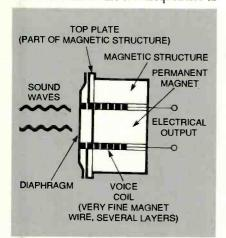
FIG. 4—THE BASIC DYNAMIC MICRO-PHONE. It is probably the most commonly used variety.
