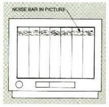
FIG. 6—THE NOISE BAR THAT APPEARS in the picture can be caused by a misadjusted guide roller.
