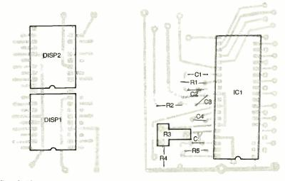
Fig. 3. If you want to build your own 7107 voltmeter, you can follow the parts placement diagrams here. Using sockets for the 7107 and the displays make troubleshooting easy.
