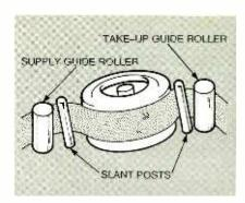
FIG. 5-TWO GUIDE ROLLERS-one before the video-drum assembly, one after-determine the tape position as it travels across the video heads.
