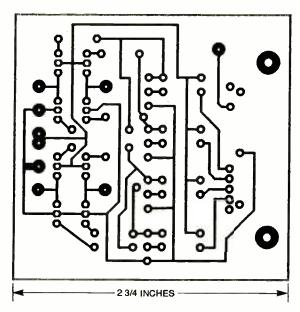
Use this foil-pattern when etching the PC board.
