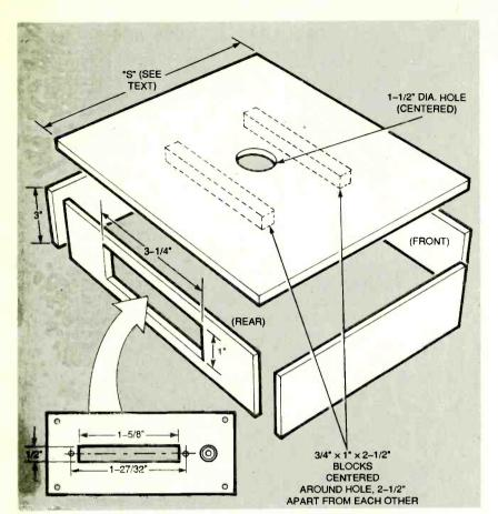
Fig. 8. One-half inch plywood serves well in building the case. The blocks on the underside hold the stepper motor, and the slot in the rear panel is for a mounting plate that connects power and the parallel port.
