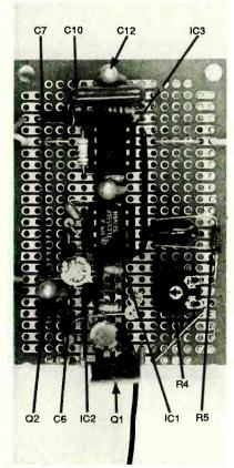
A piece of a PC board that matches a solderless board supports most of the circuit's parts. Layout is not critical; however neatness is important.
