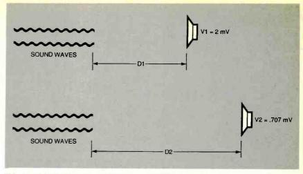
FIG. 3—A MICROPHONE'S OUTPUT FALLS OFF as it gets farther away from the source of the sound.
