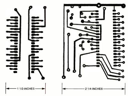
Here are the foil patterns for the basic 7107 voltmeter and the LED display. A split power supply and a handful of passive components turn the 7107 into an accurate, easy-to-use instrument. Putting the display on a separate board makes the project more versatile in terms of mounting arrangements. You can also combine both boards into one if you need to.
