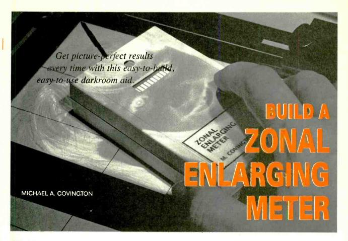
ost enlarging exposure meters tell you how many seconds to expose print paper. The Zonal Enlarging Meter described here does not! Instead, it tells you how light or dark each area of the picture will turn out, based on a selected standard exposure time for your enlarger.
