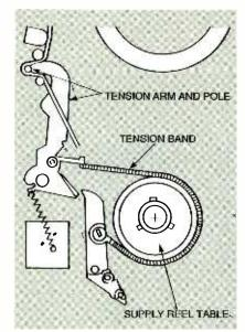
FIG. 4—TAPE TENSION MECHANICS are illustrated here. The tension band does most of the work.
