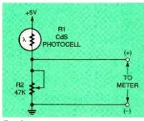
Fig. 8. We can measure light intensity the same way we measure temperature by substituting a cadmium-sulfide (CdS) photocell for the thermistor in Fig.7. In most CdS photocells, resistance will drop with an increase in brightness. Should you need to have the 7107's display reading drop as the photocell gets brighter, or if you have a photocell that increases in resistance with exposure to light, simply switch the positions of RI and R2.
