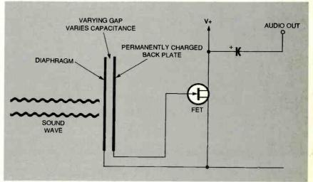
FIG. 5—AN ELECTRET CONDENSER MICROPHONE features a built-in FET amplifier.
