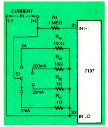
Fig. 5. With this circuit, the 7107 can measure DC current. The rotary switch lets you select from four ranges, with a capacity up to 2 amps.
