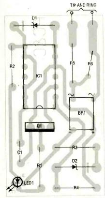
FIG. 2—IF YOU'RE USING A PC board, follow this parts-placement diagram. The LED can be mounted so that it can be bent in any direction, or remain straight up.
