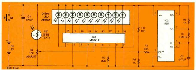
Fig. 1. Here's the schematic diagram for the Zonal Enlarging Meter. Light falling on photoresistor R8 causes LEDs in the bar-graph display DISP1 to illuminate. The number of LEDs that come on is logarithmically proportional to the light intensity.
