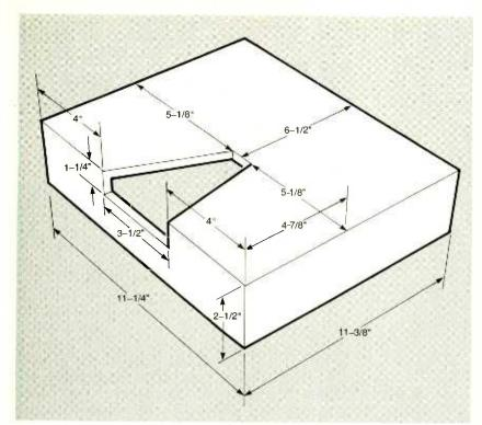
Fig. 10. The top cover is the same size as the base, and has a wedge-shaped cutout to allow access to the current bin.
