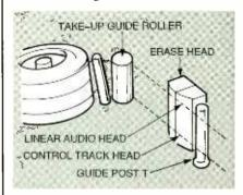
FIG. 7—ACE-HEAD ASSEMBLY is composed of three separate heads—audio erase, linear audio, and control track.
