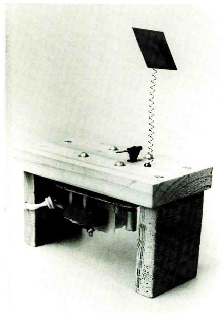
FIG. 2-FOR REPETITIVE VIBRATIONS, this simple set-up works well. A small gearreduction motor rotates a nail, which strikes the spring one time each revolution. That rotation creates a repetitive movement in the reflector.
