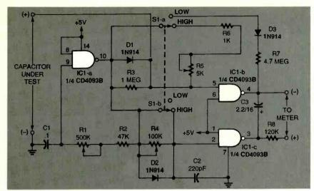
Fig. 10. With this circuit, the 7107 gains the ability to measure the value of capacitors from 2 pF to 2  $\mu$ F. Potentiometer R4 adjusts the circuit for a zero reading, while R1 and R5 calibrate the low and high ranges.
