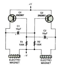
FIG. 4-IF THE ELECTROMAGNETS in this dual-timer circuit are arranged perpendicular to each other, a north-south, eastwest motion can be established.
