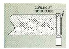
FIG. 2-TAPE CURLING AT THE TOP of the tape guide can be caused by a misadjusted reel-table height. If severe, it can physically damage the tape.
