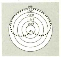
FIG. 8—WHEN FEEDBACK PROBLEMS are severe, try a hyper-cardioid type that delivers the polar pattern shown here.
