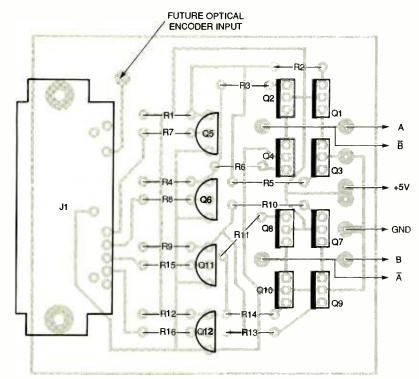
Fig. 4. Mount all components as shown here. A future installment will show how to use the optical encoder inputs.
