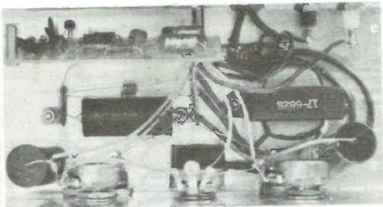
Fig. 5— Chassis view with cover removed from the case shows PC board mounted on the back panel. You may want to mount the dual-trace parts inside your scope.
