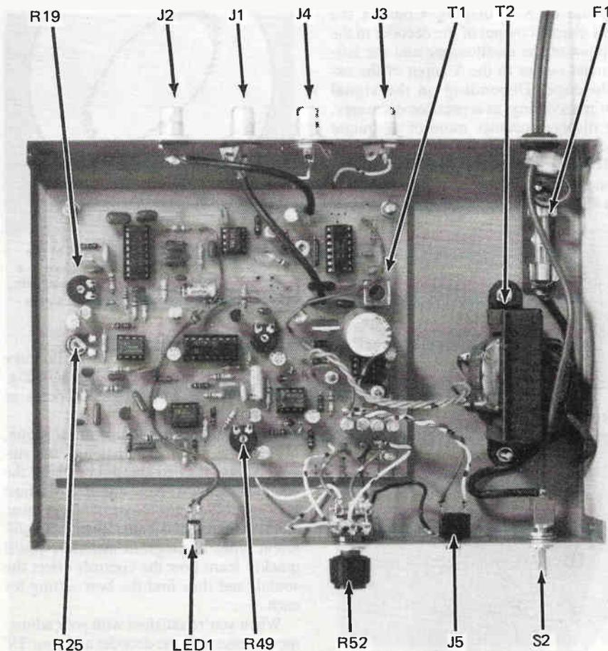
FIG. 9—THE COMPLETED DECODER appears as shown here. The board shown was an early prototype, so it doesn't match the parts-placement diagrams (shown in Fig. 7 and Fig. 8) exactly.
