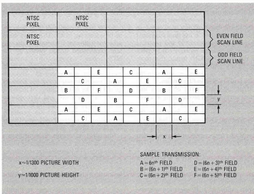
FIG. 4—IN THE DEL RAY HDTV SYSTEM, each NTSC pixel is broken up into six samples for transmission. Picture information is relayed in a sequence of six fields.
