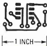
OUR ELECTRONIC SCARECROW can help chase away a less than determined burglar. If you chose to build that circuit on a PC board, here's a pattern that's appropriate.
