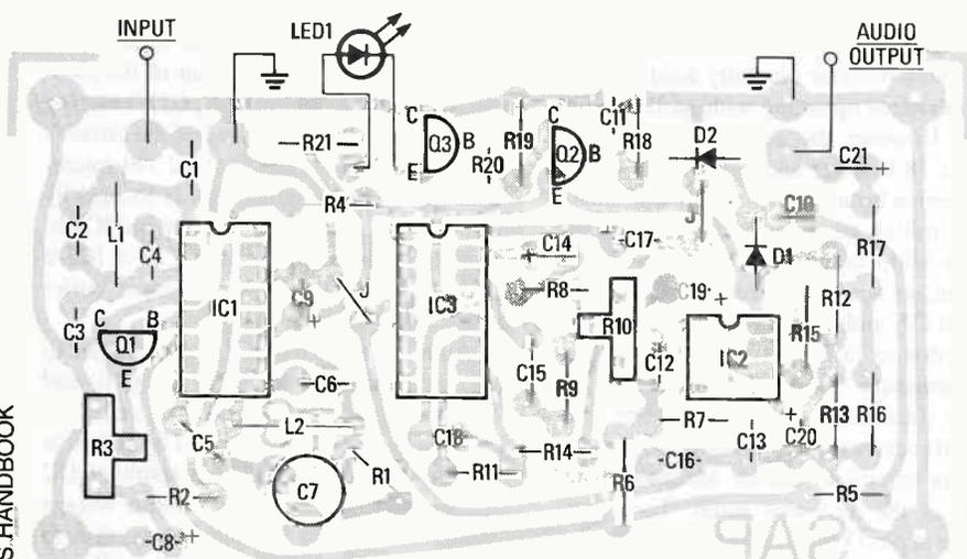
**FIG. 2—FOLLOW THIS DIAGRAM** for correct placement of the SAP board's components.
