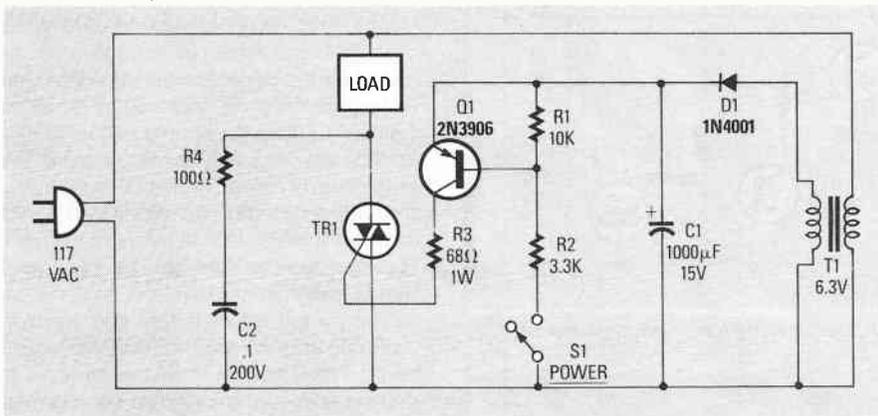
FIG 5—AC POWER SWITCH with transistor-aided DC triggering.
