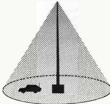
**FIG. 1—EARLY, NON-CELLULAR, MOBILE-telephone systems used a centrally located high-power transmitter. Only a few communications channels could be accommodated within a service region.**
