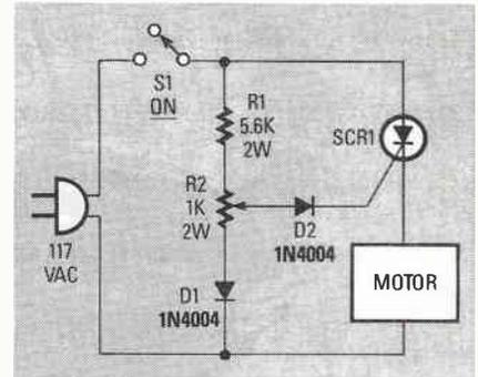
FIG 28—SELF-REGULATING UNIVERSAL-MOTOR heavy-duty speed controller.
