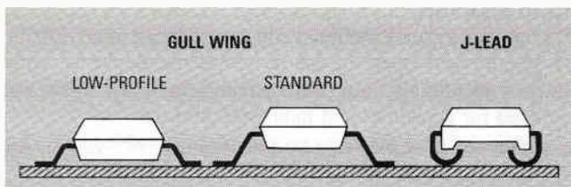
FIG. 12—GULL-WING VS. J-LEAD SMC packages. J-lead packages can be mounted using sockets
