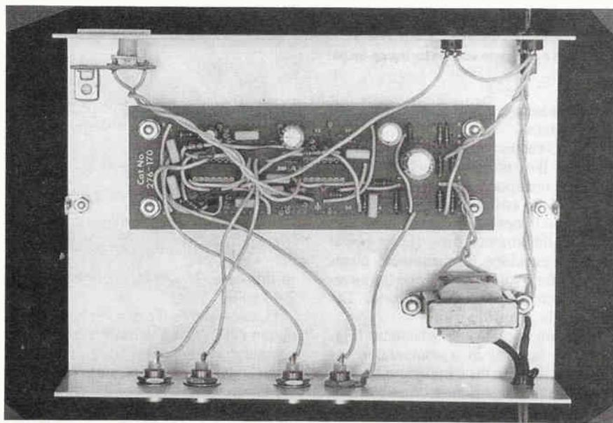
FIG. 6—THE AUTHOR'S PROTOTYPE was built on a piece of perfboard using point-to-point wiring. Keep your lead lengths short, and be careful with the 117-volt primary circuit.
