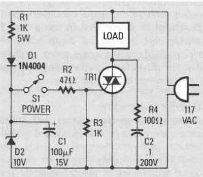
FIG 2—AC POWER SWITCH, DC triggered.
