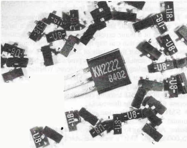
FIG. 9—A TO-92 TRANSISTOR dwarfs its SOT-23 counterparts.
