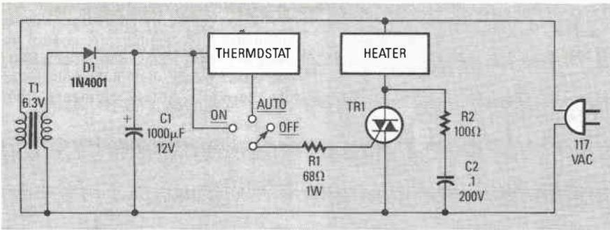
FIG 19—THERMOSTAT-SWITCHED heater controller.
