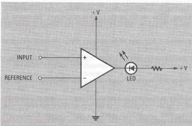
FIG. 2—IN AN INVERTING COMPARATOR, the output is low when the input voltage exceeds the reference voltage; the output is high when the input is lower than the reference voltage.
