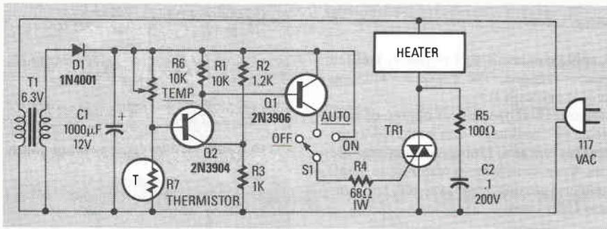
FIG 20—THERMISTOR-SWITCHED heater controller.
