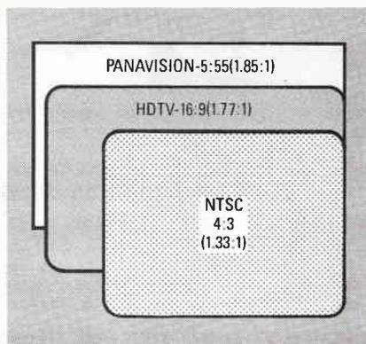
FIG. 2—ASPECT RATIOS. Here, the aspect ratios of conventional-TV, HDTV, and Panavision motion-picture viewing screens are compared.
