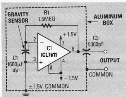
**FIG. 2—THE BASIC GRAVITY DETECTOR** is a current-to-voltage converter. The current through capacitor C1 is proportional to changes in the strength of the gravity field. IC1 amplifies the signal generated across capacitor C1 to drive a chart recorder or digital multimeter.
