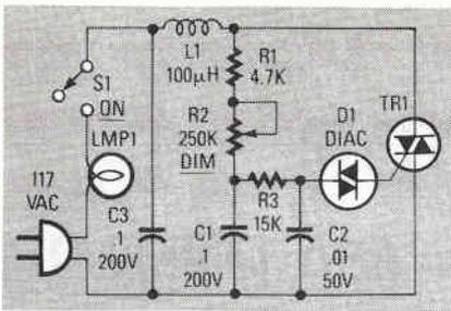
FIG 24—IMPROVED LAMP DIMMER with gate slaving.
