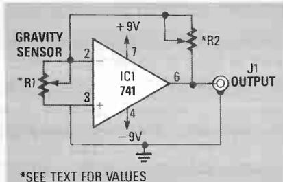
FIG. 6—A GRAVITY DETECTOR THAT USES a resistor sensor to detect gravity signals. Like the capacitor sensor, the resistor sensor is a  $1/f$  noise detector. Shield the detector unit from possible RFI interference.
