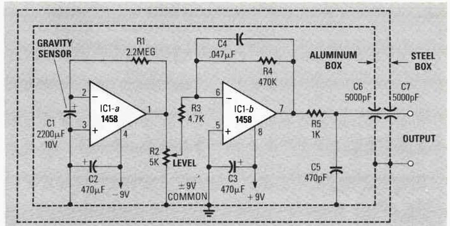
**FIG. 3—A BUFFERED GRAVITY DETECTOR** increases the detector's sensitivity to gravity fields, and also adds frequency stability to the detector. The aluminum box, the outer steel enclosure, and feedthrough filter capacitors C6 and C7, isolate the detector from electromagnetic interference (EMI).
