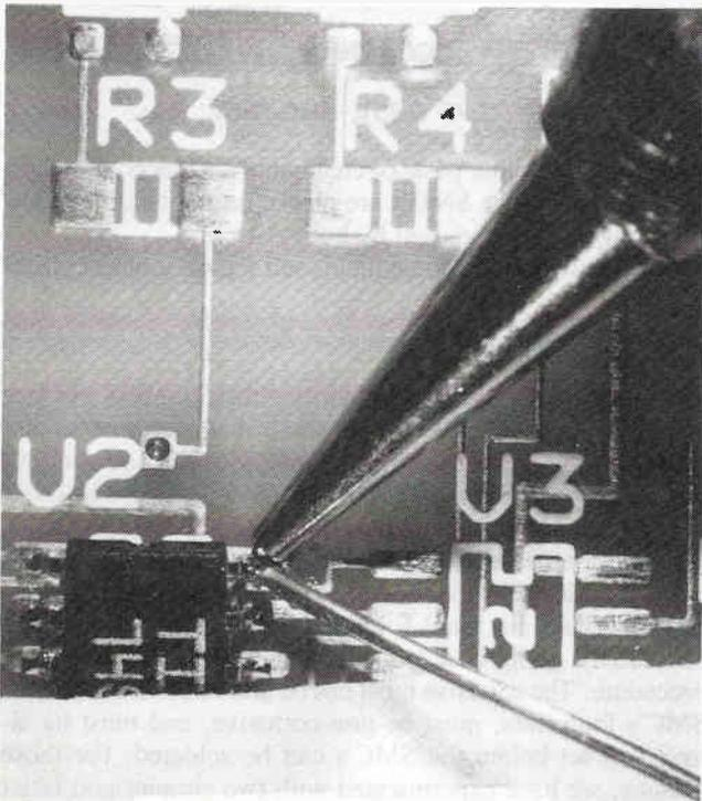
FIG. 2—ONE SIMPLE METHOD of securing an SMC in place is to tape down one side with masking tape.
