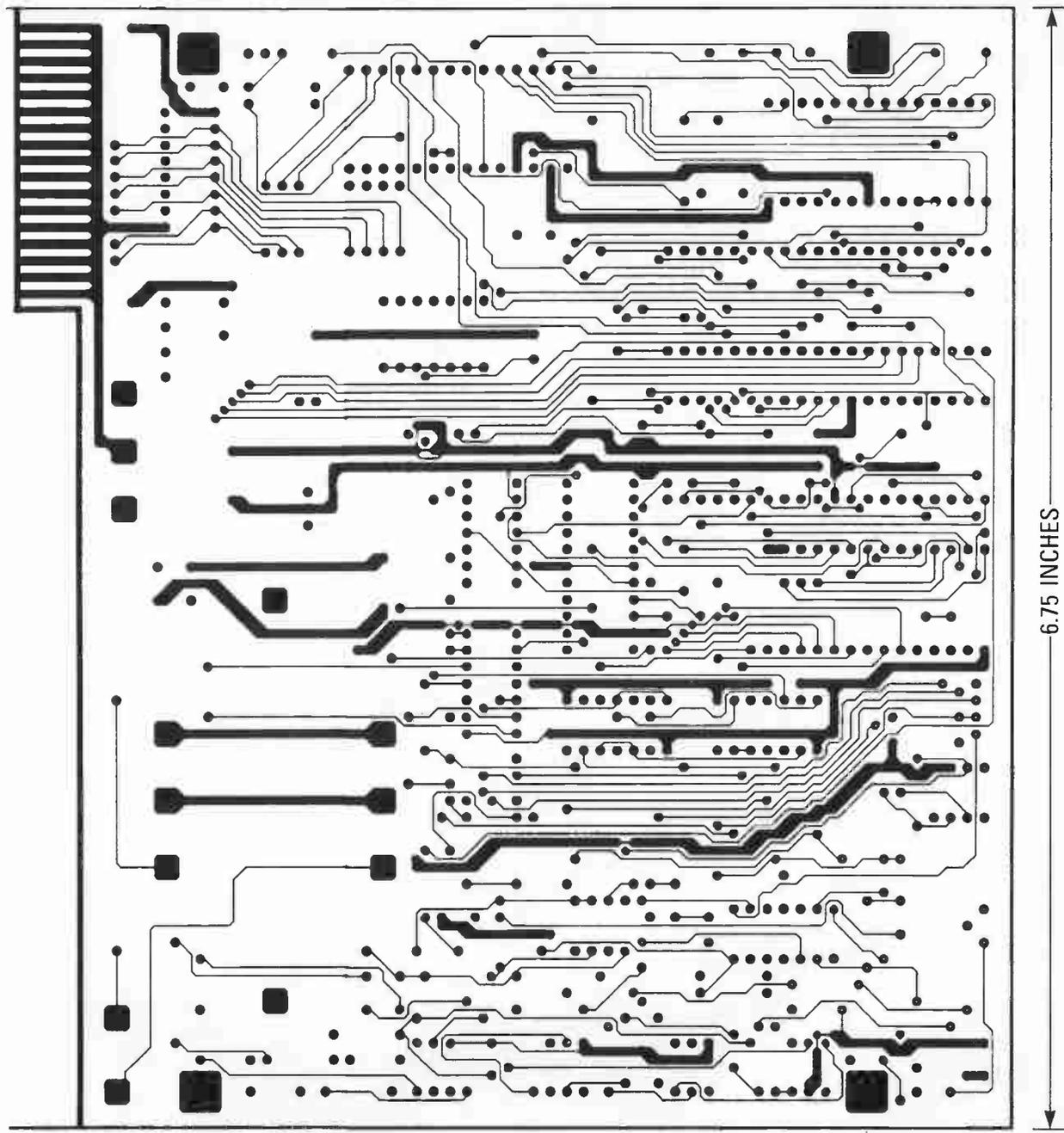
THE SOLDER SIDE of the Phonlink PC board is shown here.
