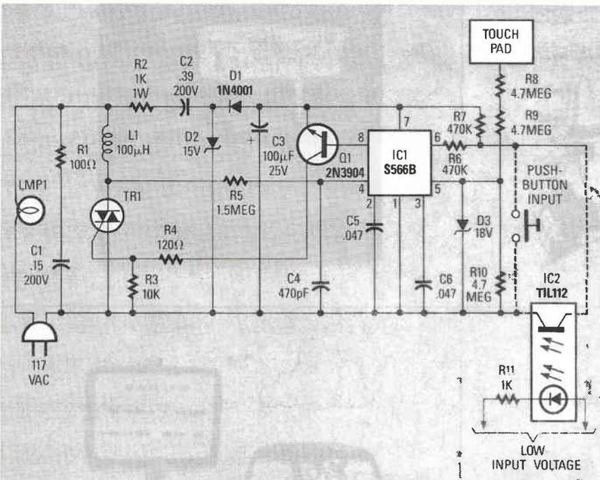
FIG 26—SMART LAMP DIMMER controlled by a Siemens S566B.
