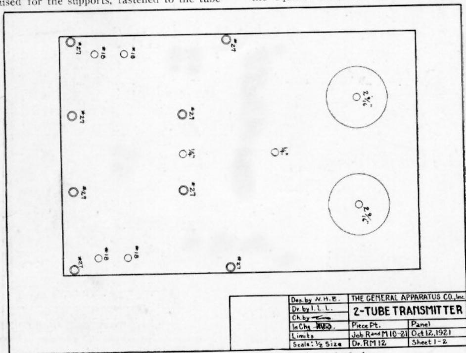
Fig. 3. The front panel reduced to one-quarter actual size.
