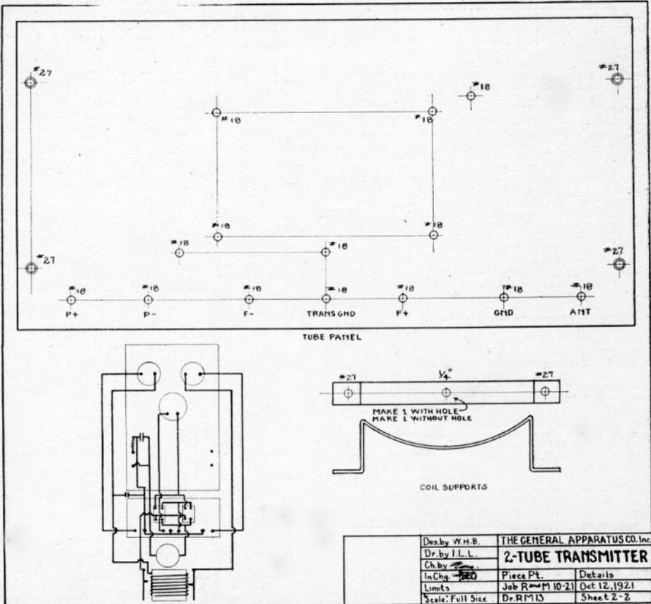
Fig. 2. Layout of the tube panel and coil supports, one-half size, with wiring diagram as it appears when looking at the rear of the set.
