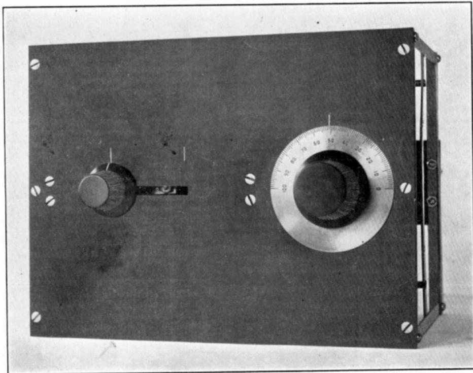
Fig. 1. Two controls only are used to tune from 12,000 to 20,000 meters, covering the range of trans-Atlantic stations.
