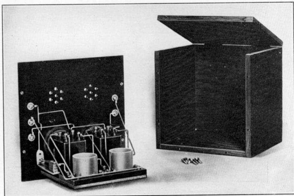
Fig. 6. The amplifier with the case removed
