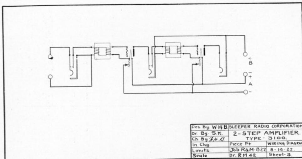
Fig. 5. Wiring diagram of the amplifier.
