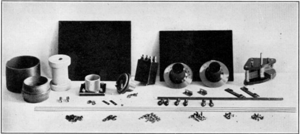
Fig. 5. Complete set of parts required for the construction of the oscillator
