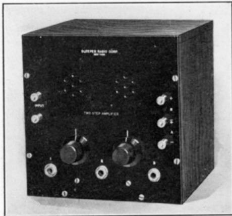
Fig. 2. Front view of the amplifier
