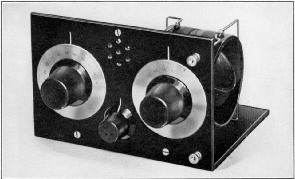
Fig. 1. Front view of the self modulated oscillator
