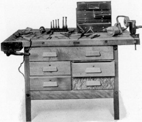
The tool chest is a particularly important adjunct to the shop equipment, for tools can be kept in good condition only by putting them away neatly in a place where they will be secure from dampness. This chest is built of mahogany, and has eight felt-lined drawers. A small bench grinder solves the problem of keeping drills, cutters, and edge tools properly sharpened.
