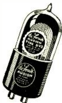
This tube, the DV-3, consumes a filament current of only 6/100 of an ampere. It operates at a filament potential of 3 volts.
