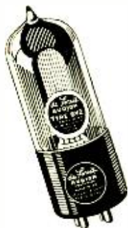
The DV-2 has a filament potential of 4½ volts and a filament consumption of 25/100 of an ampere.
