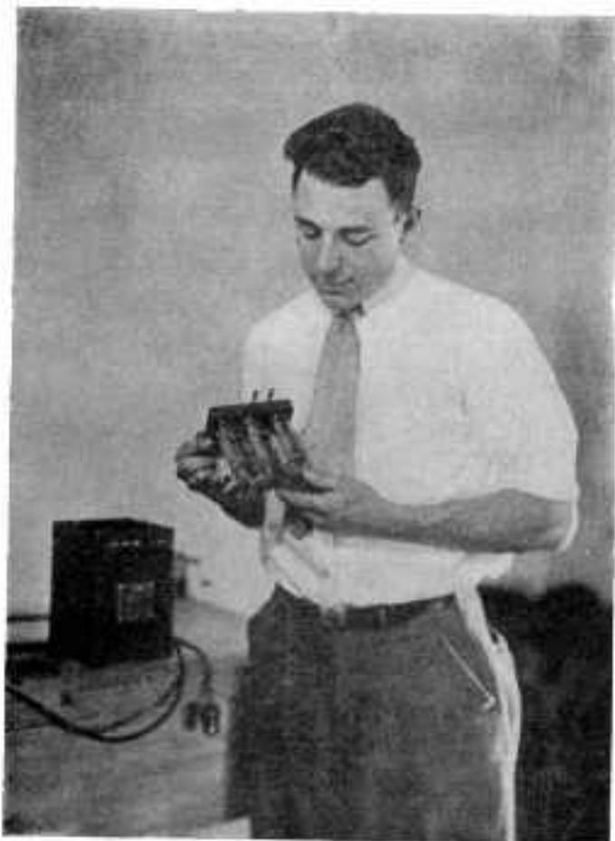
Fig. 1. The chemical cells used in the Balkite unit.
