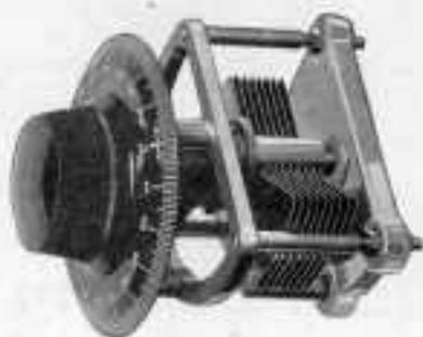
Furnished in straight line frequency and straight line wavelength design. The straight line frequency condensers spread all stations evenly around the dial according to frequency. The plates are so fashioned that no excess panel space is required.
