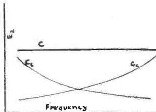
ing the constants of the circuit we can have maximum regeneration over a range of 150 to 600 meters, or increasing regeneration on the high wavelengths. In other words, we have a new regenerative control which can be set once and then will be fixed for all frequencies.
