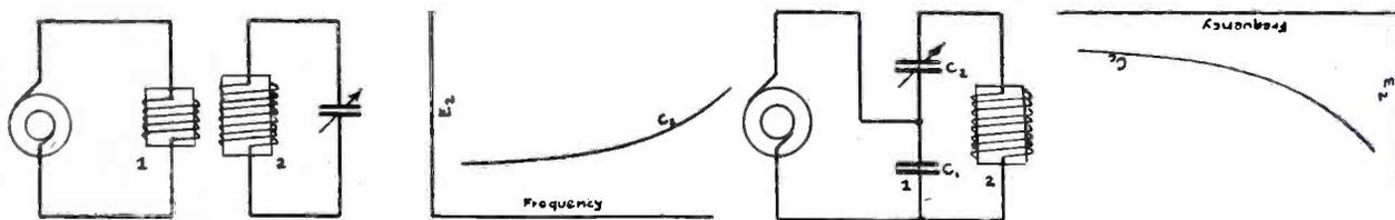
Figs. 1 and 2. Illustrating the effect of frequency upon magnetic coupling. Figs. 3 and 4. The action which takes place with electrostatic coupling between circuits
