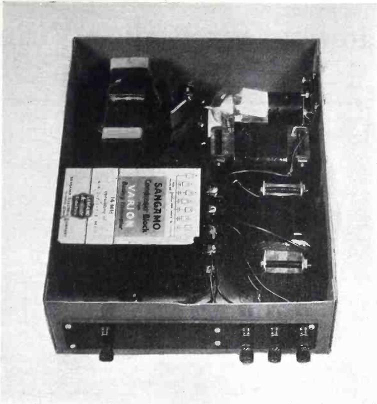
Fig. 1. The eliminator unit, made up of standard parts built into a new Raytheon circuit
