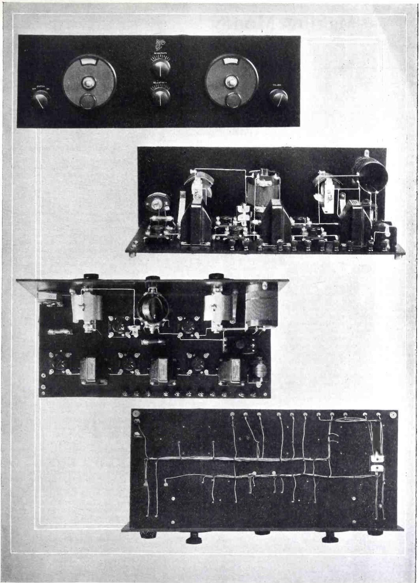
Fig 2. Four views of the assembled Dual TC, a development of the TC circuit so popular last year
