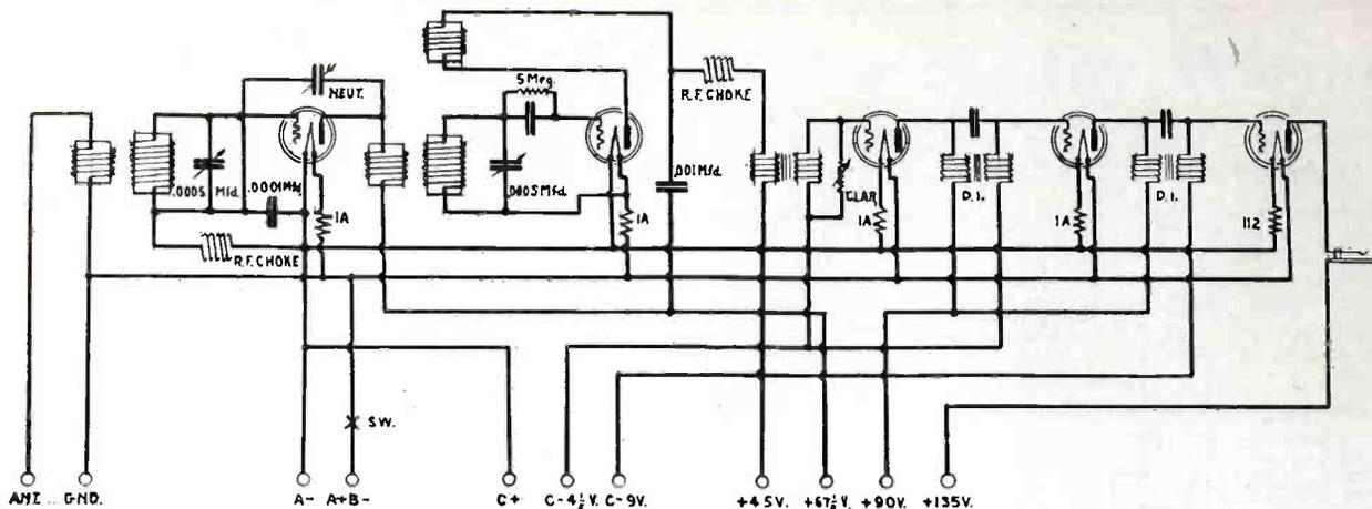
Schematic diagram of the Dual TC receiver, including the latest refinements of design as indicated in the photographs on the page opposite
