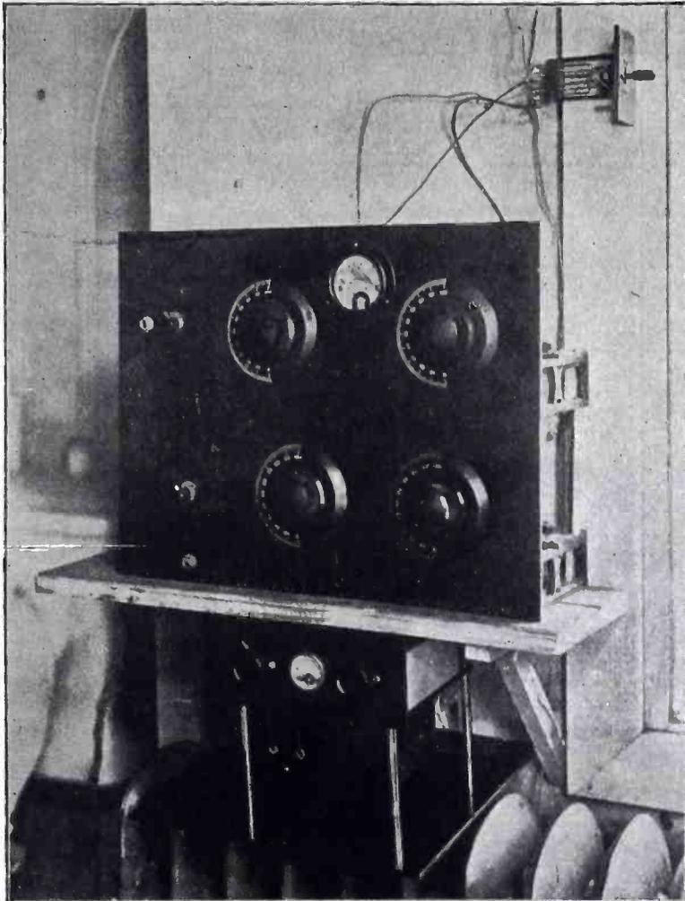
Fig. 3. The S. W. receiver and transmitter, with the power supply unit beneath
