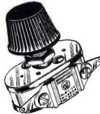
Provides a noiseless range of grid leak resistance from  $\frac{1}{4}$  to 10 megohms. Assures most effective grid leak resistance value for all tubes. Small grid condenser (0.00025) is separate. Metal parts nickel plated. One hole mounting.
