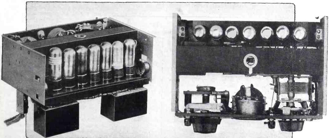
Fig. 2. Rear and top views of the 1927 Operadio. Note the catacombs, below the tubes, which contain the radio and audio amplifying circuits. The top view shows some of the mechanical developments
