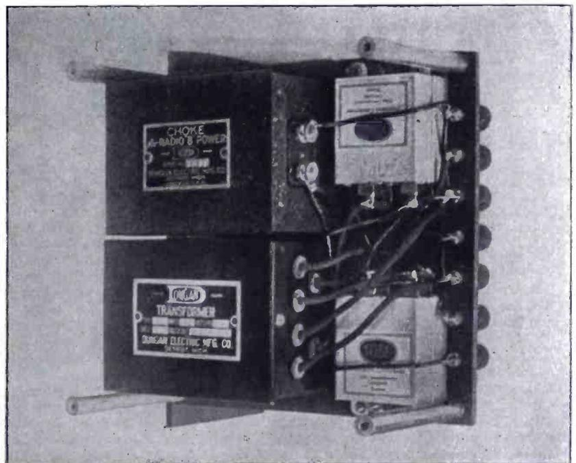
Fig. 4. Bottom view, showing the transformer, choke, and a part of the filter
