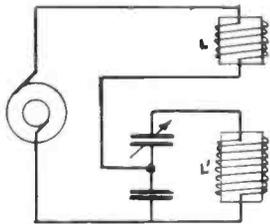
Figs. 5 and 6. Loftin and White combine magnetic and electrostatic coupling to produce constant coupling at all frequencies
