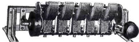
Perlesz gang-mounted condensers are operated by a self-adjusting worm drive giving a 340 degree movement to the speedometer type dial. Back lash is eliminated.
