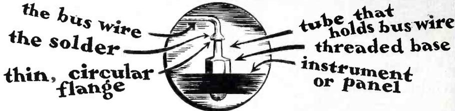
The Standard, tubular Soldering Terminal
