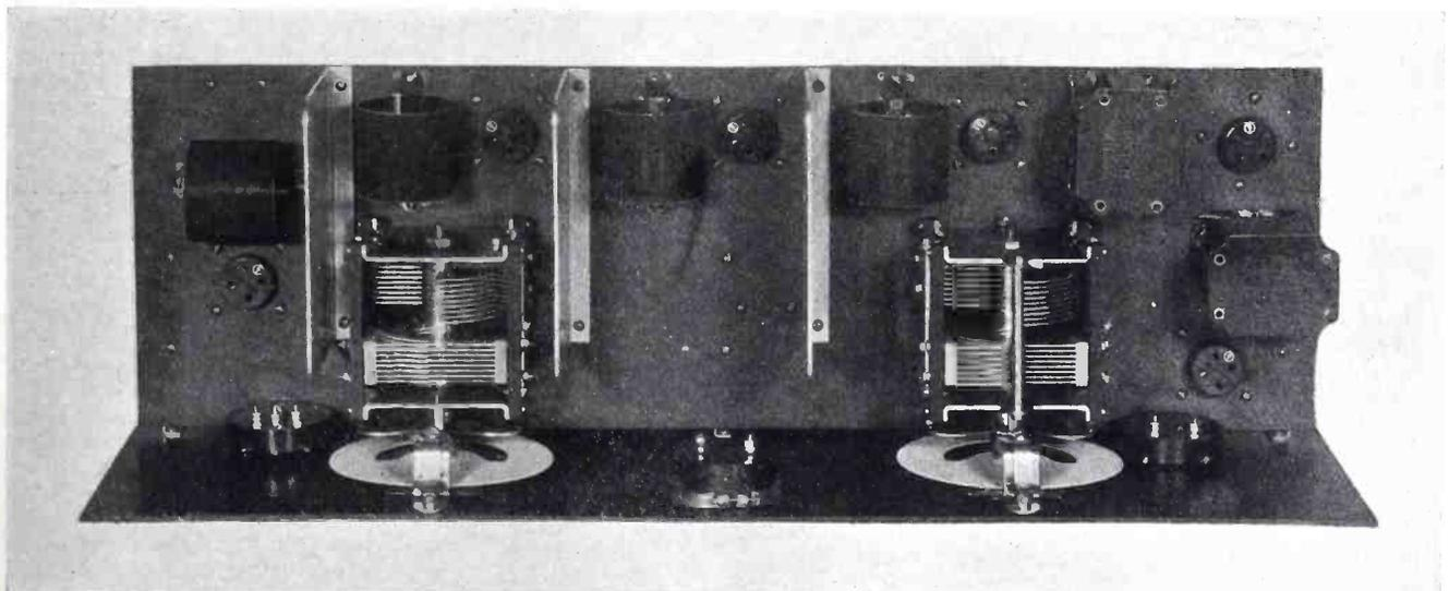
Fig. 2. Five 199 tubes and a 171 are used in this Varion set. The very finest parts have been chosen, and the circuit has been worked out with unusual thoroughness
