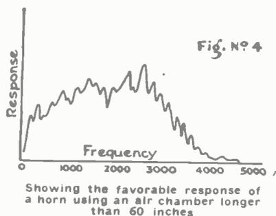
Showing the favorable response of a horn using an air chamber longer than 60 inches
