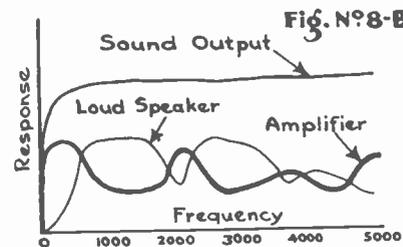
Desirable characteristics of an amplifier to work in conjunction with a cone loudspeaker
