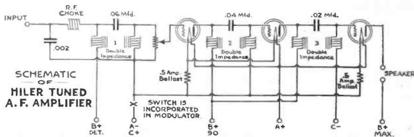
The general circuit of the tuned double impedance amplifier. Variations of this circuit are covered in the article
