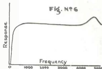
Curve of an improved audio frequency transformer. Low frequency response is lacking and the unit peaks at a high frequency
