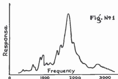
The effect of a combination of the early transformers and horn type speakers
