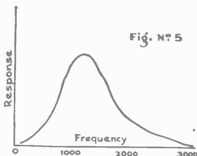
Curve of an early audio transformer, designed for code work in radio telegraph
