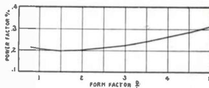
Fig. 3. Showing the desirability of keeping the form factor about 1 to 2.5
