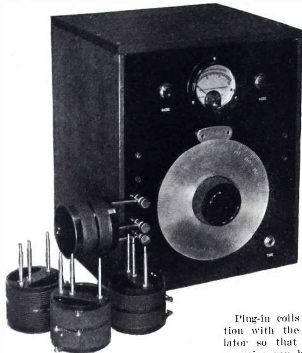
Left: A view of the completed Modulated Oscillator and a group of plug-in coils for covering various frequency ranges. The frequency of the R.F. oscillator is controlled by the dial. Below: The schematic diagram of the test oscillator. Note that the negative filament leg is grounded.
