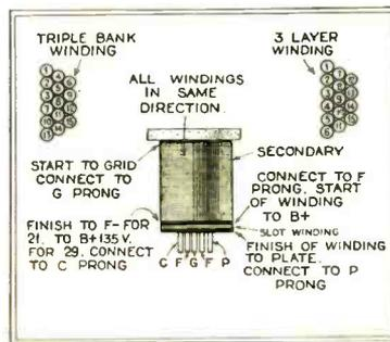
Winding details of the long wave coils.
