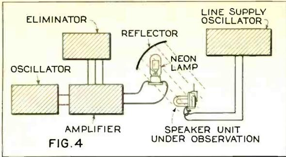
General layout of the apparatus constituting the neon stroboscope, and the line supply oscillator connection.
