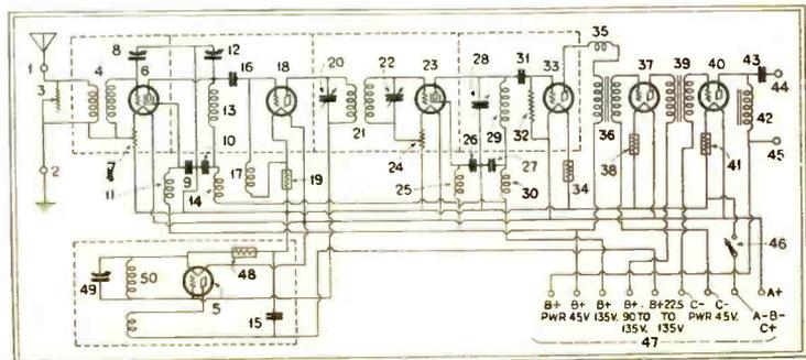
Schematic diagram of "Ultra Shield Grid Seven."
