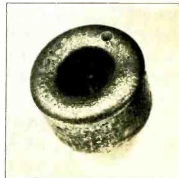
Chilled cast iron die for drawing No. 3 to No. 14 gauge wires.
