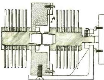
Fig. 8. Cross section of the spark gap invented by Prof. E. L. Chaffee.
