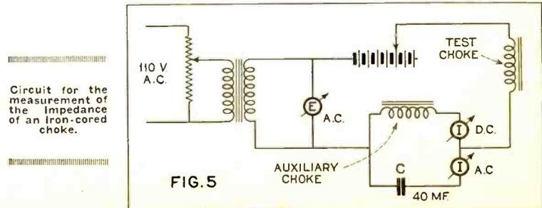
Circuit for the measurement of the impedance of an iron-cored choke.
