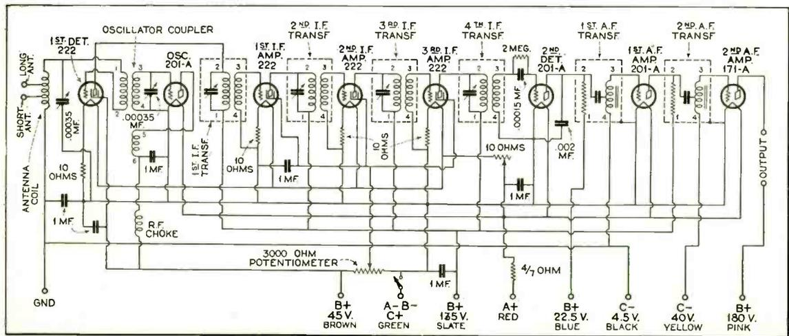
The schematic diagram of the Lincoln 8-80 One Spot Super. Note that a screen-grid tube is used as the first detector. The same type of tube is used in the I.F. amplifier. The Clough system of audio frequency amplification is employed.
