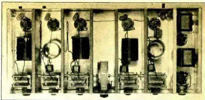
Fig. 2. Interior view of the Sargent-Raymont Receiver. Note position of R.F. coils and the elaborate shielding.
