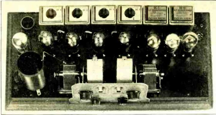
Inside view of the Lincoln 8-80. The I.F. and A.F. transformers are mounted in a straight line along the rear of the sub-base.
