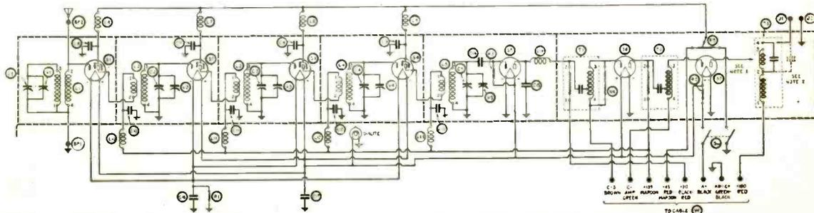
Fig. 4. Schematic diagram of the Sargent-Rayment Receiver. Screen-grid tubes are used in the R.F. stages.
