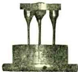
Fig. 9. The Branly Tripod Detector.
