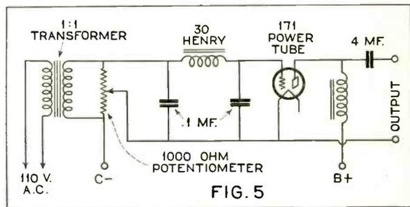
Circuit diagram of the line supply oscillator which is used in connection with the speaker unit under observation.
