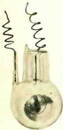
Fig. 2. This is the type of photoelectric cell which is employed for the reproduction of music from sound films.
