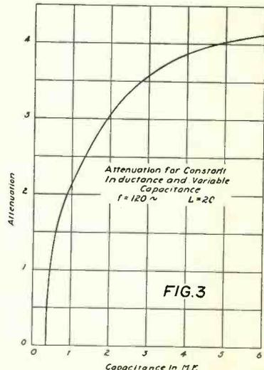
Curve of attenuation plotted against capacitance.
