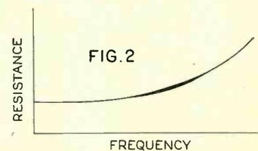
Curve showing the relative change of resistance with a change in frequency.
