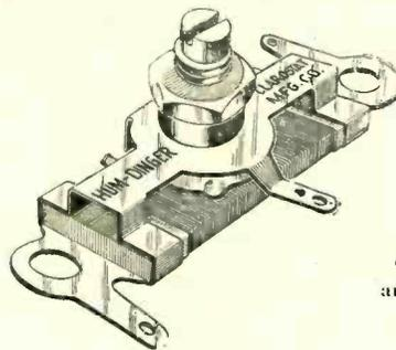
THE slotted head is recessed in the bushing mounted in panel or sub-panel, ready for instant adjustment by service man or expert, but out of the way of meddling fingers. Available in any resistance range from 6 to 200 ohms. Cheaper than usual potentiometer; cheaper than center-tapped transformer winding. Carrying capacity—more than ample for any A-C tube circuit.
