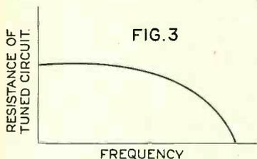
Another typical case of the "bends," where the resistance of a tuned circuit changes with a change in frequency.
