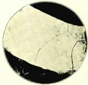
Fig. 2. The piece of tungsten here shown was burned in an oxidizing atmosphere and shows oxide contamination along the grain boundaries. Mag. 50.
