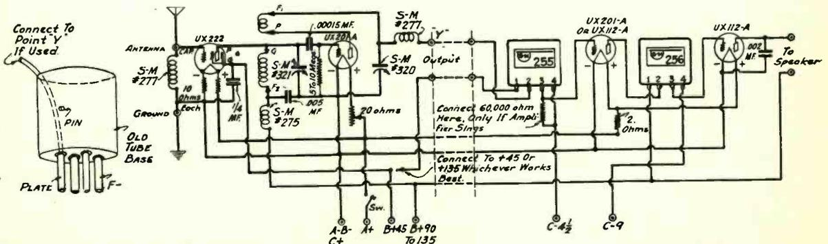
Complete schematic diagram of the "Round the World Four" and, at the left, details of the adapter.
