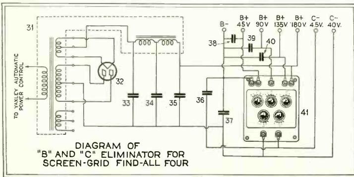
The B and C power unit, which employs a 80-type full-wave rectifier. Note the compact, variable voltage divider.
