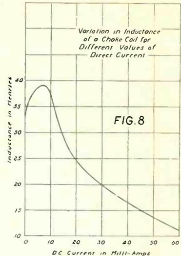
Curve showing the variation in inductance of a common type of filter choke.
