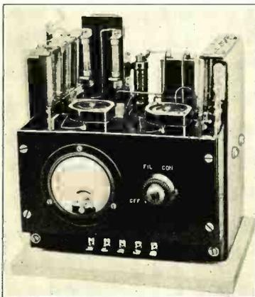
Fig. 4. The amplifier to which the photoelectric cell is connected, showing the suspension for absorbing vibrations. The tubes are not in place.
