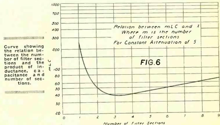
Curve showing the relation between the number of filter sections and the product of inductance, capacitance and number of sections.
