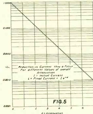
Ratio of A.C. amplitude in the output and input sides of the filter.
