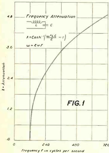
Curve showing attenuation of a filter at various frequencies.
