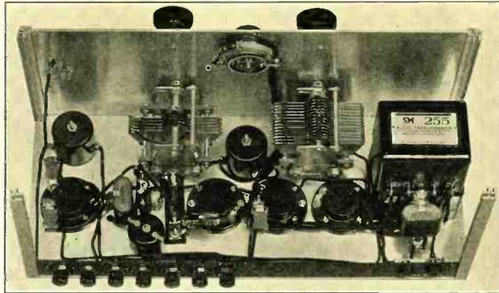
Interior view of the "Round the World Four". Note the neat layout of the parts. Regeneration is controlled by the large variable condenser.
