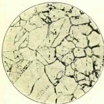
Fig. 1. A microphotograph of nickel that has been burned in a sulphurous atmosphere and which shows sulphur contamination along grain boundaries. Mag. 200.
