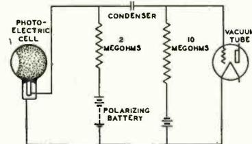
Fig. 3. The circuit employed between the photoelectric cell and the adjacent amplifier.
