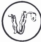
This is a close-up view of the new Eby double contact prong. Spring tension evenly divided between top and bottom of both sides.
