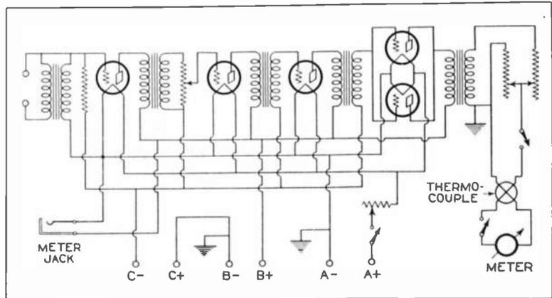
Schematic diagram of the Acoustimeter. The pick-up is not shown connected in the circuit.
