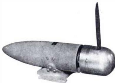
The wind-driven generator, which supplies all the necessary current for operating the transmitter and receiver.
