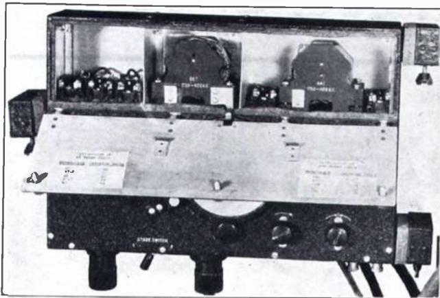
The five-tube receiver has wave-length ranges of 50 to 150 meters and 580 to 1100 meters. Notice the special suspension mounting clamps, which facilitate mounting. The weight is approximately 11 pounds.
