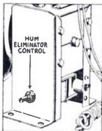
The variable hum control is conveniently mounted on the speaker chassis and can be adjusted by the user.
