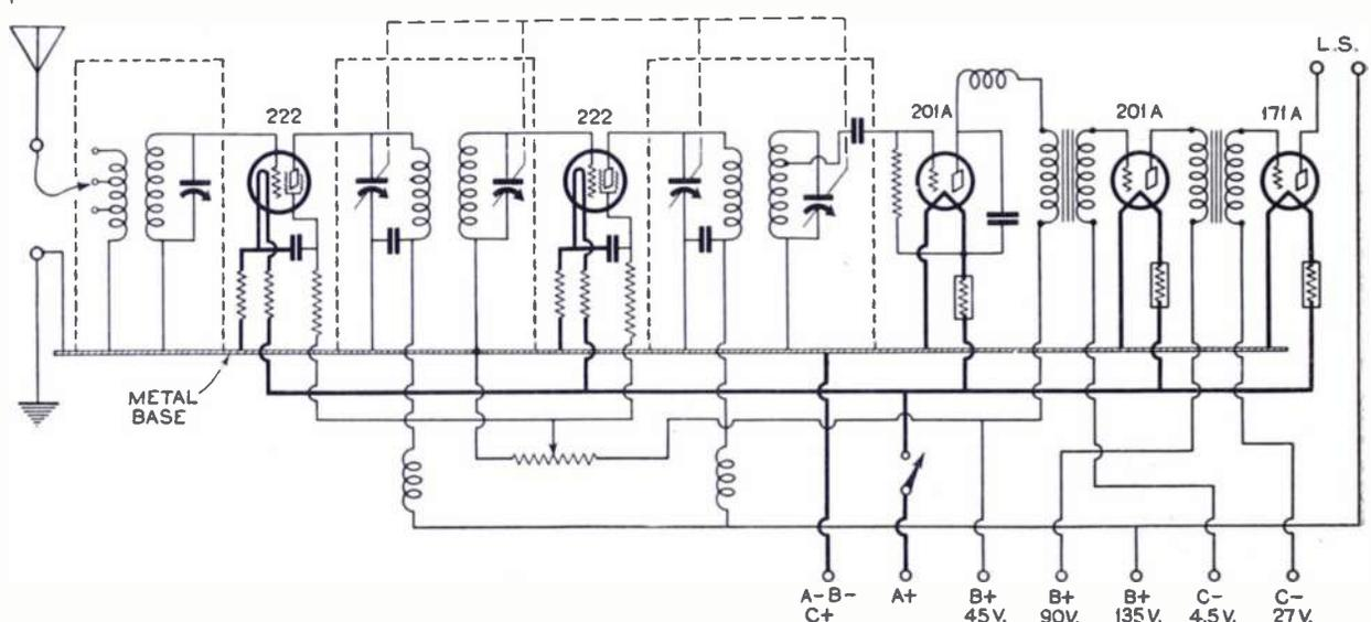
A typical band selector circuit, with tuned plate and grid circuits, which provides a rectangular resonance curve.
