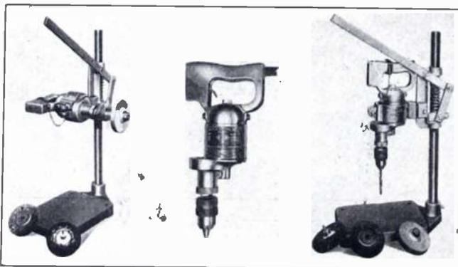
The Wodack portable electric drill and the special stand which allows the drill to be operated in a vertical or a horizontal position.
