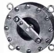
The new Electric - Acoustic Products Co. two - button microphone.
