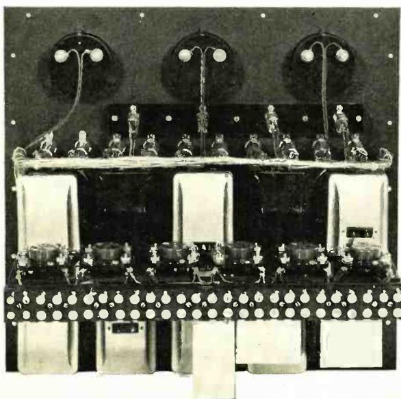
Fig. 2. Rear panel view of the pick-up amplifier, showing the resistor bank, the tube sockets, the connector strip and the special transformers and impedances. Note the bunched leads.
