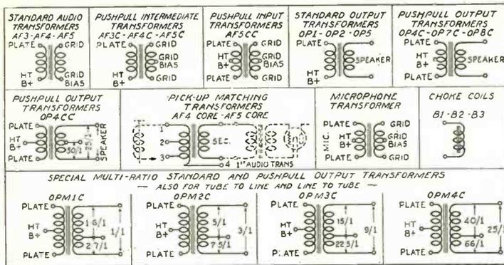
Fig. 3. Showing, in schematic form, a group of transformers well suited to meet the special requirements of audio-frequency transmission lines, etc. (Courtesy of Ferranti, Inc.)
