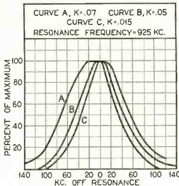
A family of resonance curves, taken at 925 KC., for various values of circuit coupling.
