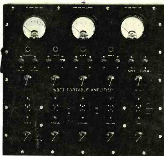
when more than one microphone is being used simultaneously or if one microphone is being used for the program pick-up and another for the announcing the volume controls can be so set that the volume level of the program and the announcer is whatever is required for proper operation and when switching from one to the other of the microphones, the over-all gain of the amplifier would not have to be adjusted each time the change is made.
