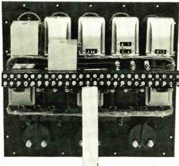
Fig. 3. Another rear view of the pick-up amplifier, which brings partially to view the microphone volume controls and the gain control. Directly in front of these controls are the Mike-to-Tube and Mike-to-Line transformers.
