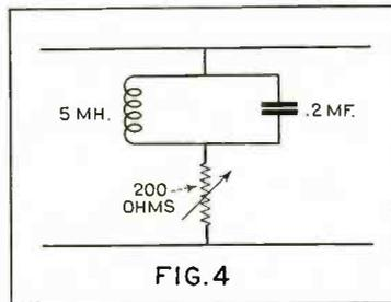
Equalizer circuit to neutralize peak at 1000 cycles
