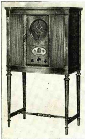
The "Silver" model 95 screen-grid receiver with 245 push-pull output and dynamic speaker.
