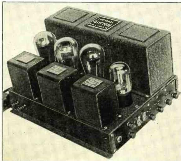
The new National Velvetone Amplifier. A 227 is employed in the first stage and two 245 tubes, in push-pull, in the output stage. B and C voltages are supplied by a 280 rectifier tube.
