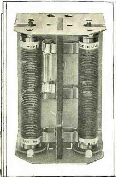
The rectifier units can be easily replaced when necessary as may be seen here.
