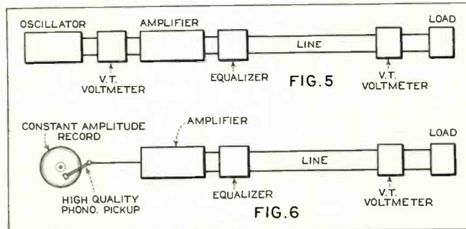
Fig. 5. Set-up, with beat frequency oscillator, for making frequency runs on transmission lines.
