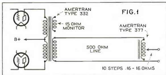
undistorted power output is obtainable when the tube works into a load impedance of twice its  $R_p$ . Hence
