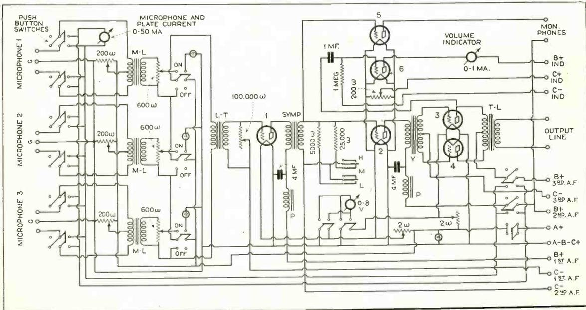
Complete schematic diagram of the mixer and line amplifier, described in the accompanying article.
