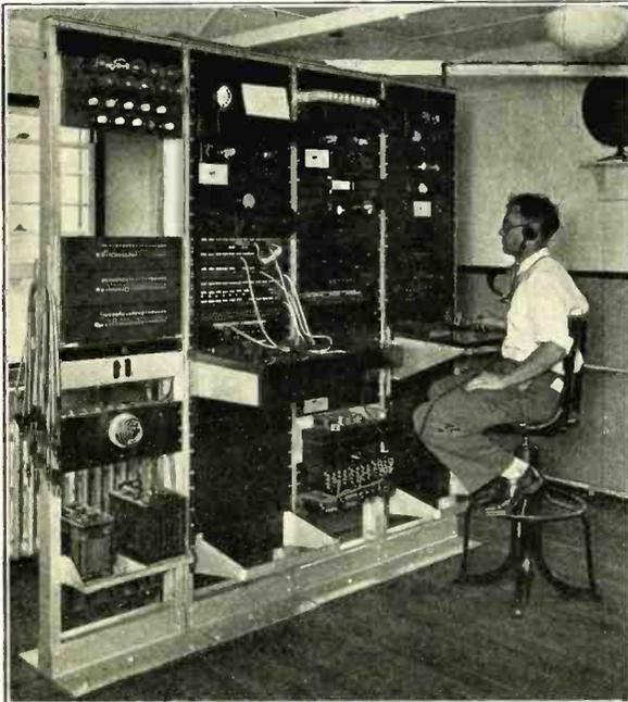
Line terminal equipment at Netcong, used by the Bell Telephone Laboratories for short-wave radio telephony between the United States and Great Britain.
