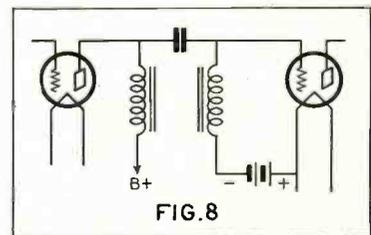
A double impedance coupled amplifier circuit, which may or may not be of the "tuned" type.
