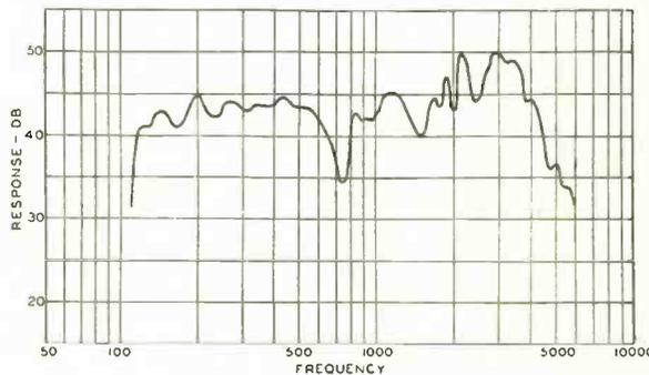
Fig. 5. Response-frequency characteristic of 3/2-inch piston-diaphragm loudspeaker. Measured 12 feet from diaphragm, in highly absorbing room.
