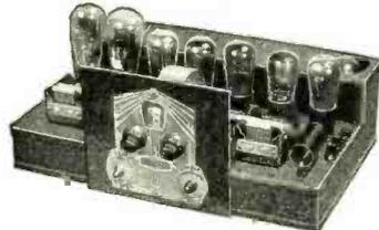
Chassis of Pierce-Airo receiver, designed for use with either an a-c. or d-c. dynamic speaker.
