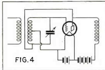
The introduction of regeneration has considerable bearing on the shape and amplitude of the resonance curve.
