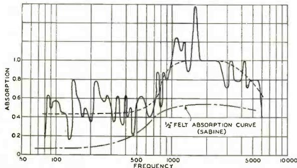
Fig. 8. Absorption - frequency characteristic of felt-lined room with respect to a region relatively near its center and the sound source. Calculated from data of Fig. 7.
