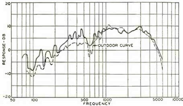
Fig. 7. Response - frequency characteristic of 3½-inch piston-diaphragm loud-speaker. Measured in highly absorbing room and averaged in small region 12 feet from diaphragm.
